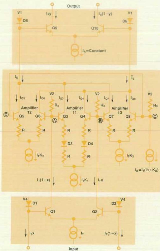
Fig. 11. The Booster IC's triangle-to-sine converter uses a new technique that offers advantages over conventional methods. See text for details.
