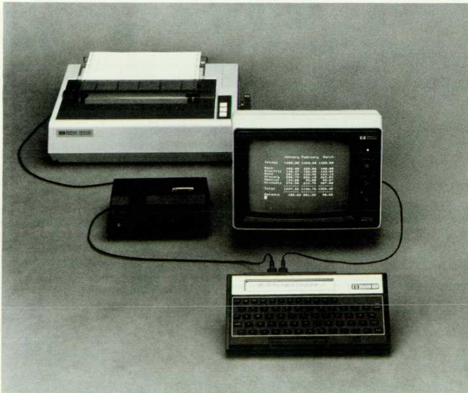
**Fig. 1.** This HP-75 system features HP's 82161A Digital Cassette Drive, 82163A Video Interface (plus a video monitor) and 82905B Printer.
