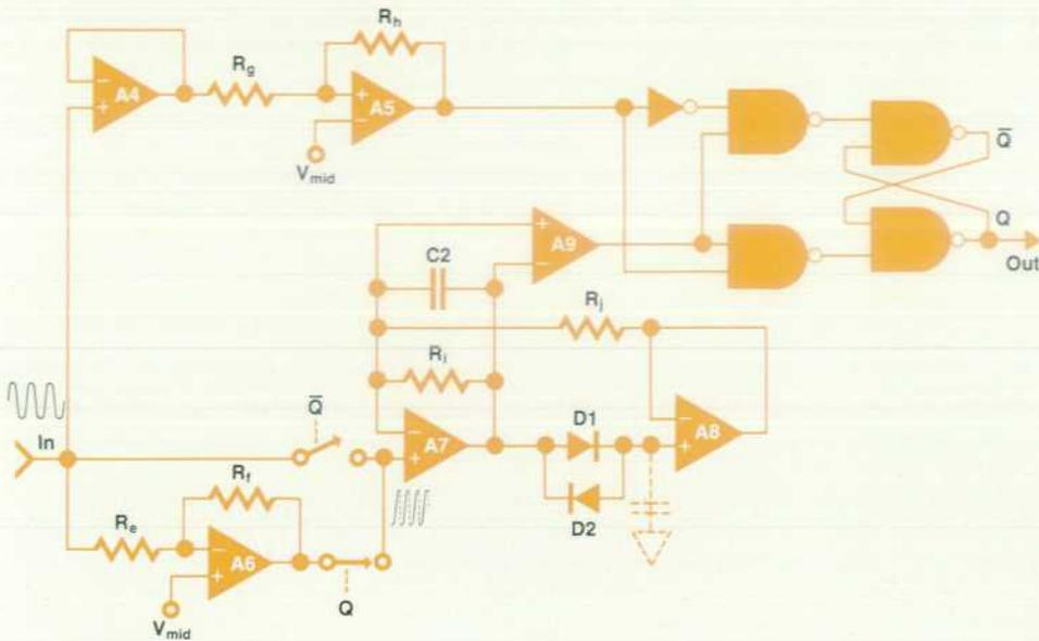
**Fig. 11.** Detector circuits. Timing track detection uses only the threshold-detect circuit formed by A4 and A5. Data track detection uses both threshold-detect and peak-detect (A6, A7, A8, and A9) circuits.
