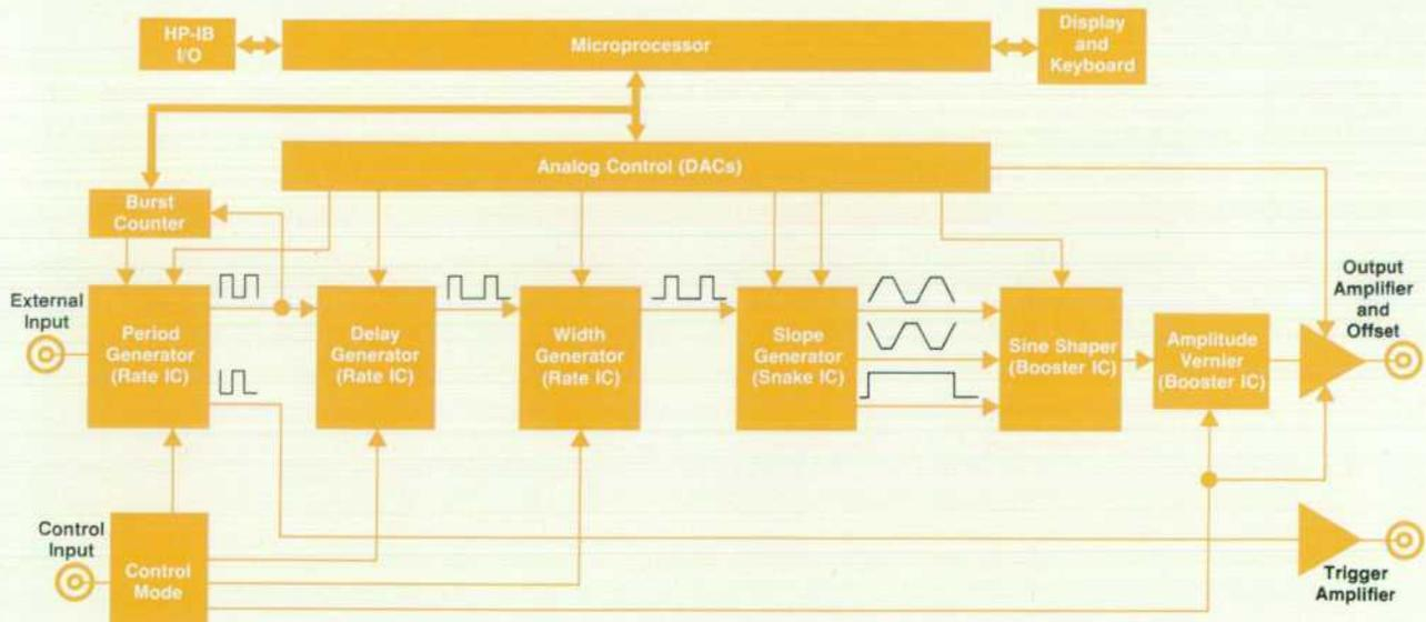
Fig. 7. Block diagram of the 8112A Pulse Generator. Three custom integrated circuits (Rate, Snake, and Booster) are used in all three instruments in the family. The output amplifier is also common to all three instruments.
