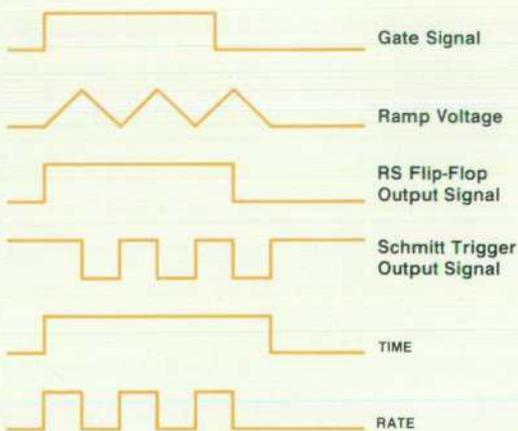
Fig. 5. Timing diagram for Fig. 3 in gate mode.
