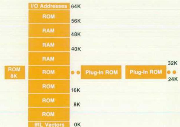
Fig. 3. Memory organization in the HP-75 Portable Computer.
