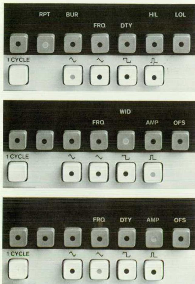
Fig. 5. The 8116A prompts the user by backlighting only the parameter mnemonics appropriate to the selected mode and waveform.
