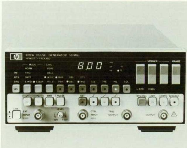
**Fig. 3.** Model 8112A Pulse Generator has all of the traditional pulse features for testing digital circuits, along with modulation capabilities useful for analog testing. It is HP-IB programmable and has a maximum repetition rate of 50 MHz.
