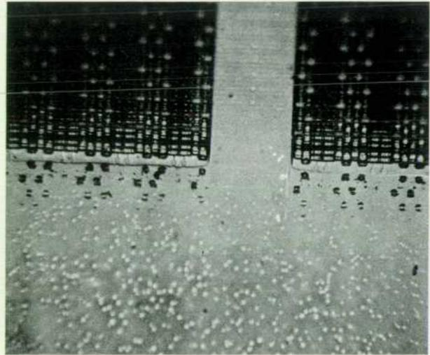
Fig. 2. Microphotograph of angle-lapped and Wright-etched cross section of an early 128K-bit RAM wafer showing heavy concentration of oxygen precipitates that contributed to excess junction leakage.
