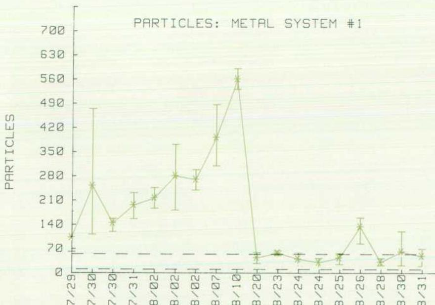
Fig. 1. Control chart showing the reduction in particle count over a period of time as a metal deposition process was improved.
