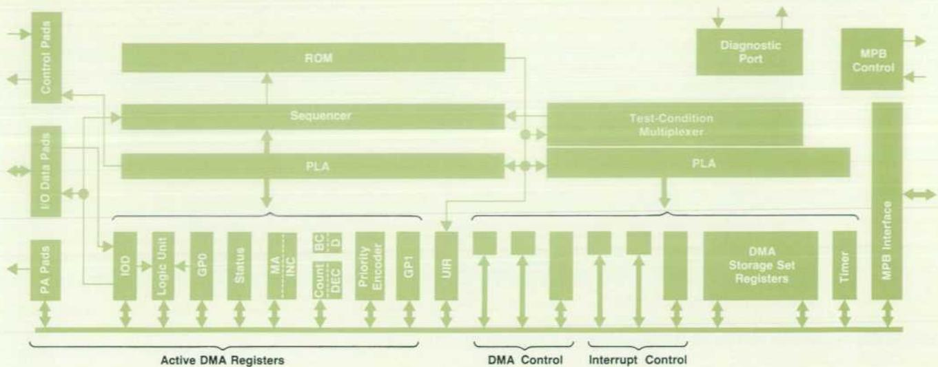
Fig. 2. Block diagram of the I/O processor chip.
