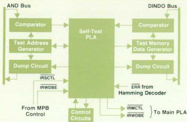
Fig. 7. Block diagram of self-test system incorporated onto the memory controller chip.
