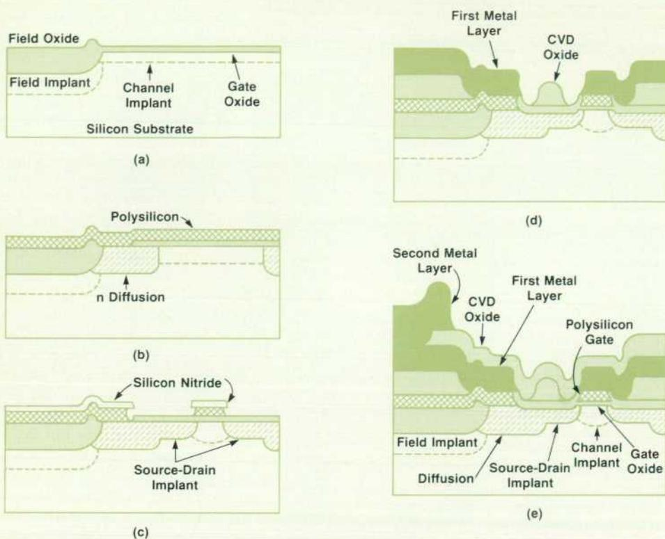
**Fig. 3.** Cross sections of the device structure during various steps of the NMOS-III process. (a) After gate oxidation. (b) After polysilicon deposition and doping. (c) After polysilicon patterning and source-drain implantation. (d) After first-layer metal patterning. (e) Completed device structure.
