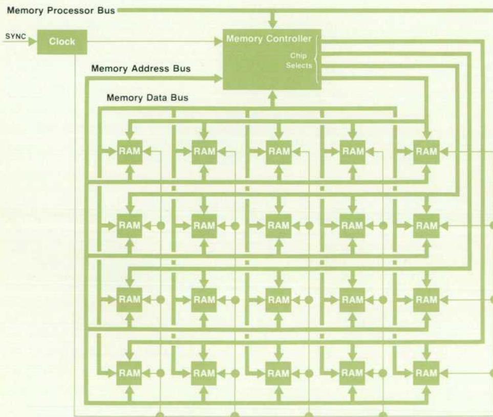
Fig. 1. Block diagram of high-performance VLSI memory system.
