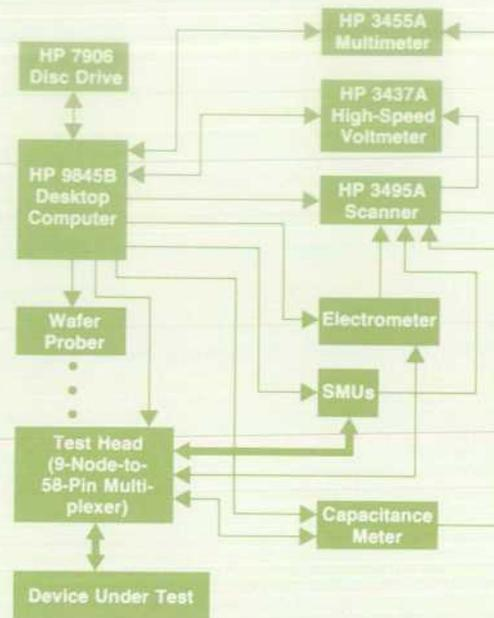
**Fig. 1.** Block diagram of the automated wafer parameter test system used for the NMOS-III process.
