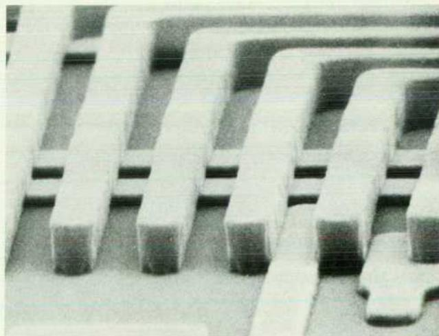
Fig. 4. Microphotograph of exposed and developed PMMA pattern.
