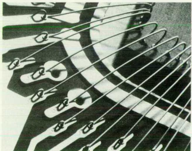
**Fig. 2.** Wire bonds from the IC to the finstrate use an extra ball bond over the tail bond as shown.
