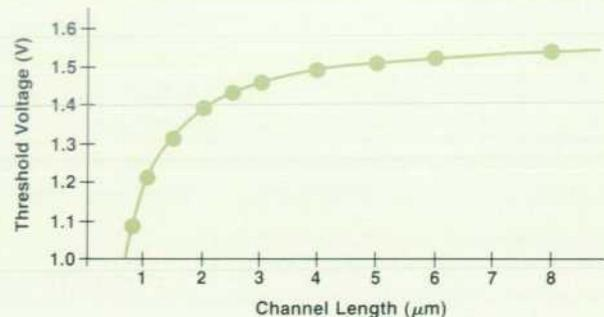
Fig. 1. Effect of channel length on threshold voltage.
