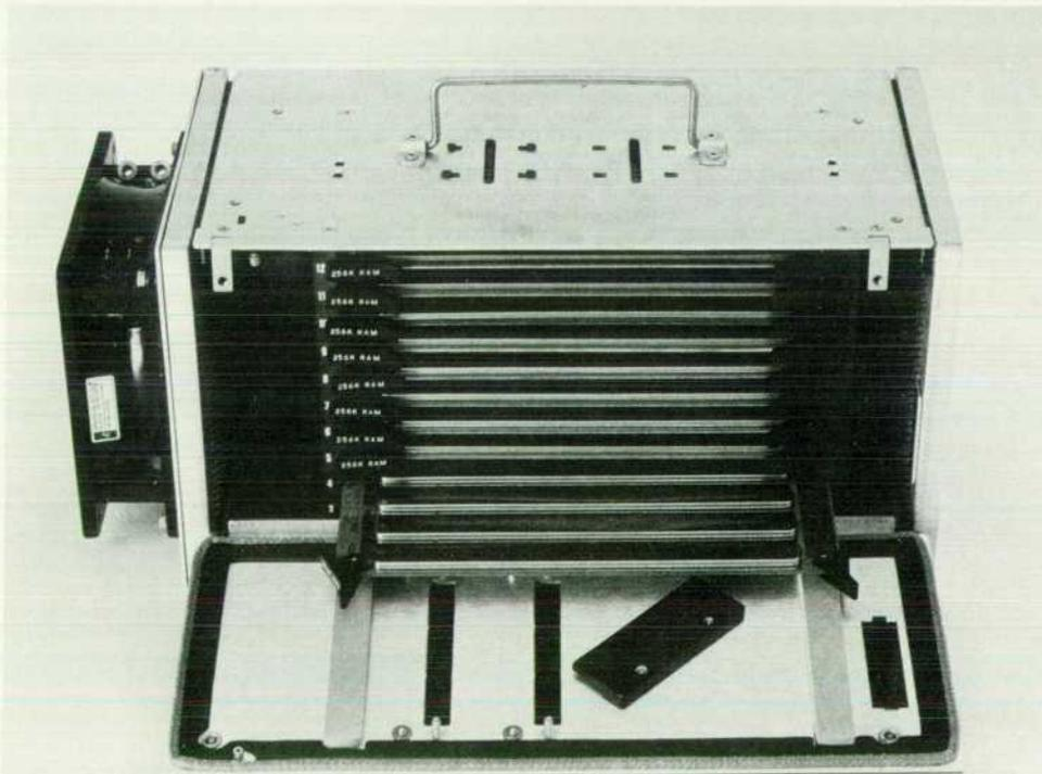
Fig. 4. This package, called the Memory/Processor Module, can contain a complete 32-bit computer system with 2.5 megabytes of RAM. Performance can be enhanced by exchanging some of the memory boards for additional CPU and/or I/O processor boards.
