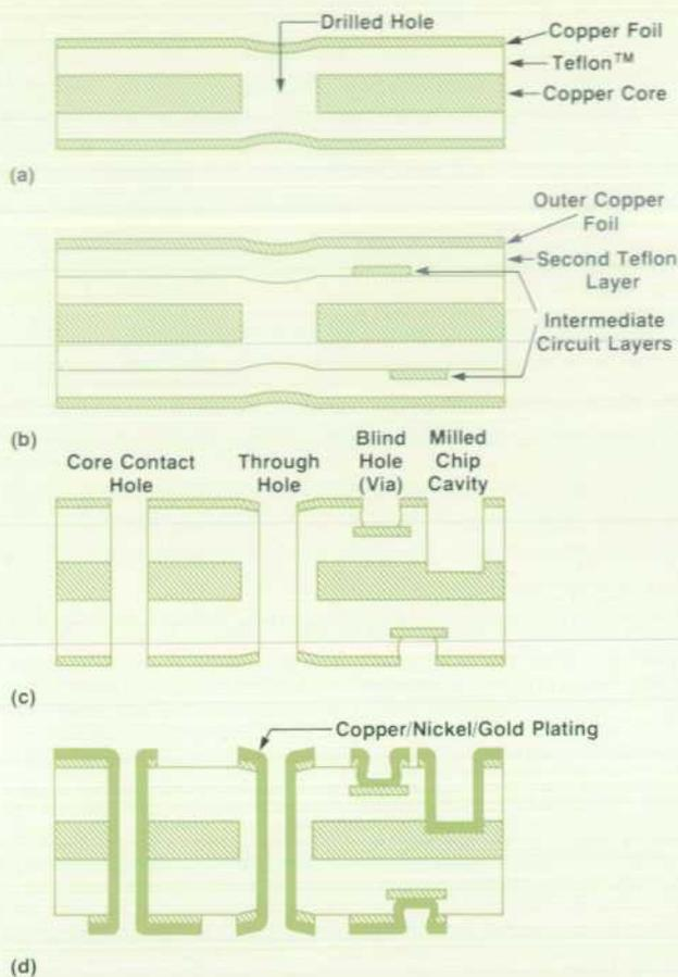
**Fig. 1.** Cross sections during the finstrate fabrication sequence. (a) After lamination of the intermediate copper foil layer. (b) After definition of the intermediate layer circuit pattern and subsequent outer copper foil layer lamination. (c) After drilling and cavity milling steps. (d) Completed finstrate.
