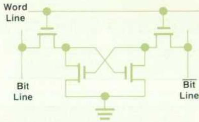
Fig. 2. Four-transistor dynamic storage cell.
