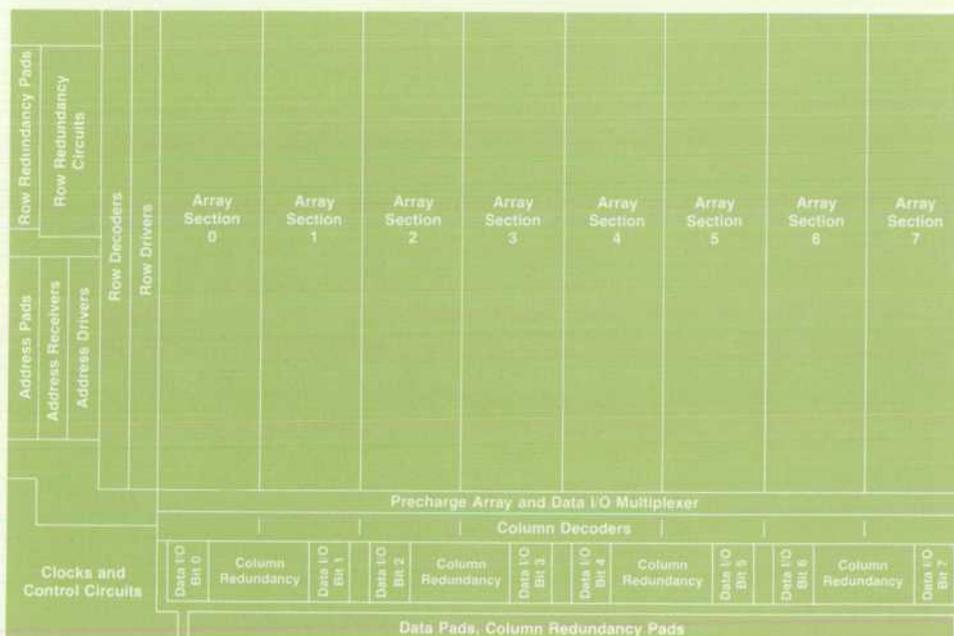
**Fig. 1.** Physical layout of 128K-bit NMOS dynamic RAM.
