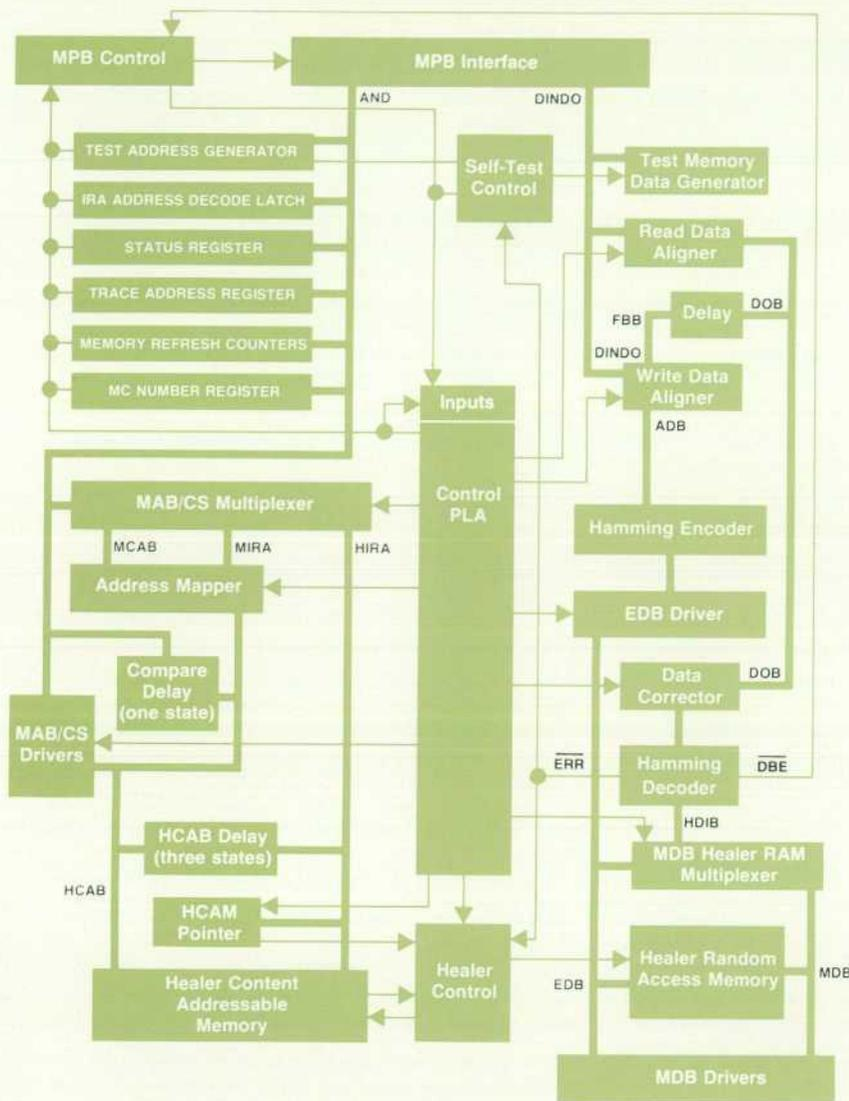
Fig. 3. Block diagram of memory controller chip architecture.
