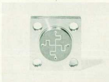
Fig. 6. The low-pressure compliance (LPC) connects the metering pump to the high-pressure pump. The contributions of the three solvent channels are combined in the mixing chamber (photo). The deflection of the diaphragm of the LPC is measured by a strain gauge system mounted on a prestressed spring.
