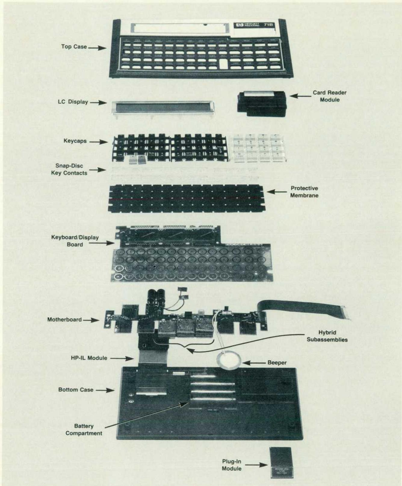
**Fig. 1.** Exploded view of the HP-71B Computer showing the various packaging features. The mainframe is composed of two subassemblies: the top case assembly and the bottom case assembly. The top case assembly contains the keyboard, display, and CPU and display driver circuitry. The bottom case assembly contains the built-in memory, power circuits, and piezoelectric beeper, and accommodates the optional card reader/recorder and other plug-in modules.
