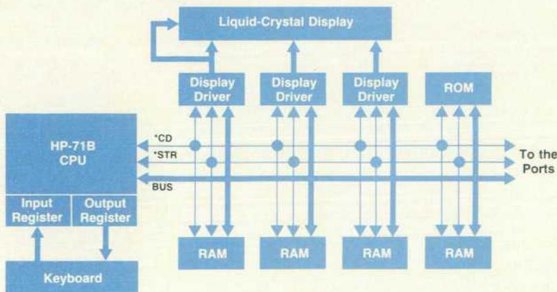
Fig. 1. Simplified block diagram of the HP-71B mainframe system electronics.
