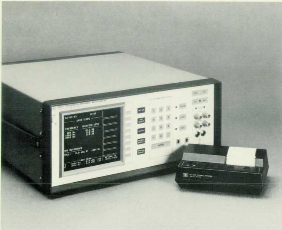
**Fig. 2.** The HP 4945A Transmission Impairment Measuring Set tests voice and data telephone circuits according to the Bell standards used in the U.S.A. and Canada. A choice of three control interfaces is offered for integrating the instrument into an automatic system. One of these, HP-IL, makes the new TIMS compatible with battery-powered controllers and peripherals, such as the printer shown here.
