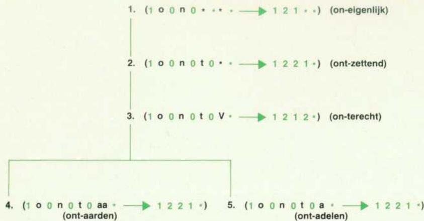
Fig. 1. This part of the tree of linguistic rules handles the prefix on(t). For example, in analyzing the pattern ontz, the hyphenation algorithm will search the tree until it finds rule no. 3, which does not apply. Rule no. 2 will then be used.
