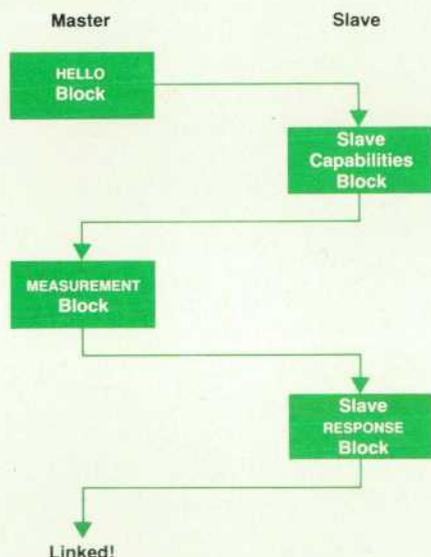
Fig. 1. Master/slave exchanges in the linkup phase.
