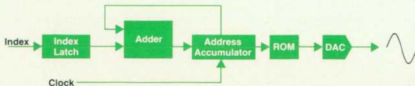
Fig. 4. This basic fractional-N synthesizer is modified to generate waveforms transmitted by the HP 4945A.
