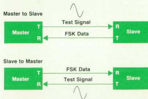
Fig. 2. Master/slave communication in the measurement phase.
