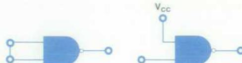
Fig. 2. Configurations of a NAND gate used as an inverter.
