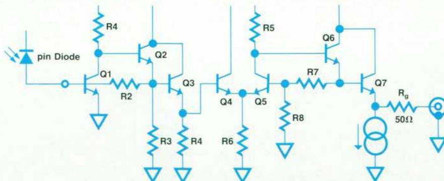
**Fig. 4.** Schematic diagram of the high-frequency amplifier.
