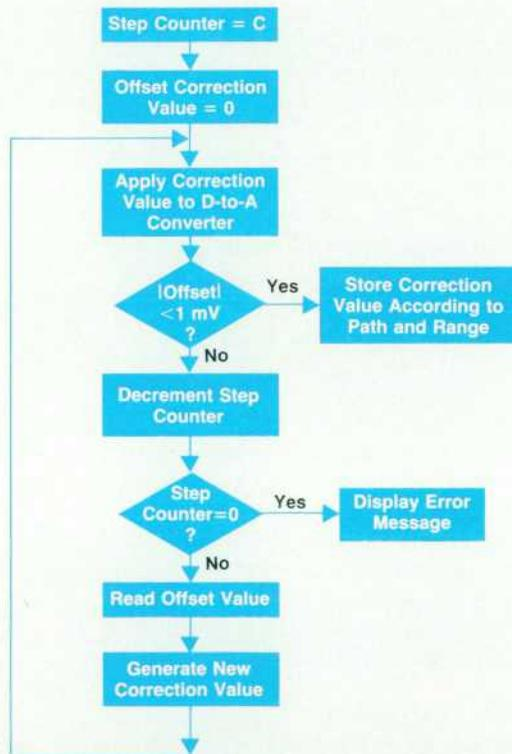
Fig. 13. Flow chart of the offset determination routine.
