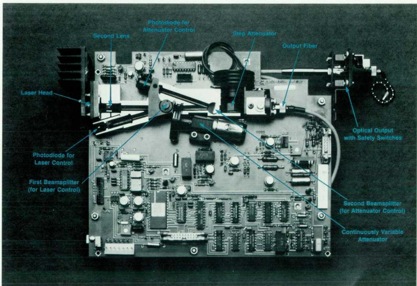
Fig. 13. The laser light is controlled and attenuated within this miniature optical bench. A solid metal block carries the optical elements.
