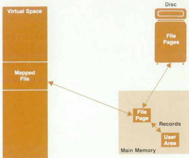
Fig. 8. Internal caching by means of file mapping.
