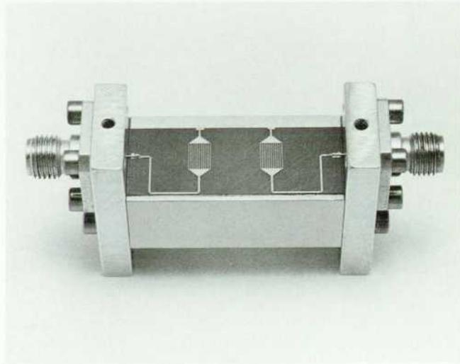
**Fig. 10.** Photographs of a narrowband MSW delay-line filter using seven-element transducer gratings on a 254- $\mu\text{m}$ -thick sapphire substrate with YIG film in place (left) and removed (right).
