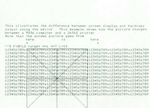
Fig. 5. Because the ratio of graphics dots to alpha dots varies from display to display and from printer to printer, text may look different on the screen (left) and in hard copy (right).
