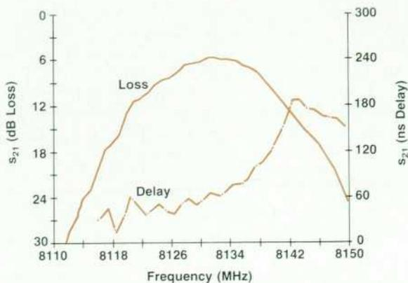
**Fig. 17.** Amplitude and delay response of an MSW delay line using an 18- $\mu\text{m}$ -thick YIG film, a 254- $\mu\text{m}$ -thick sapphire substrate, seven-element microstrip transducers, and an external magnetic bias field of 2140 oersteds.
