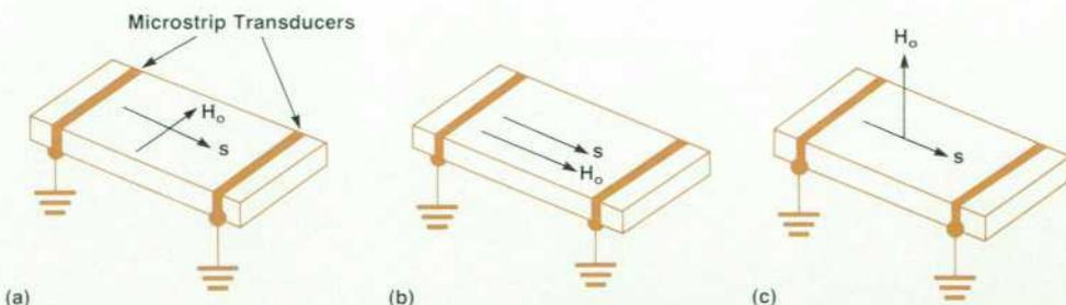
Fig. 1. Three magnetostatic wave modes as determined by the orientation of the propagation vector  $s$  and the direction of the external magnetic bias field  $H_o$ .<sup>3</sup> (a) Surface wave mode. (b) Backward volume wave mode. (c) Forward volume wave mode.
