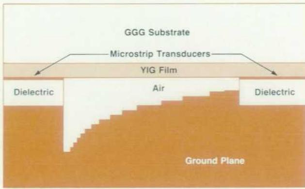
**Fig. 7.** Cross section of an MSW delay line using continuously varying YIG-film-to-ground-plane spacing<sup>6</sup> to linearize the dispersion characteristic (see Fig. 8).
