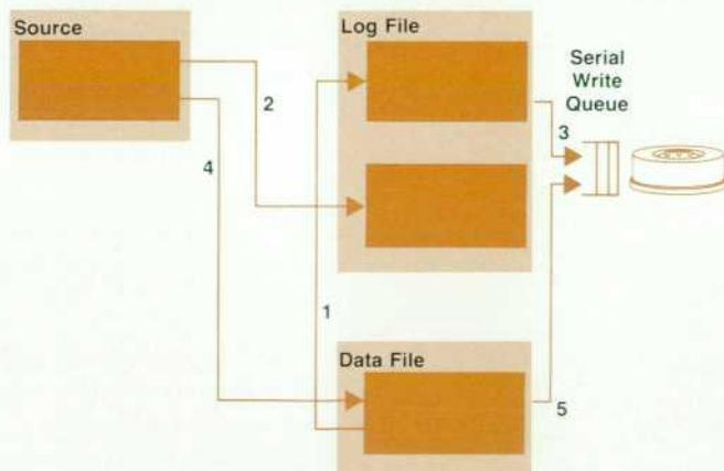
Fig. 19. Sequence of operations for write-ahead logging with serial posting. This mechanism was developed to minimize the probability of waiting for disc writes to complete.
