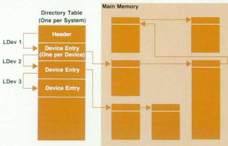
**Fig. 16.** Cached disc domain location mechanism used in the breadboard MPE kernel. A separate list is maintained for each disc, identifying the memory regions corresponding to currently cached domains from that disc.
