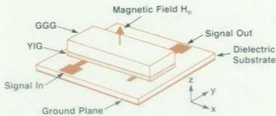
Fig. 4. Basic configuration of a magnetostatic-wave delay line.
