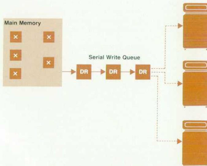
**Fig. 20.** To ensure disc consistency, only one write access for a serial write queue can be pending at any time. Multiple serial write queues can be used to allow parallel use of available disc drives for unrelated postings.
