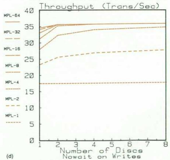
Fig. 10. Dependency on disc access time and the number of discs is dramatically reduced with disc caching, as shown here for file mapping.
