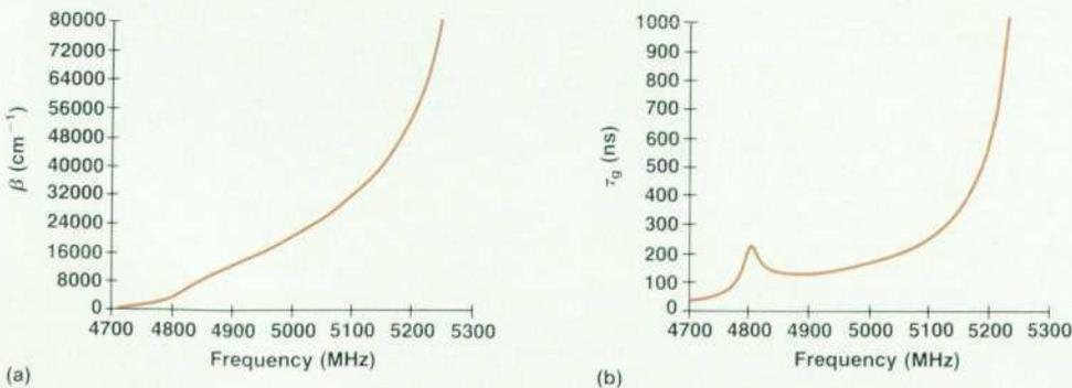
Fig. 5. Dispersion (a) and group delay (b) versus frequency for a magnetostatic-surface-wave delay line using a YIG film 20  $\mu\text{m}$  thick placed 254  $\mu\text{m}$  away from the ground plane. The applied magnetic bias field is 1000 oersteds and  $4\pi M = 1760$  gauss.
