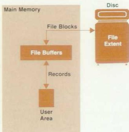
Fig. 5. Many systems provide limited disc caching in main memory on a subsystem, file, or application basis.
