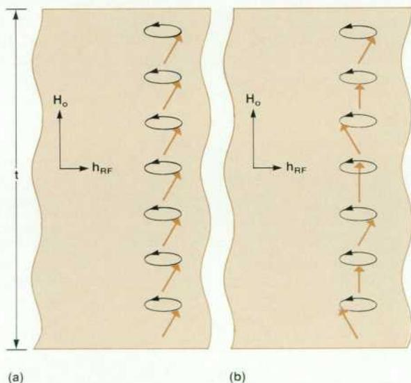
**Fig. 1.** Under the influence of uniform magnetic fields (a), the magnetic dipoles in a ferrimagnetic material precess at the same rate and have the same phase. For this case, the wavelength =  $\infty$ . If the RF magnetic field is not uniform (b), a volume spin wave is set up where the phase of neighboring dipoles differs slightly and this difference propagates with a wavelength =  $2t/3$ , where  $t$  is the thickness of the material.
