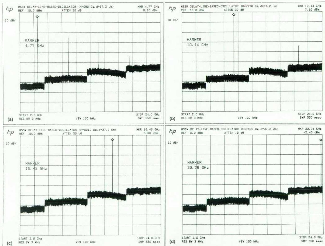
**Fig. 18.** Frequency response of circuit shown in Fig. 16 using the MSW delay line whose characteristics are shown in Fig. 17. This oscillator is tunable from 4 GHz to more than 24 GHz, as shown by the spectrum analyzer plots for oscillation at (a) 4.77 GHz, (b) 10.14 GHz, (c) 16.43 GHz, and (d) 23.78 GHz.
