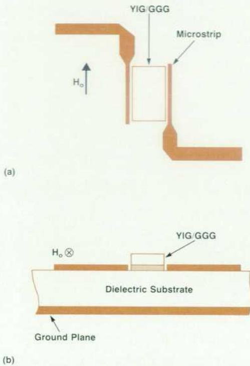
Fig. 12. Top (a) and side (b) views of basic straightedge MSW resonator structure.<sup>9</sup>
