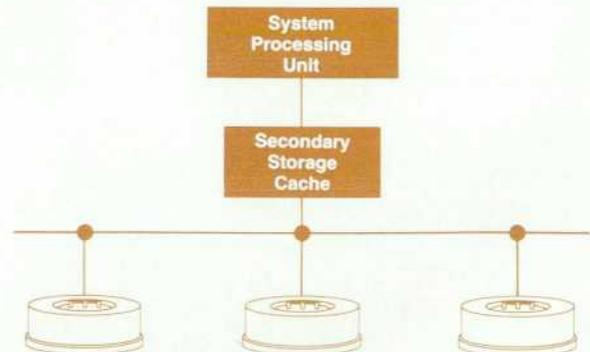
Fig. 4. External caching at an intermediate storage level.
