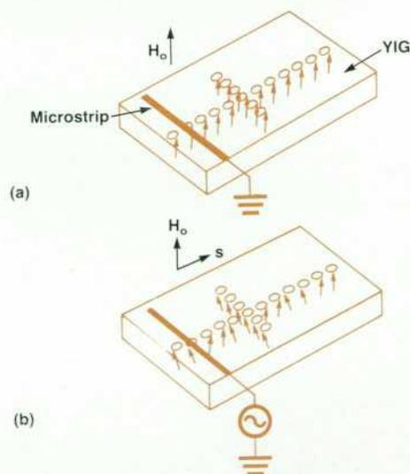
**Fig. 3.** (a) Under uniform field conditions, the magnetic moments in a thin ferrimagnetic film precess at the same rate and have the same phase. (b) When an RF field is applied to the microstrip transducer, a local perturbation of the magnetic field occurs, which then propagates through the film via the coupling of adjacent magnetic moments.
