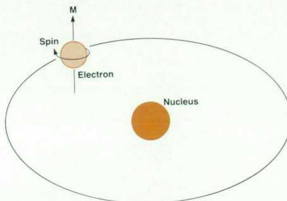
**Fig. 1.** In a crystal of ferrimagnetic material, the spinning electrons circulating around the nuclei of the atoms forming the crystal lattice generate a strong magnetic moment  $M$  that precesses around the direction of an external magnetic field.
