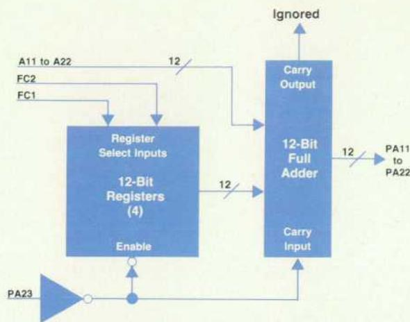
Fig. 3. Block diagram of memory management unit.
