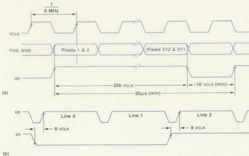
**Fig. 11.** Timing diagrams for interface signals between the display system and the rest of the Integral PC electronics. (a) Horizontal sync versus video clock and pixel enables. (b) Horizontal sync versus vertical sync.
