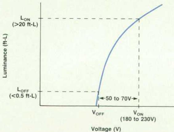
Fig. 4. Typical luminance-versus-voltage curve for electroluminescent display.
