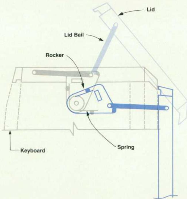
**Fig. 3.** Top lid hinge mechanism. (Gray) Closed. (Shaded color) Partially open. (Solid color) Open.
