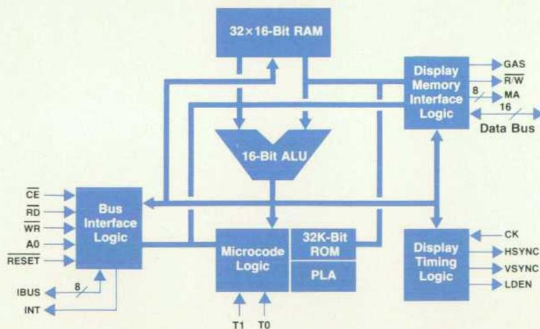
Fig. 1. Block diagram of custom graphics processor unit for the Integral PC.
