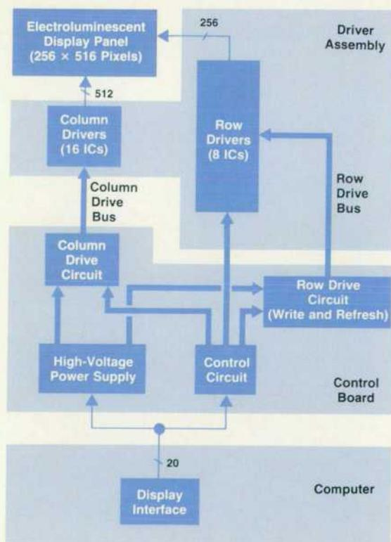
Fig. 2. Block diagram of Integral PC display system.
