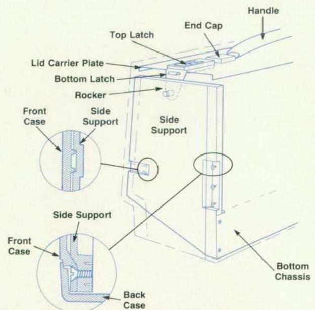
Fig. 2. Details of handle and side support assemblies.
