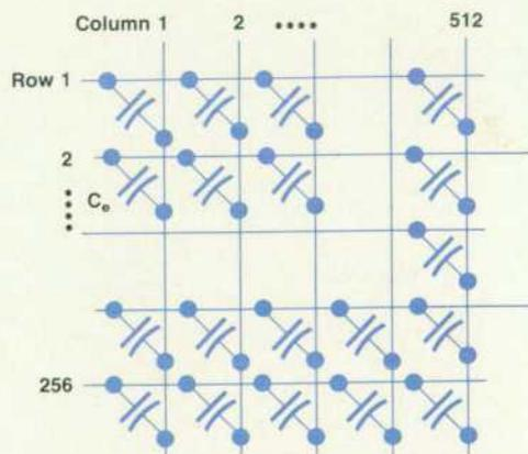
Fig. 7. Each pixel of the electroluminescent display contributes a capacitance  $C_0$  that must be charged and discharged by the driver ICs.
