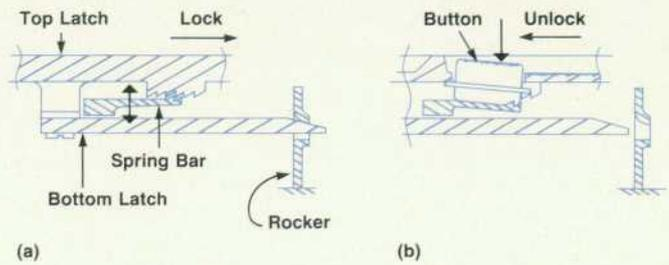
**Fig. 4.** Latch operation. (a) Locking, edge cross section of mechanism (button not shown). (b) Unlocking, center-line cross-section of mechanism showing caged release button. See Fig. 2 for perspective view.
