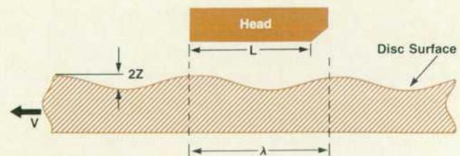
Fig. 7. Disc surface waviness model.  $L$  = length of air bearing surface.
