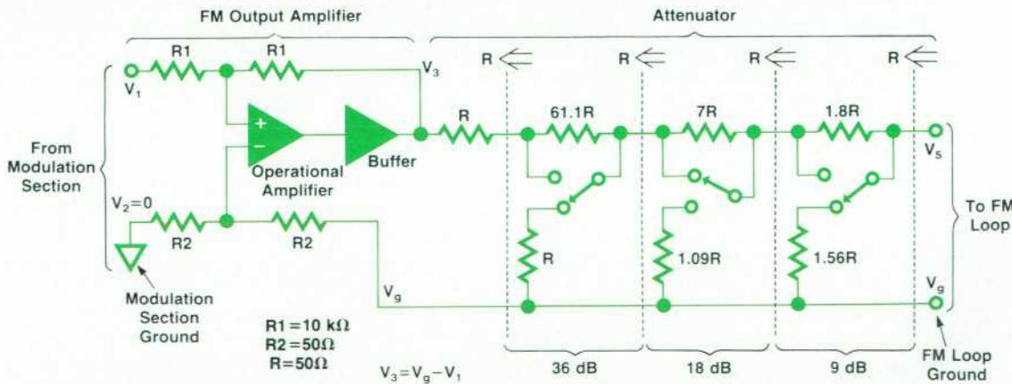
Fig. 2. FM output attenuator with floating ground.
