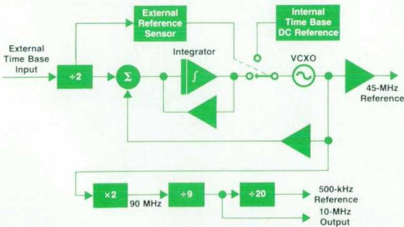
**Fig. 2.** Time base loop block diagram.
