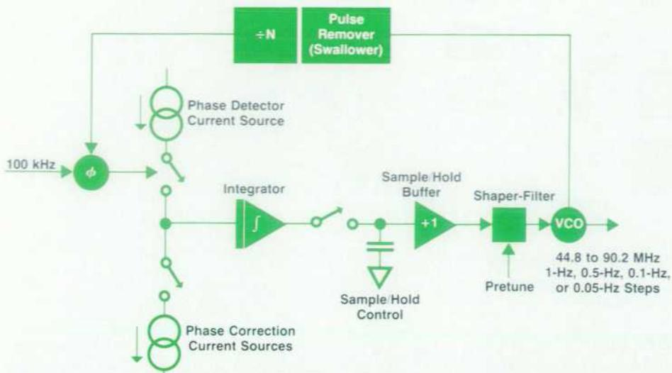
**Fig. 5.** IF loop block diagram.
