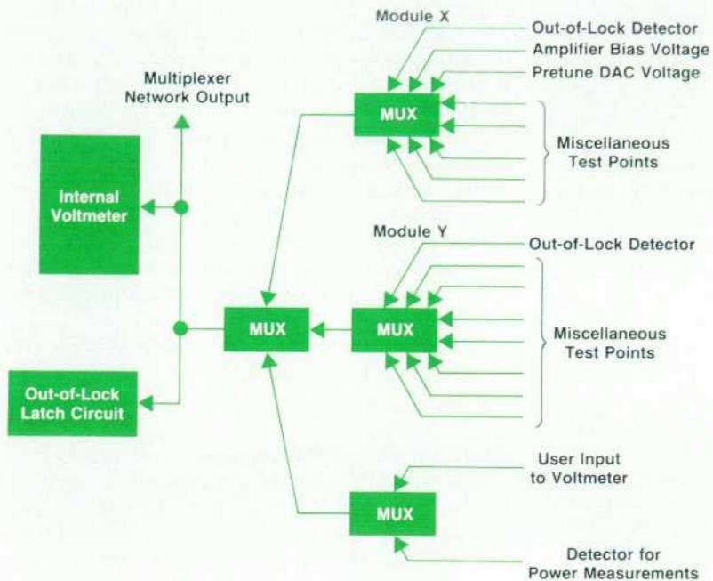
**Fig. 2.** To minimize connections through casting walls, only one service feedback line is allocated to each module. These lines are connected in parallel to the out-of-lock latches and an analog multiplexer, which selects one line for the voltmeter.
