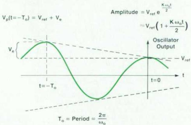
Fig. 7. Optimization of ALC loop gain.
