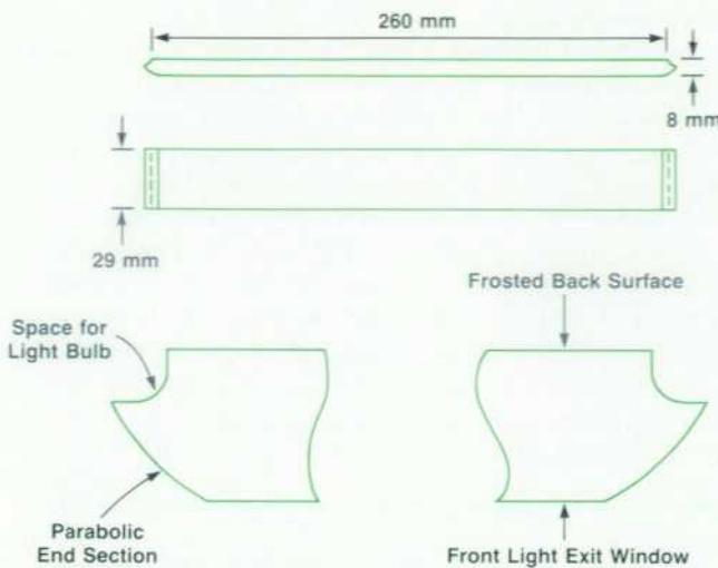
**Fig. 5.** Backlight detail.
