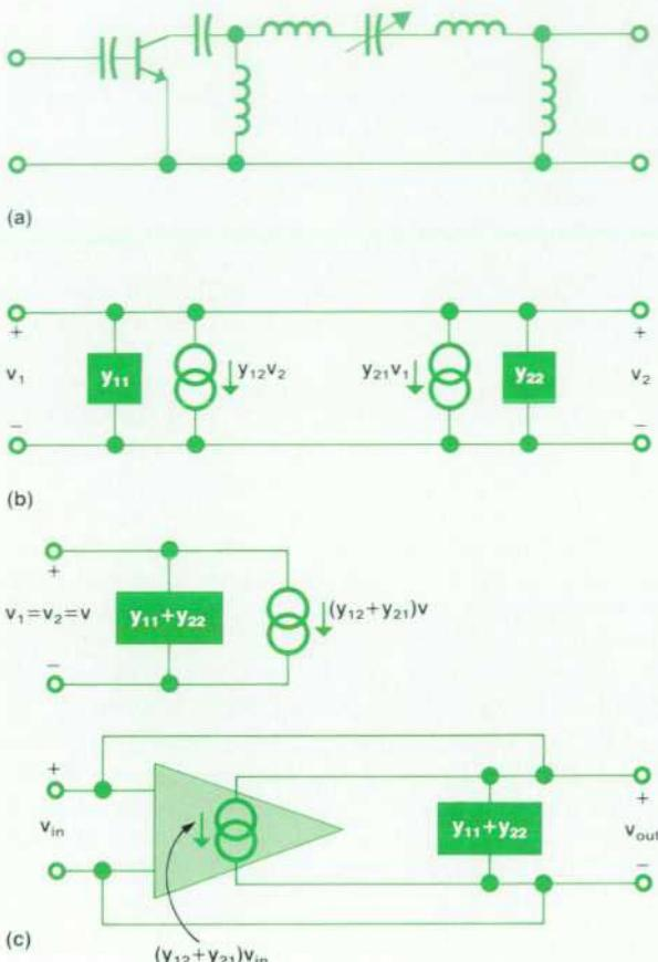
**Fig. 1.** (a) Oscillator circuit drawn as ideal amplifier with feedback loop opened. (b) S-parameters converted to y-parameters. (c) Loop closed and circuit redrawn as an ideal amplifier with feedback.
