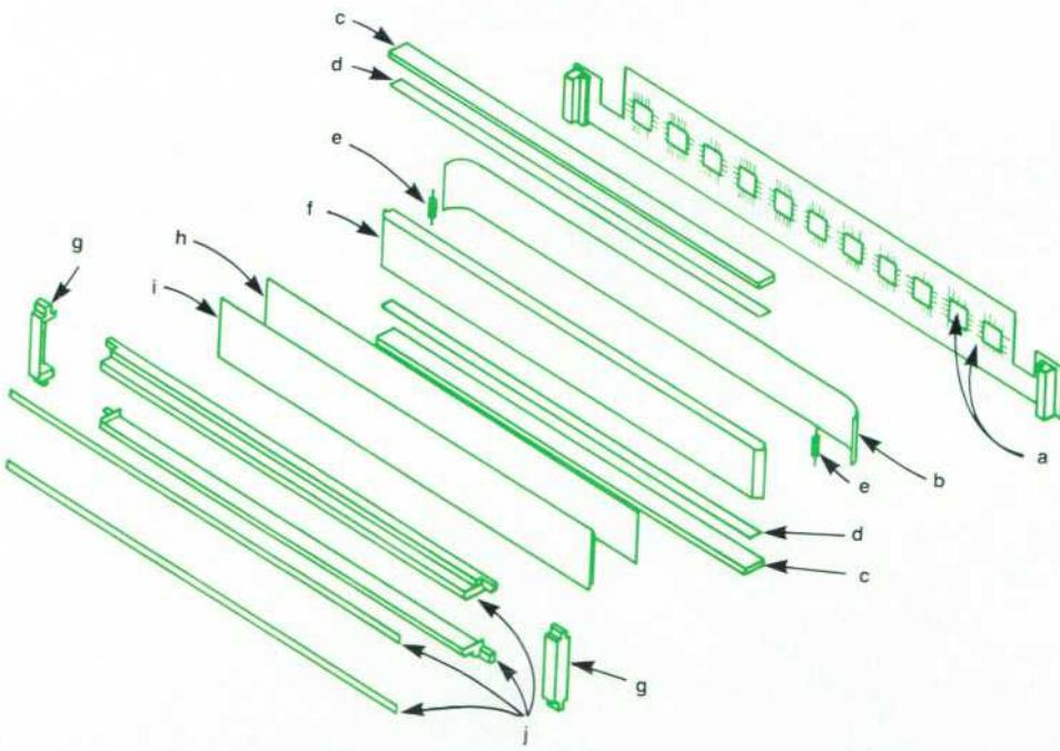
**Fig. 4.** LCD display construction.
