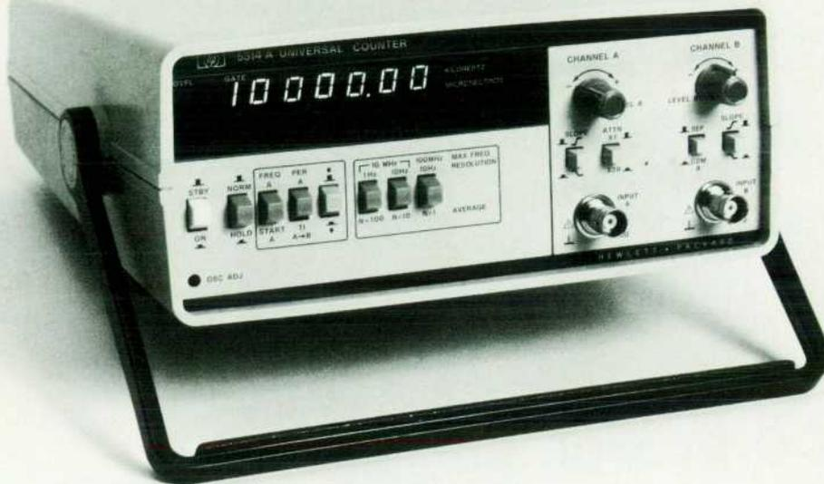
Fig. 1. HP 5314A front panel.
