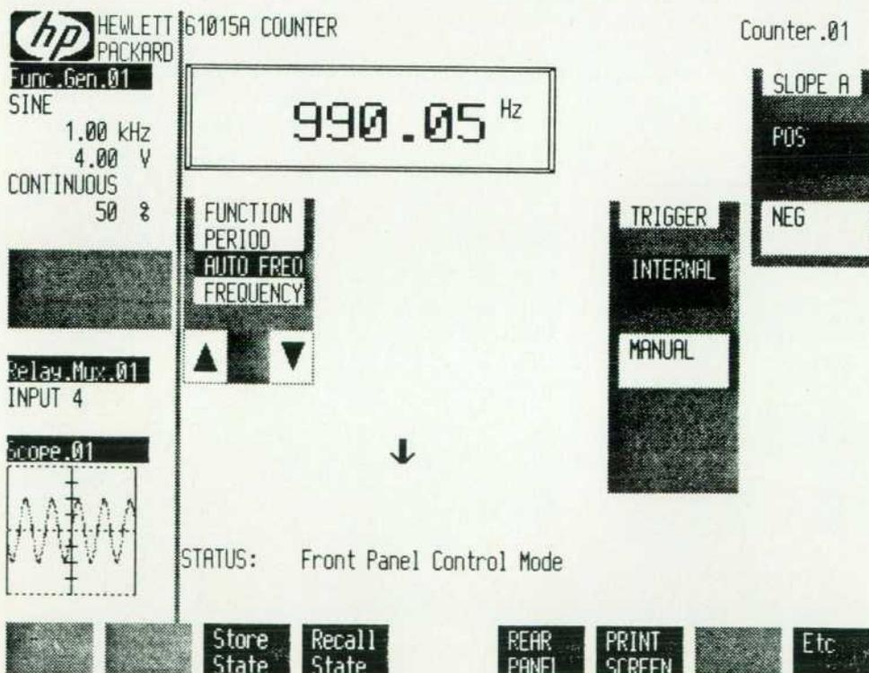
Fig. 2. Counter soft front-panel display in autofrequency operation.
