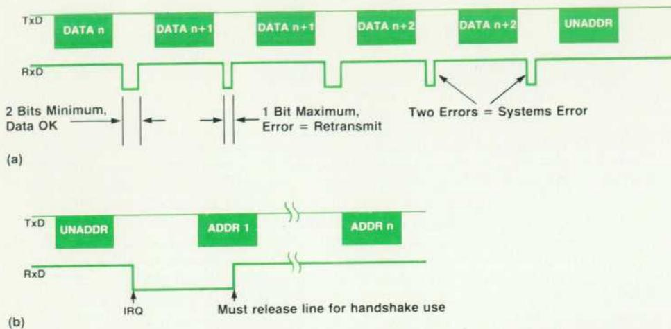
**Fig. 5.** PCIB serial communications. (a) Error handshake. If there is no acknowledgment, error or data OK handshake, a system error will result. (b) IRQ protocol. After an unaddress command, an instrument may signal on RxD to indicate that an interrupt is requested. The instrument must release RxD when any transaction is sent on TxD.
