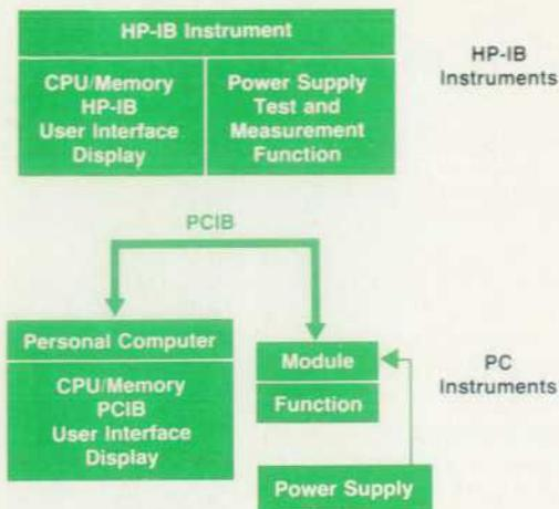
Fig. 2. Difference in HP-IB and PCIB architectures.
