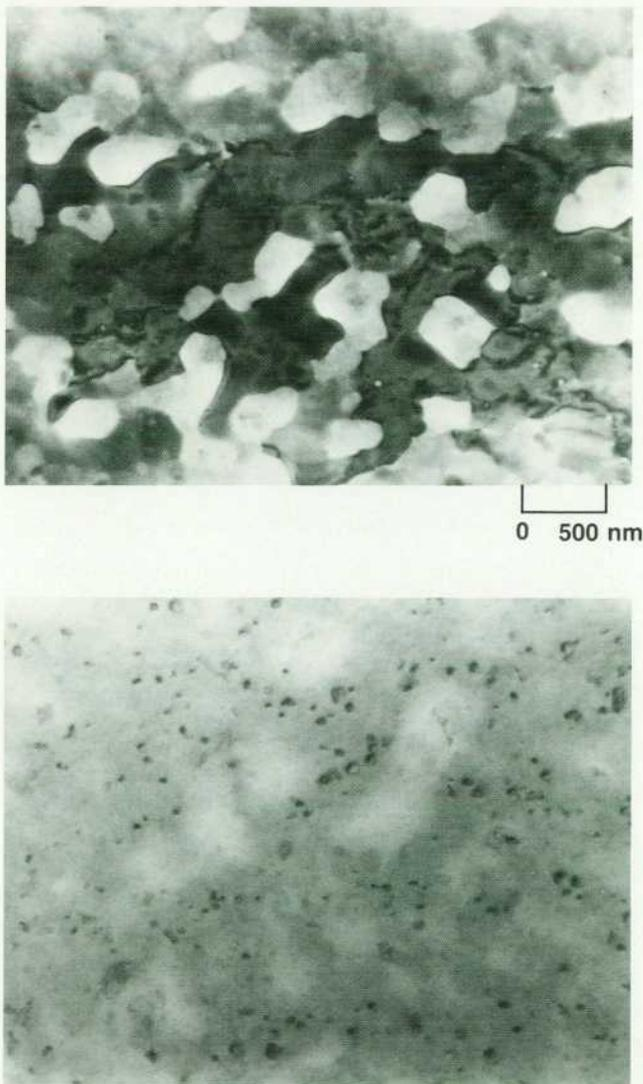
**Fig. 7.** TEM photomicrographs of the  $TiSi_2$  layer after annealing for 60 minutes at  $900^\circ C$  in a vacuum (top) and the silicon substrate with the  $TiSi_2$  layer chemically removed (bottom).
