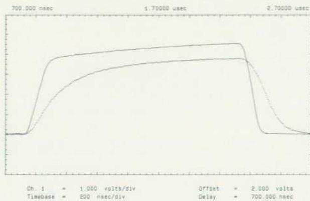
**Fig. 2.** Difference in rise and fall times (room temperature) for a 10:1 ratio of capacitive load, same custom IC and axis scaling. Capacitance varies from 130 pF to 1.3 nF. Actual pulse widths on the PCIB are much longer.
