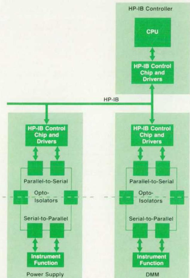
Fig. 1. Typical HP-IB system with isolated instruments.
