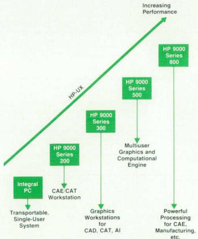
Fig. 3. The HP-UX computer family and its applications.
