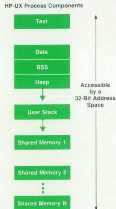
**Fig. 8.** AT&T's UNIX System V Interface Definition implies that processes have the following components: text, data, uninitialized data, a user stack, a heap, and zero or more shared memory segments. The user stack may grow automatically to suit the procedure call nesting of the process. The heap will grow (or shrink) when the process requests more (or less) memory using the `brk` or `sbrk` system calls.
