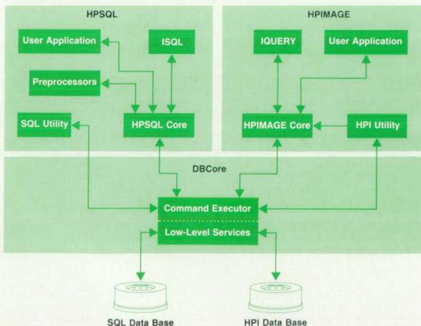
Fig. 2. HP ALLBASE product structure. HPSQL is the relational user interface. HPIMAGE is the network user interface. DBCore is used by both interfaces.
