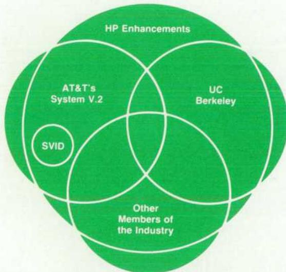
Fig. 2. Origins of the HP-UX operating system.
