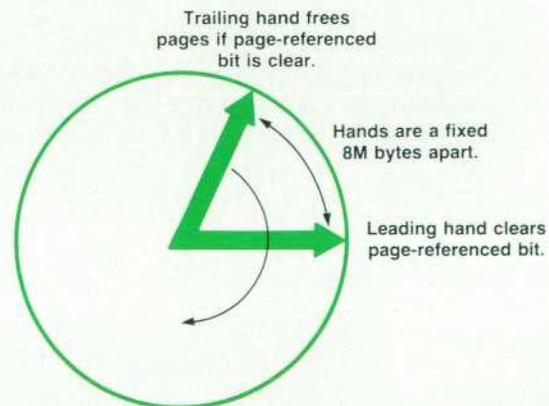
**Fig. 11.** The global clock algorithm is used to approximate a least recently used page-replacement algorithm. In this algorithm, the pages of real memory are depicted as wrapped around the edge of a clock. A pair of hands sweeps around the clock, with the leading hand clearing the page-referenced bit, and the trailing hand freeing pages that have not been referenced.
