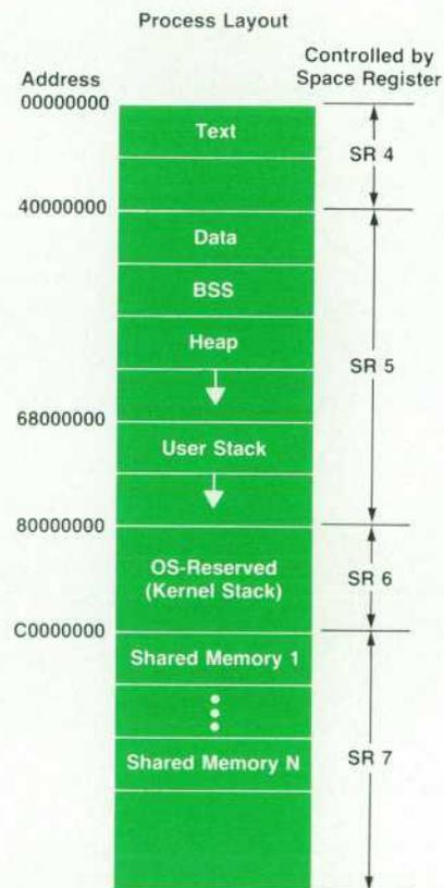
**Fig. 9.** The components of an HP-UX process are mapped onto HP Precision Architecture as shown. The kernel stack is a stack used only while the kernel is executing on behalf of the process, and it is otherwise inaccessible to the process. The kernel is not included in the short-pointer address space of the process. Rather, it executes out of a separate space (0) and it accesses the memory of the process using a handful of functions that use long-pointer addressing mode.
