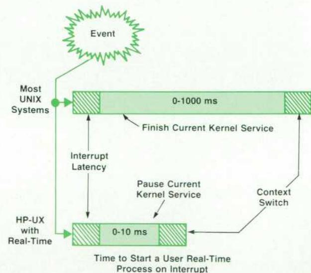
Fig. 6. HP-UX real-time extensions achieve an order of magnitude improvement in preemption latency over traditional UNIX systems.
