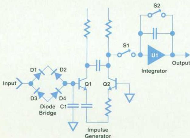
Fig. 6. Sampler schematic.
