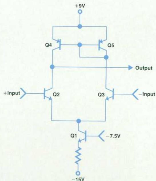
Fig. 14. Differential limiter circuit.
