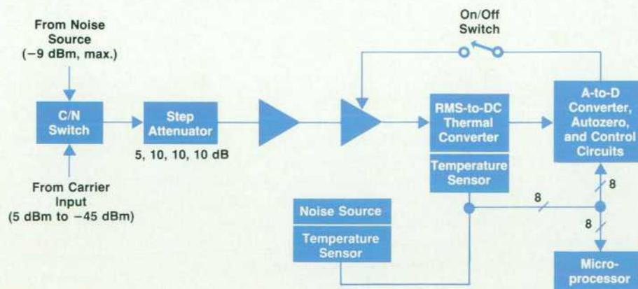
Fig. 1. Block diagram of the HP 3708A's internal power meter.
