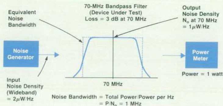
Fig. 1. Derivation of noise bandwidth NBW from total output power and output noise density at 70 MHz.
