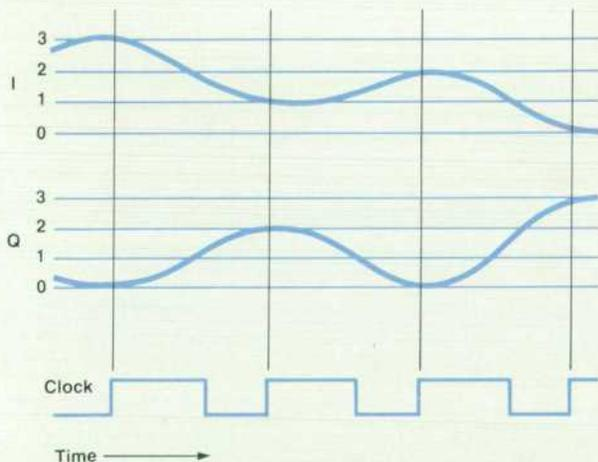
**Fig. 3.** Typical baseband and symbol clock waveforms for a 16QAM radio system. The two channels, I and Q, have four possible states: 0, 1, 2, and 3. The waveforms are filtered to conserve bandwidth, so they look more sinusoidal than square. At the valid edge of the clock (leading edge) the I and Q data will be at one of the four levels.
