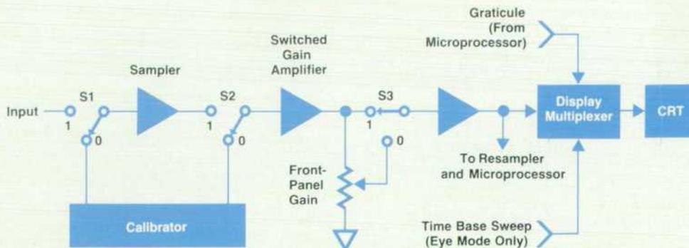
**Fig. 12.** Analog signal processing. Four functions are performed: 1) input signal displayed on CRT ( $S1 = S2 = 1$  and  $S3 = 0$ ), 2) graticule is displayed on CRT, 3) front-panel gain potentiometer is measured ( $S1 = S2 = S3 = 0$ ), and 4) sampler is calibrated ( $S1 = 0$  and  $S2 = S3 = 1$ ).
