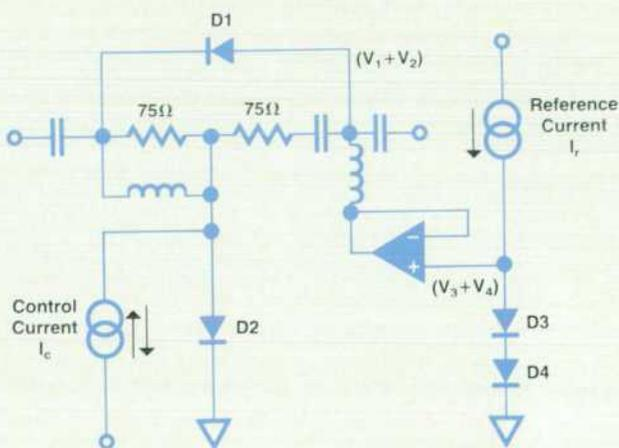
Fig. 3. Method for biasing bridged-T pin diode attenuator to maintain its characteristic impedance with varying temperature.  $V_1 + V_2 = V_3 + V_4$ .
