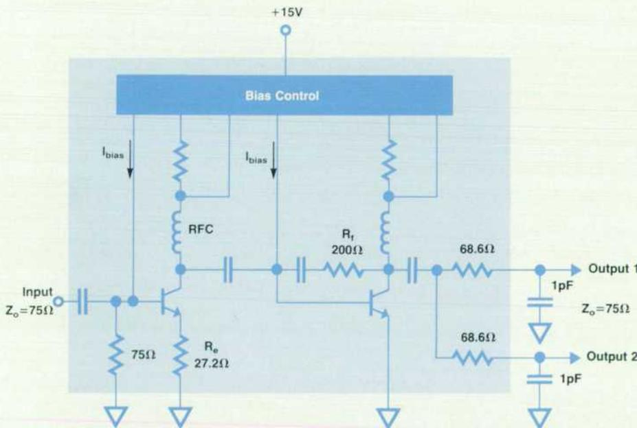
Fig. 1. Schematic of wideband thick-film amplifier.
