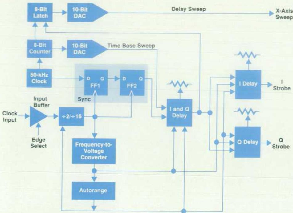
Fig. 8. Time base block diagram.
