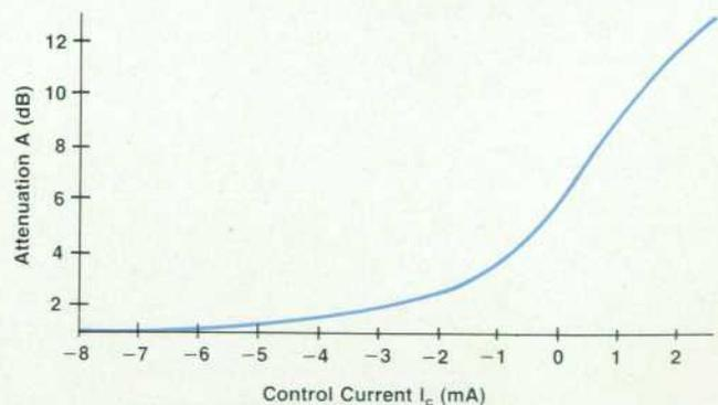
Fig. 4. Plot of attenuation versus control current for equation 7 with  $a = 1.563$ ,  $b = 1.31$ , and  $d = 0.8$ .
