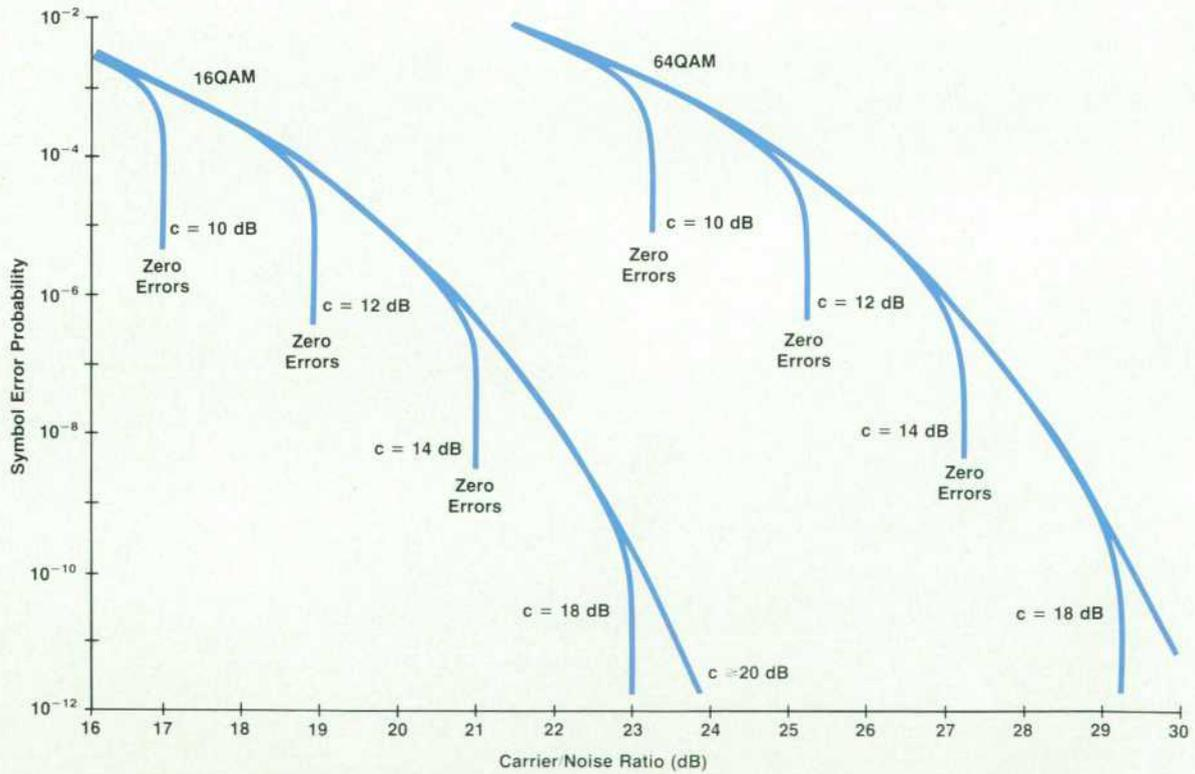
**Fig. 2.** Probability of symbol error versus CIN ratio for finite noise crest factor  $c$  for  $N$ -phase PSK (phase shift keying) data transmission and (b) QAM (quadrature amplitude modulation) data transmission.
