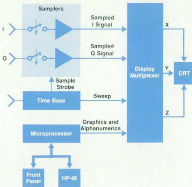
Fig. 5. Block diagram of HP 3709A Constellation Display.
