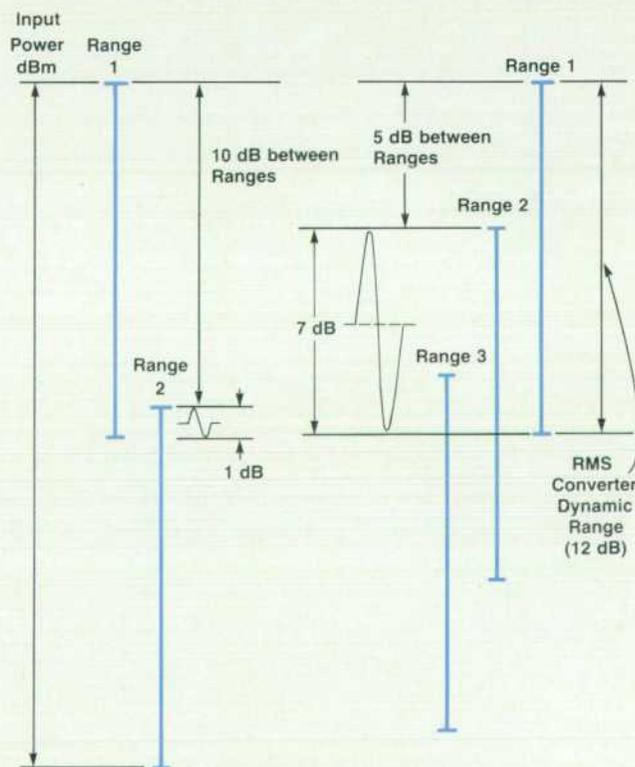
Fig. 3. Power meter ranges. With 10-dB differences between ranges (left), a signal greater than 1 dB peak-to-peak may require a range change. With 5-dB differences between ranges, as in the HP 3708A (right), a signal must vary in level by at least 7 dB to effect a change in range.
