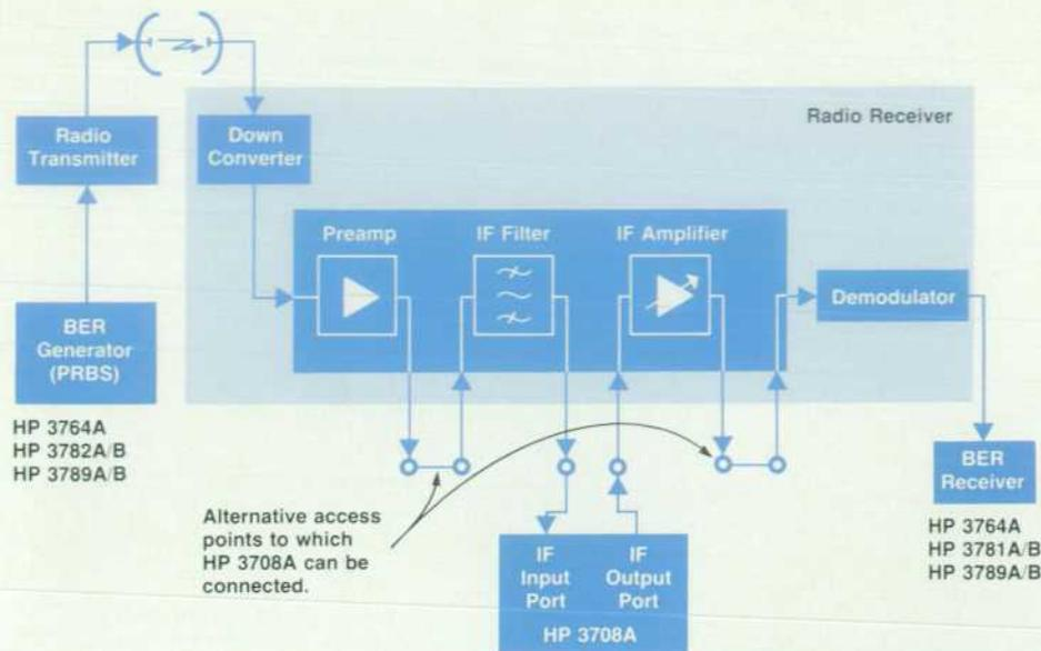
Fig. 3. Typical test configuration using HP 3708A Test Set.
