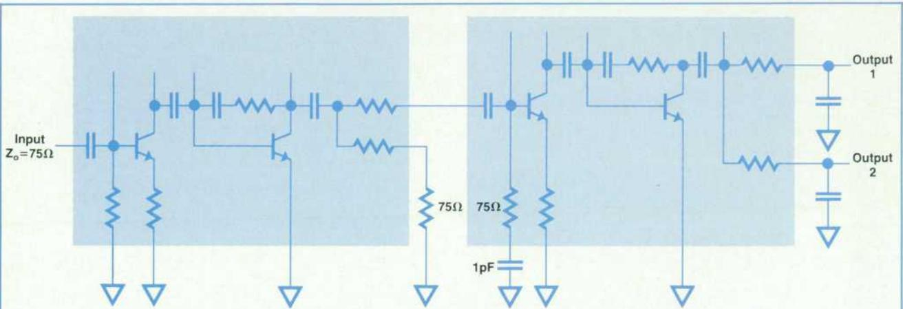
Fig. 2. Connection of two hybrid circuit amplifiers in HP 3708A Test Set to obtain 26-dB gain.
