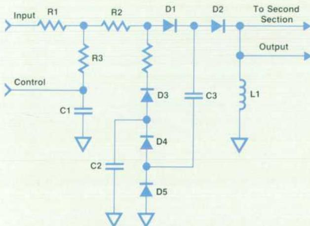
Fig. 2. C/N pin diode switch (one of two channels).
