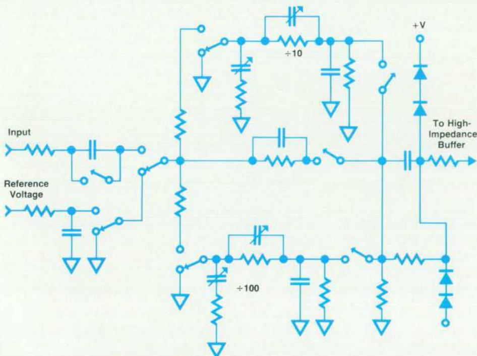
Fig. 1. HP 5183A Waveform Recorder input attenuator.
