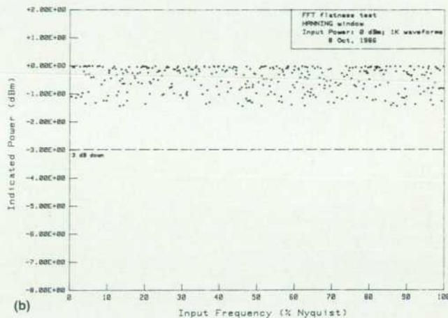
Fig. 11. (a) Accuracy of the flattop window is demonstrated by a series of spectra of 0-dBm sine waves at random frequencies. (b) The Hanning window is less accurate but has superior frequency resolving properties.
