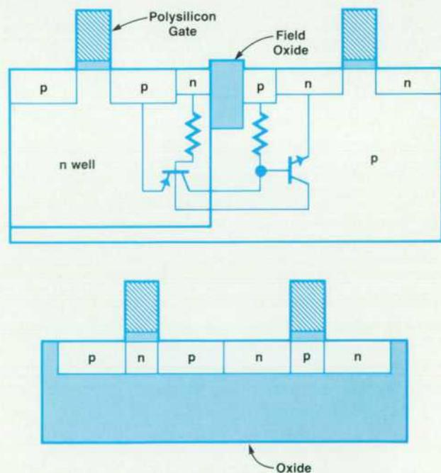
**Fig. 1.** Cross-sections of CMOS inverters made using bulk-silicon (top) and SOI (bottom) technologies. Resistors and bipolar transistors in the bulk device symbolize the nnp latch-up path.
