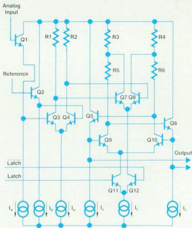
Fig. 5. Quantizer IC comparator cell schematic.
