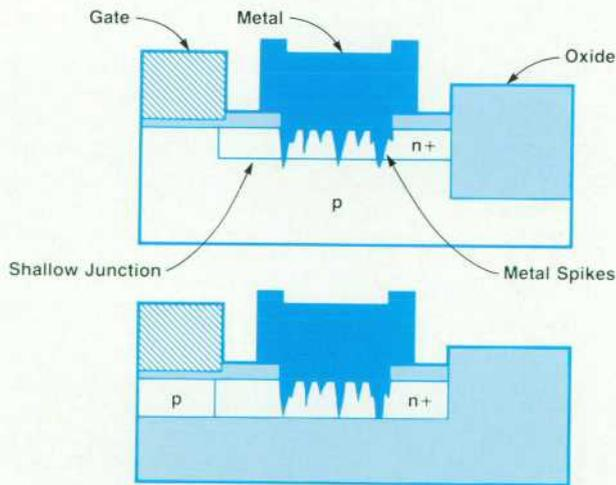
**Fig. 2.** Illustration of metal spikes punching through a shallow junction in a bulk transistor (top). In the case of an SOI device (bottom) where the source and drain regions extend throughout the entire film thickness, no junction punchthrough is possible.
