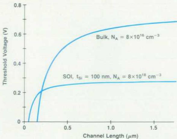
**Fig. 10.** Calculated threshold voltage in *n*-channel transistors as a function of channel length. The top curve represents a bulk device, while the bottom curve represents an SOI device. Both transistors have the same constant channel boron doping profile ( $8 \times 10^{16}/\text{cm}^3$ ). The SOI transistor is made in a 100-nm-thick silicon film.
