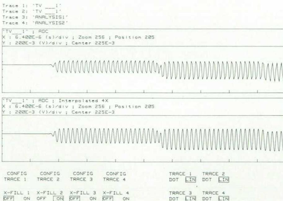
**Fig. 8.** Phase change in the color burst signal without and with reconstruction.
