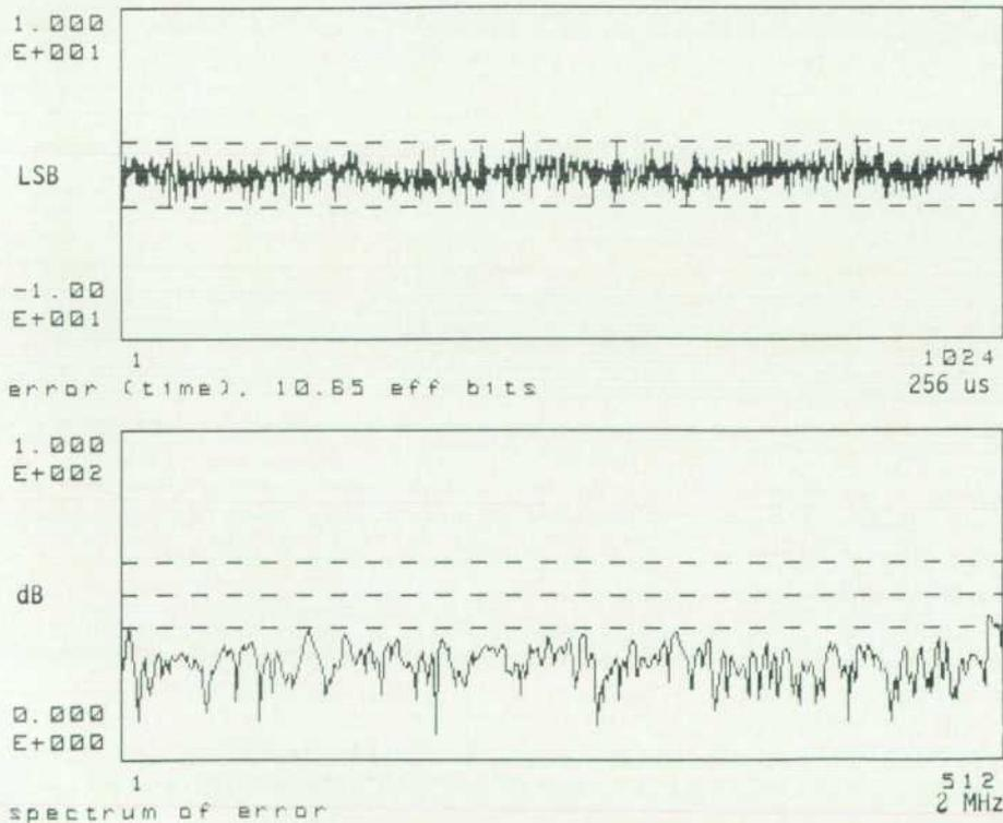
**Fig. 8.** (Top) Error in curve fit test for a test sine wave at 0.985 MHz. (Bottom) Frequency spectrum of the error.
