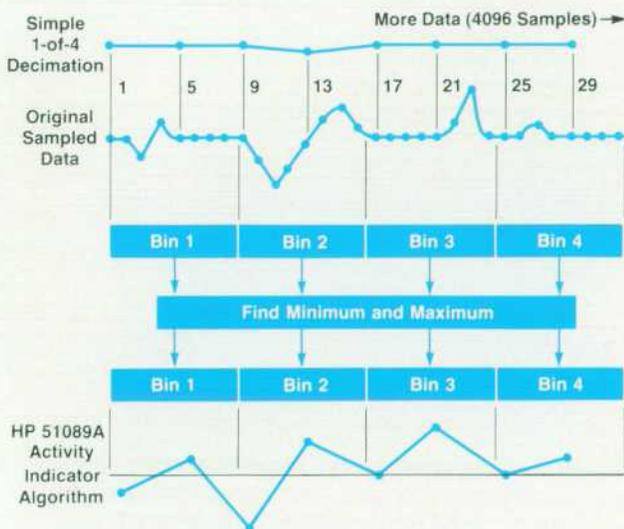
Fig. 5. The compression algorithm in the HP 51089A ensures that signal activity is never missed.
