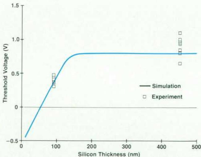
**Fig. 6.** Threshold voltage as a function of film thickness in *n*-channel SOI MOSFETs. The boron doping level is constant ( $8 \times 10^{16}/cm^3$ ), and the gate oxide thickness is 25 nm.
