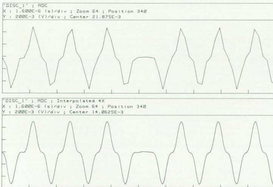
Fig. 10. A typical disc dropout without and with reconstruction.
