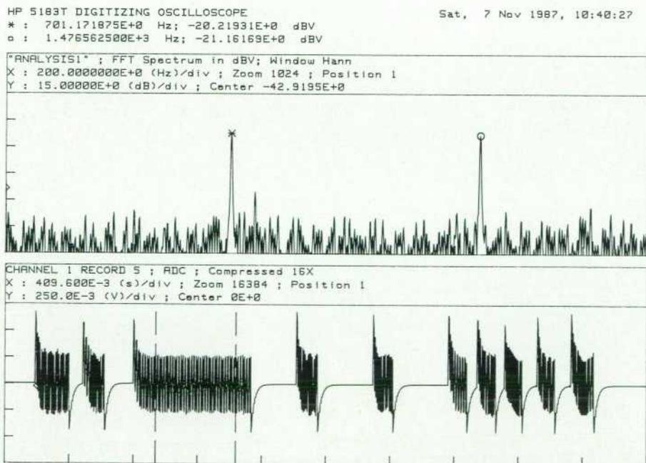
Fig. 10. (bottom) Time-domain display of a touchtone generator output. (top) Spectrum in dBV shows that the third key pressed was a 3.
