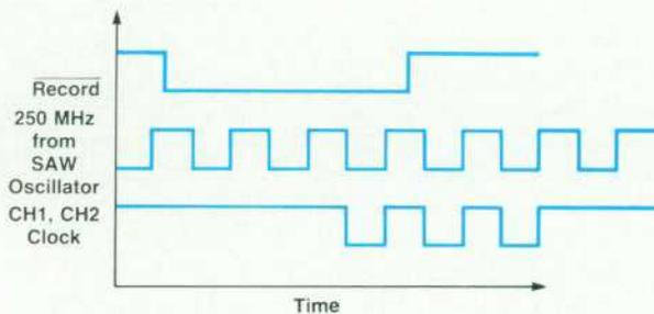
**Fig. 8.** Synchronous startup of the clocks in the two HP 5185A channels is guaranteed by a de-teeter circuit at the output of the 250-MHz SAW oscillator.
