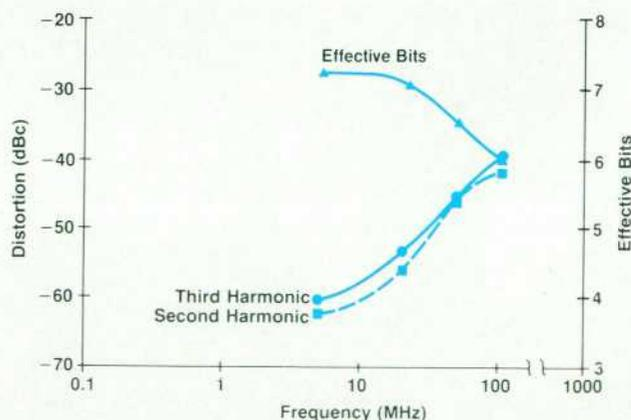
Fig. 7. Distortion and effective bits versus frequency for the analog-to-digital converter of the HP 5185A Waveform Recorder.
