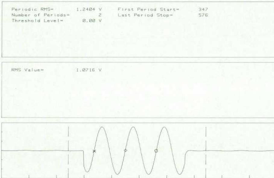
**Fig. 17.** The periodic rms function can avoid errors caused by inclusion of partial periods in the rms result.
