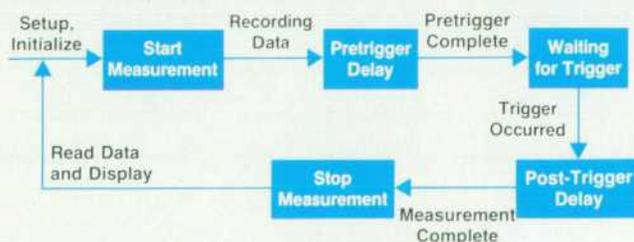
Fig. 2. Basic HP 5185A measurement sequence.
