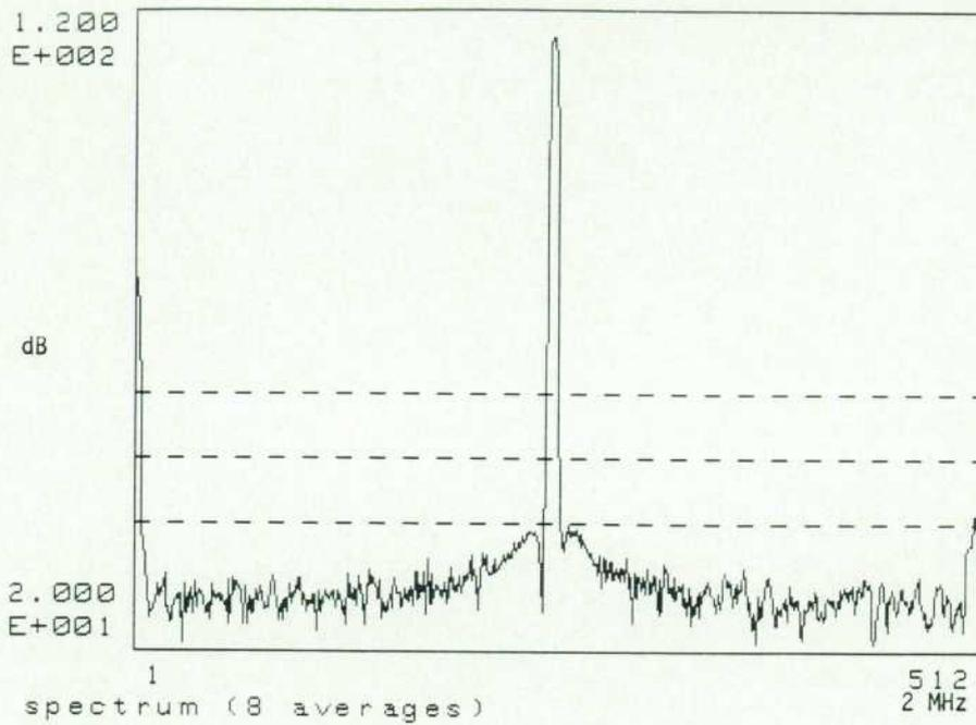
Fig. 9. Spectrum of a digitized 0.985-MHz sine wave.
