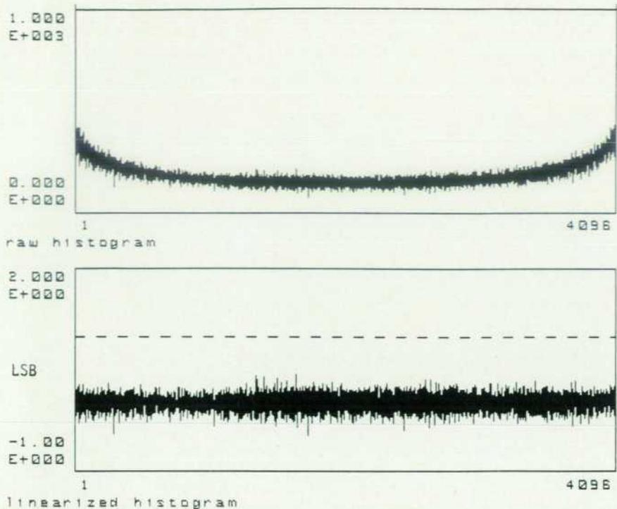
**Fig. 11.** Raw and linearized histograms show the ac differential nonlinearity of the ADC to be within  $\pm 1$  LSB.
