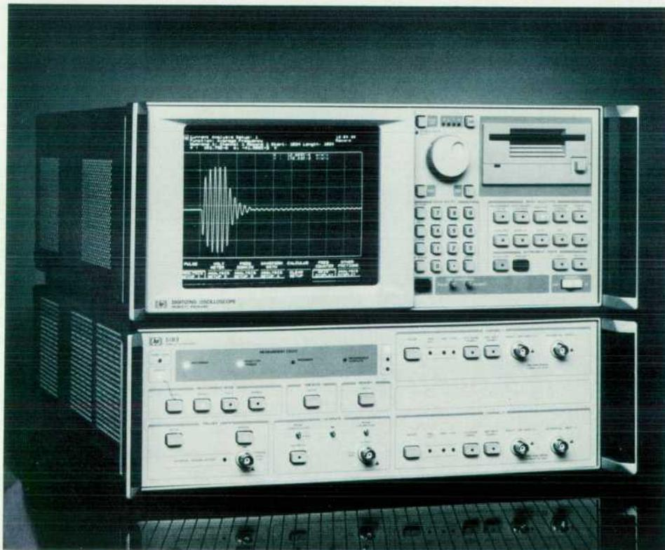
**Fig. 2.** The HP 5183T Precision Digitizing Oscilloscope consists of an HP 5183A Waveform Recorder and an analysis, display, and I/O section. The HP 5183A is a low-cost recorder that provides 4-MHz, 12-bit analog-to-digital conversion.
