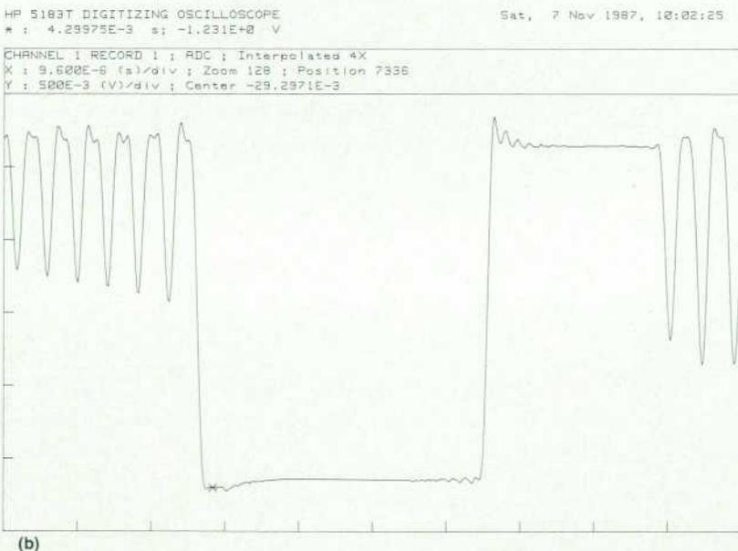
Fig. 6. (a) 16K-sample display shows a macro view of a function generator turn-on transient. (b) Display zoomed in on cursor, showing fine detail.
