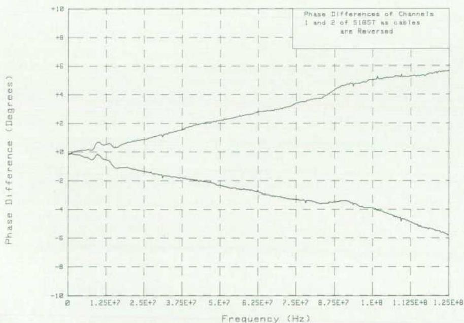
Fig. 12. A measurement with no device under test can be used to calibrate timing differences between HP 5180T, HP 5183T, or HP 5185T inputs.
