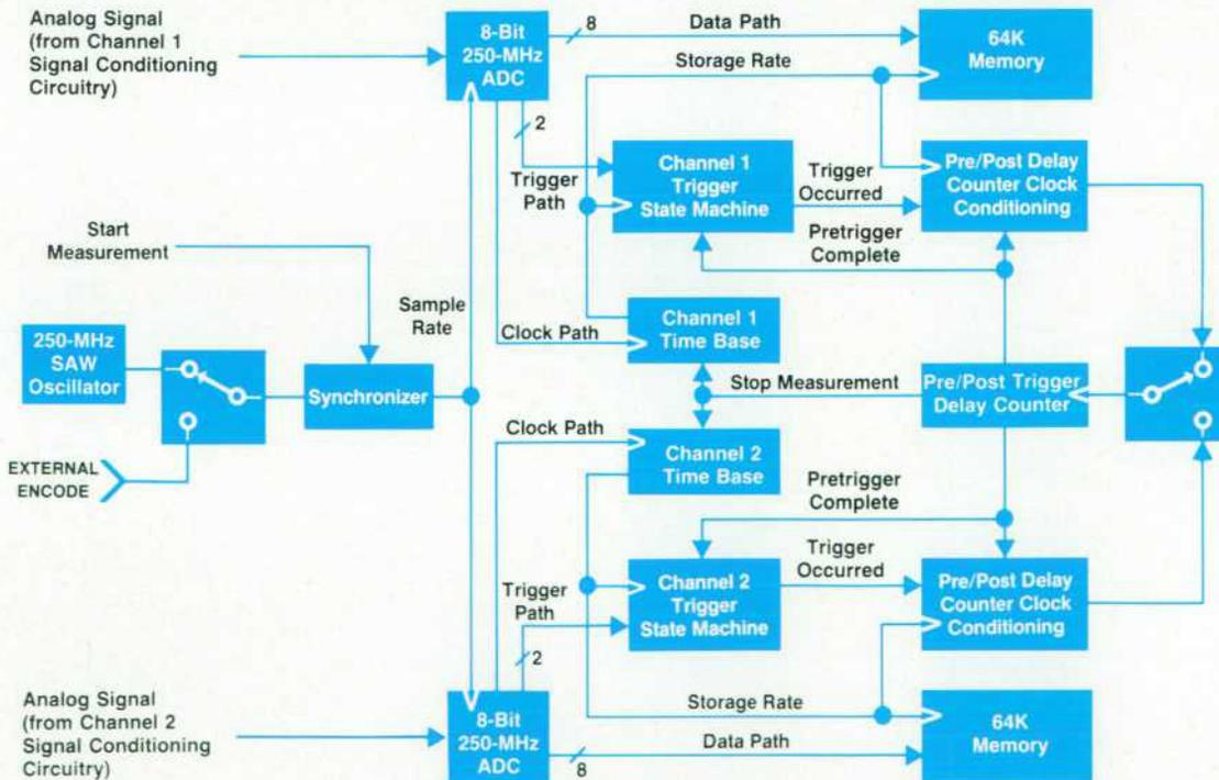
Fig. 1. HP 5185A high-speed digital system architecture.
