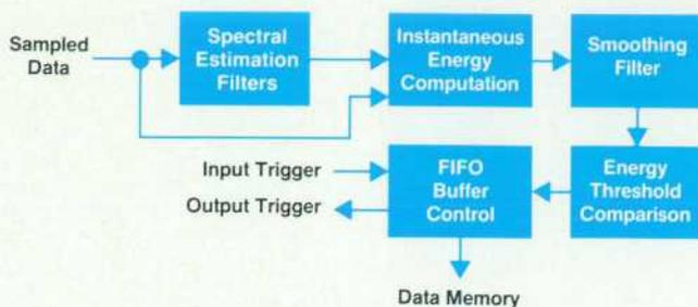
Fig. 2. Adaptive sample rate system single-channel data flow.
