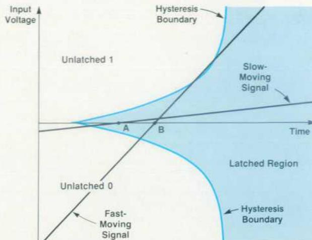
Fig. 9. Hysteresis boundary versus time for the latch of Fig. 8.
