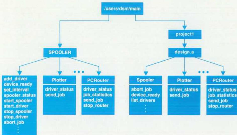
Fig. 3. DSM project and design hierarchy with spooler menus.
