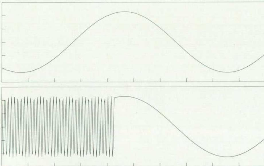
**Fig. 1.** HP 5183T display of the output of the adaptive sample rate circuit (bottom) and the reconstructed input waveform (top). The bottom waveform shows the actual memory contents. Before the trigger point, the input waveform is down-sampled; only one out of every 64 possible sample values is stored, making the display appear compressed. The top waveform shows that the original signal can be reconstructed from the stored data.
