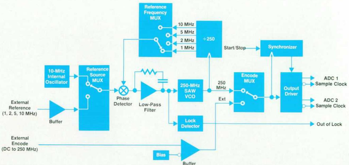
Fig. 13. 250-MHz SAW oscillator phase-locked loop system.
