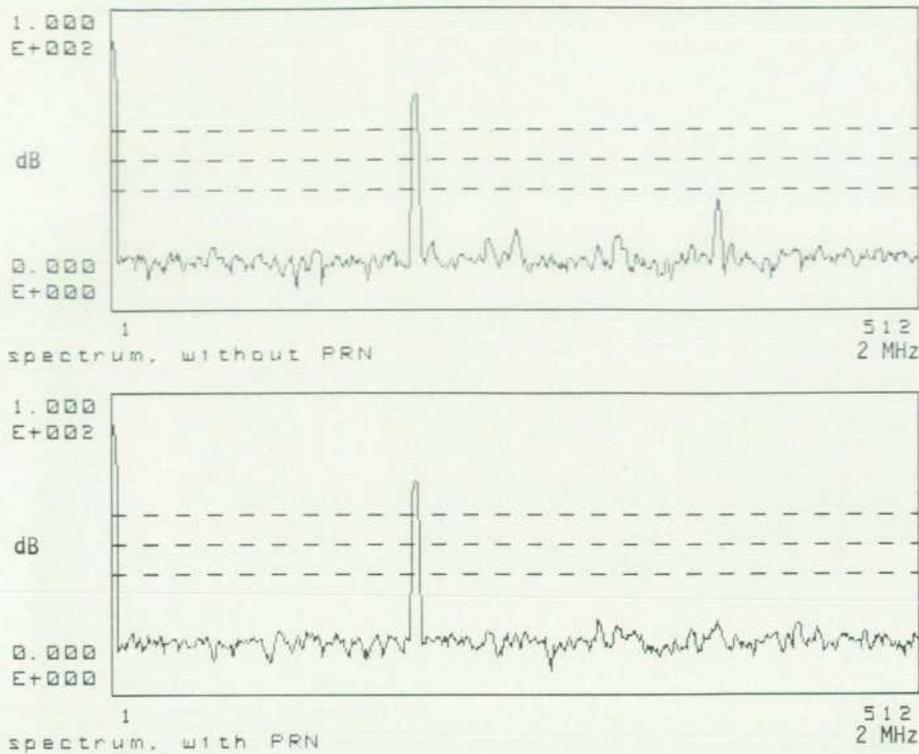
**Fig. 7.** Spectra of a digitized low-level sine wave with and without pseudorandom noise.
