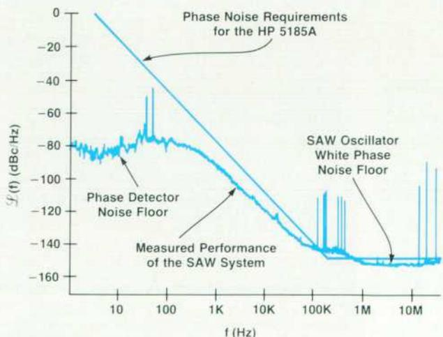
Fig. 12. Frequency-domain phase noise requirement and actual performance.
