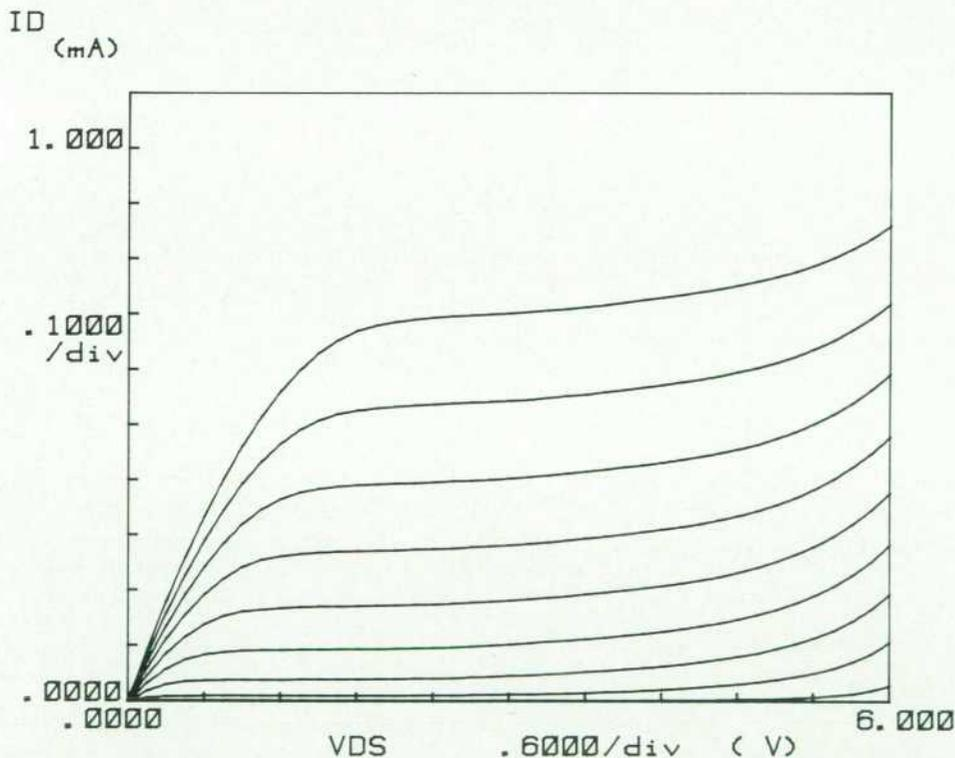
**Fig. 9.** Same device as in Fig. 8, but the backside gate voltage is now set to 0V. The kink in the output characteristics has disappeared since the device is now fully depleted. Gate voltage ranges from 0 to 2.5V in 0.25V steps.
