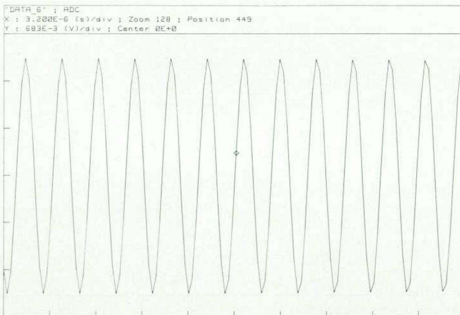
**Fig. 1.** HP 5180T display of a sinusoid captured using 10 points per cycle without reconstruction.
