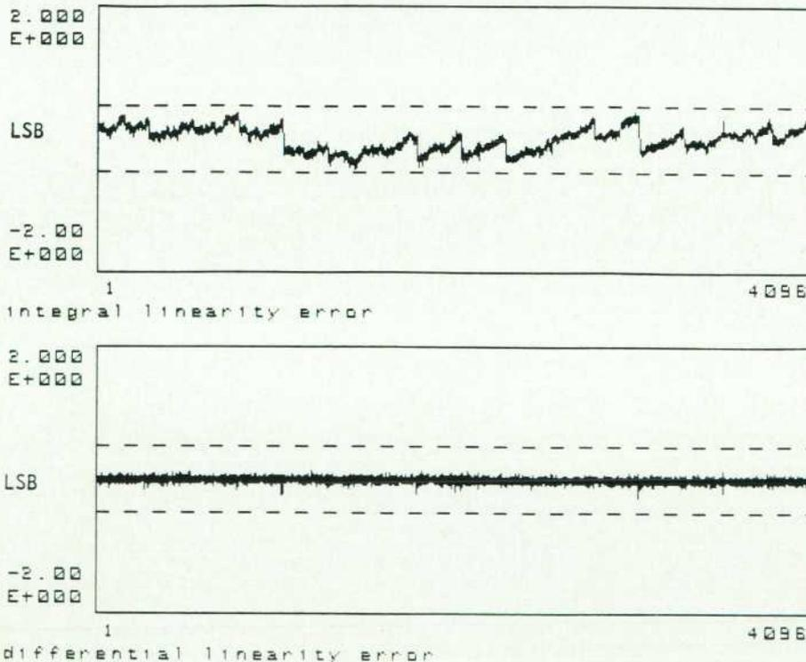
Fig. 10. Integral and static differential nonlinearity of the HP 5183A ADC.
