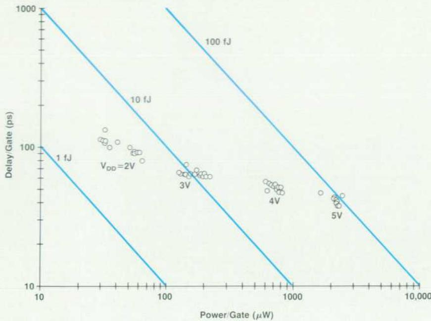
**Fig. 4.** Scatter plot of delay per gate versus power dissipation per gate in CMOS SOI ring oscillators. The straight lines represent different delay-power products. The effective channel lengths are 0.25 and 0.47  $\mu\text{m}$  for the n-channel and p-channel devices, respectively.
