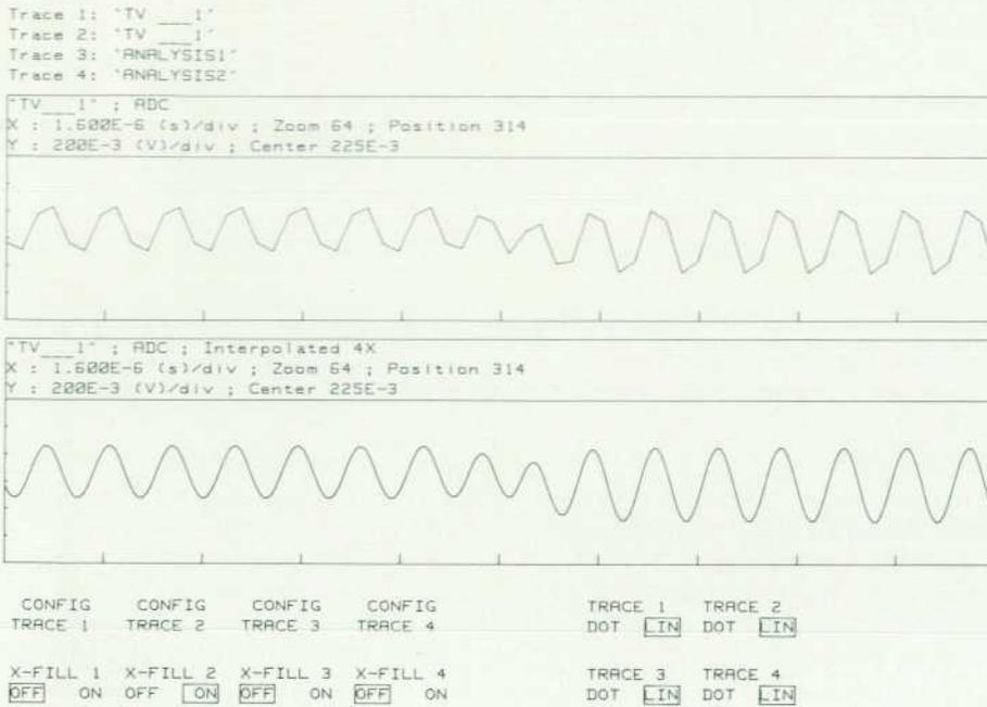
Fig. 9. Detail view of color burst signal.
