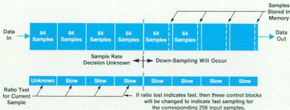
Fig. 3. Adaptive sample rate FIFO buffer operation.
