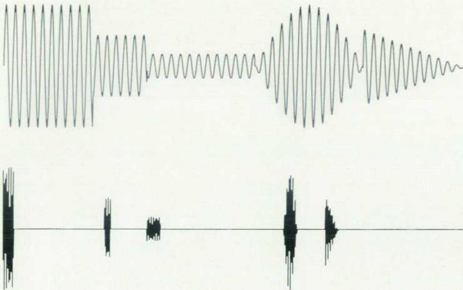
**Fig. 8.** Burst time base mode is used to record a selectable number of samples after a trigger and then stop, rearm, and begin recording again after another trigger. Memory is conserved because no samples are recorded during uninteresting periods between bursts. Recorded signal (top) for input signal (bottom).
