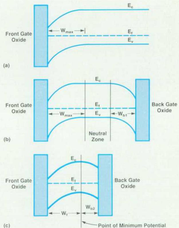
**Fig. 5.** Band diagram for n-channel transistors under inversion. (a) Bulk device. (b) Thick SOI device. (c) Thin SOI device.  $W_{max}$  is the maximum depletion depth.  $W_l$ ,  $W_{b1}$ , and  $W_{b2}$  are the depletion depths related to the front gate, the back gate in a partially depleted film, and the back gate in a fully depleted film, respectively. The following relationships apply:  $W_{max} > W_l$  and  $W_{b1} > W_{b2}$ .
