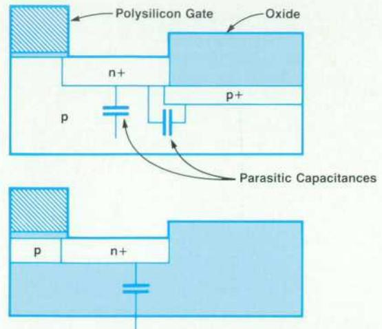
**Fig. 3.** Drain-to-bulk and drain-to-field-implant capacitances in a bulk transistor (top). In an SOI device (bottom), the drain-to-substrate capacitance is reduced because of the insulating oxide underneath the device.
