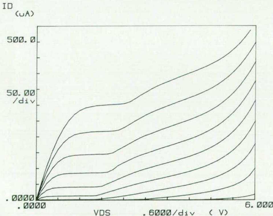
**Fig. 8.** Output characteristics of an n-channel MOSFET made in a 100-nm-thick SOI film. The back-side gate bias is set to -20V to accumulate the bottom of the silicon film and create a floating substrate in the device channel region. Gate voltage ranges from 0 to 2.5V in 0.25V steps.
