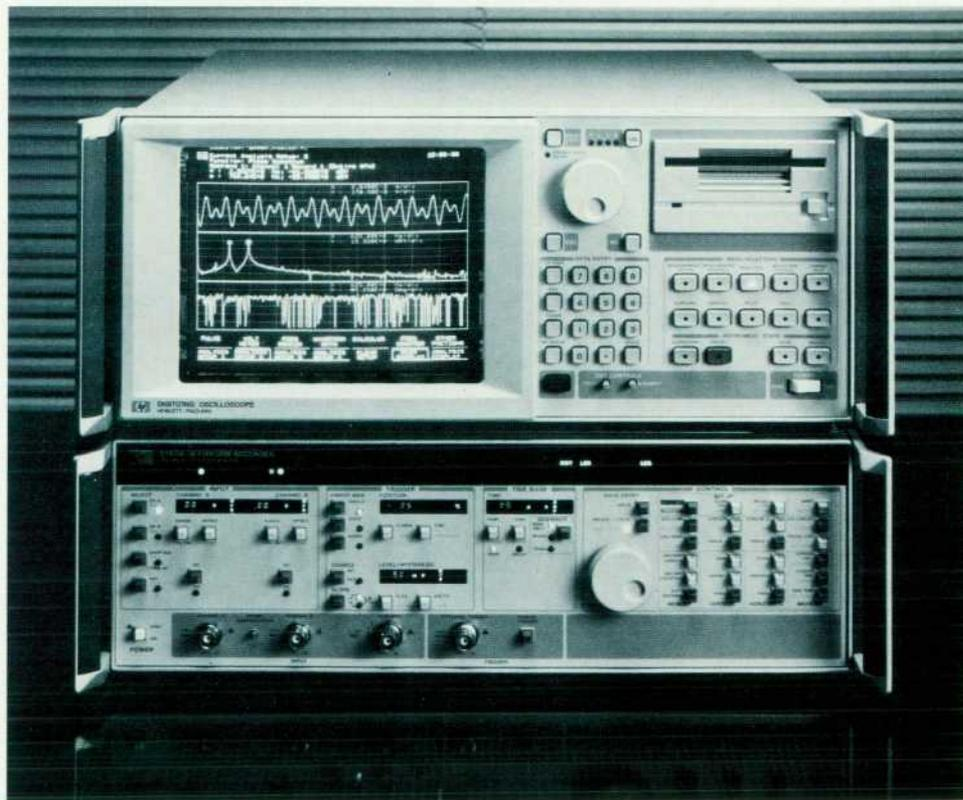
**Fig. 1.** The HP 5180T Precision Digitizing Oscilloscope consists of an HP 5180A Waveform Recorder and an analysis, display, and I/O section. The HP 5180A provides 20-MHz, 10-bit analog-to-digital conversion.
