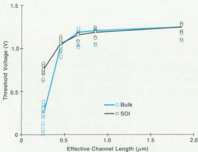
**Fig. 11.** Measured threshold voltages in bulk and SOI *n*-channel MOSFETs as a function of effective channel length. The devices were made in the same lot and received the same threshold implants. The SOI devices were made in a 200-nm-thick SOI film.
