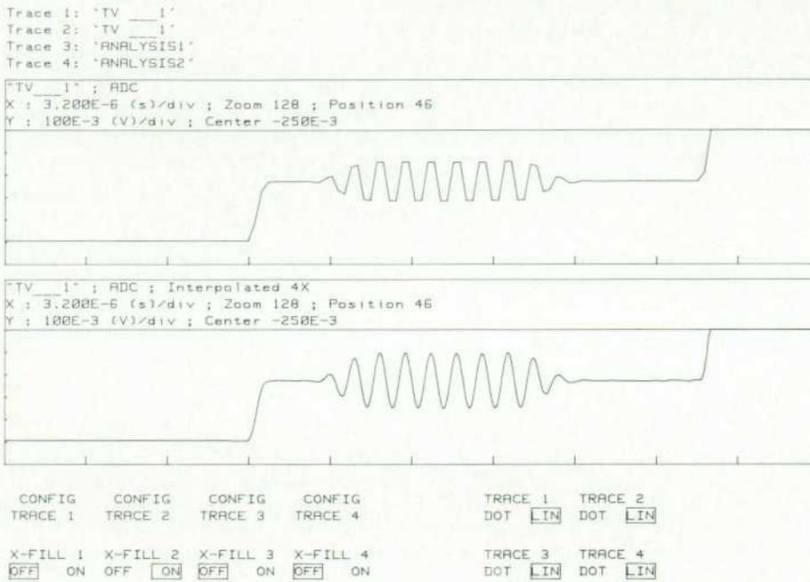
**Fig. 7.** Video sync portion of a single television scan line sampled at four times the color burst frequency without and with reconstruction.
