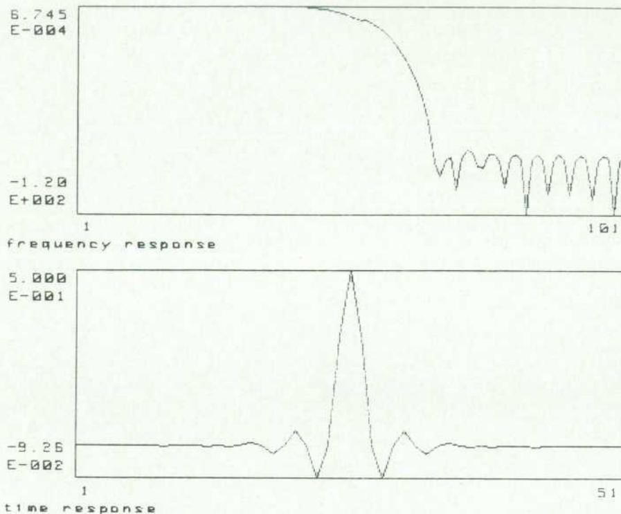
**Fig. 13.** Response of the digital filter used to increase effective bits for low-frequency signals by removing high-frequency quantization noise.
