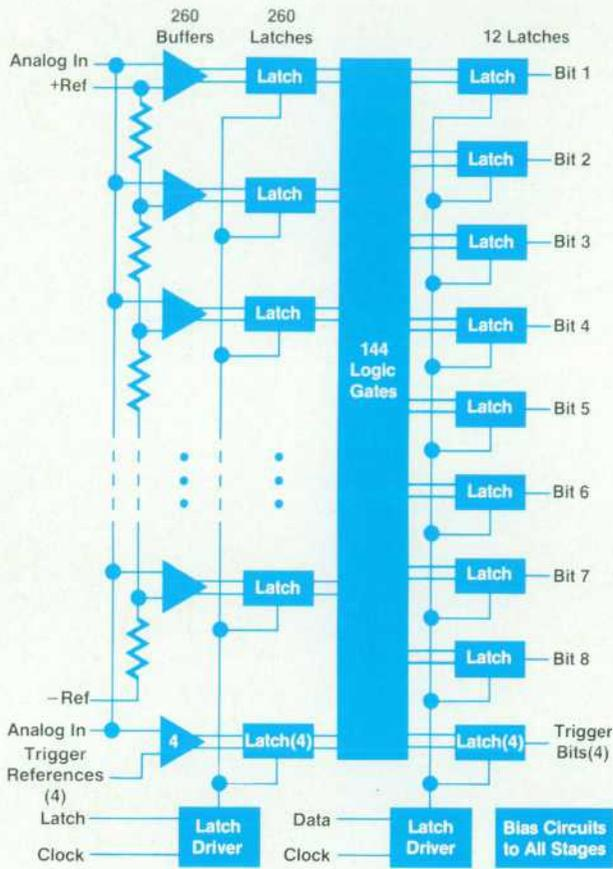
Fig. 2. 8-bit quantizer IC block diagram.
