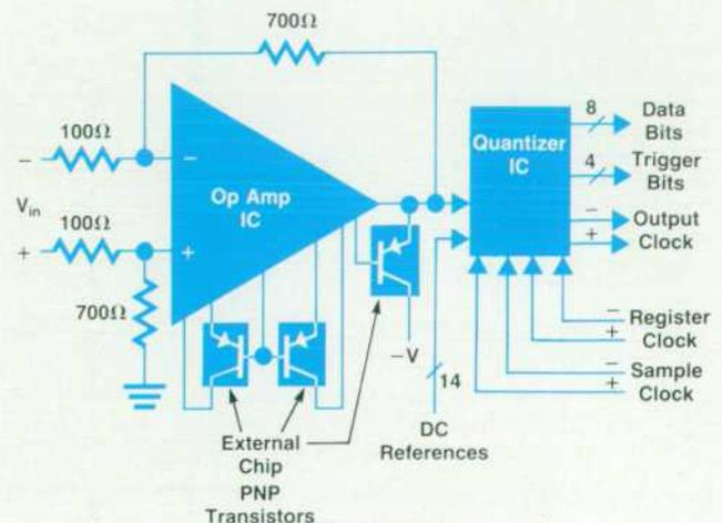
**Fig. 1.** ADC hybrid block diagram. The electrical and thermal requirements of the hybrid packaging scheme revolve around the quantizer IC.
