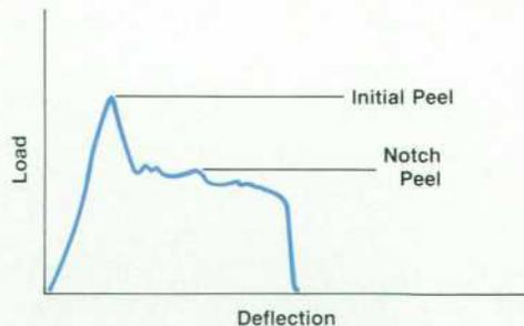
Fig. 7. Typical data from a peel test.
