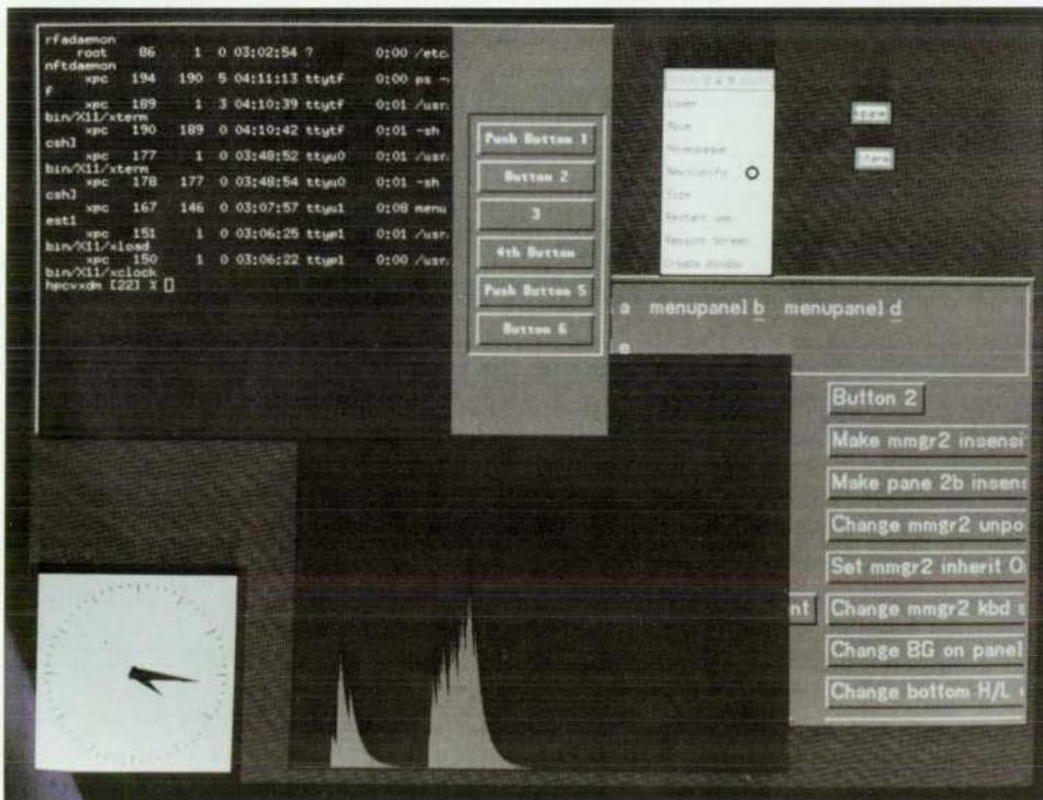
Fig. 3. Final screen for the scenario presented in the text. The Launch menu and the menu containing the iconify command are pop-up menus; they are called up by clicking the proper mouse button and go away after a selection is made. The two icons for the terminal emulator and electronic mail applications are in the upper right corner.
