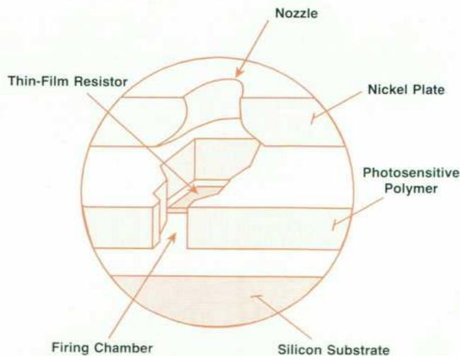
Fig. 2. Cross section of an inkjet nozzle.
