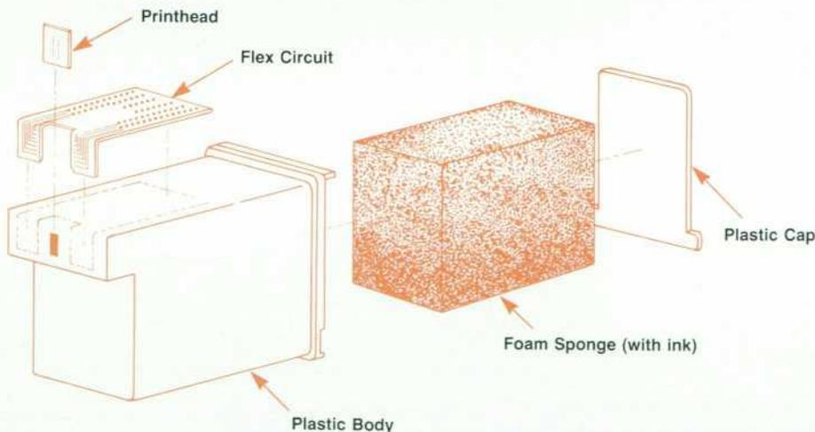
Fig. 9. Exploded view of the DeskJet print cartridge.
