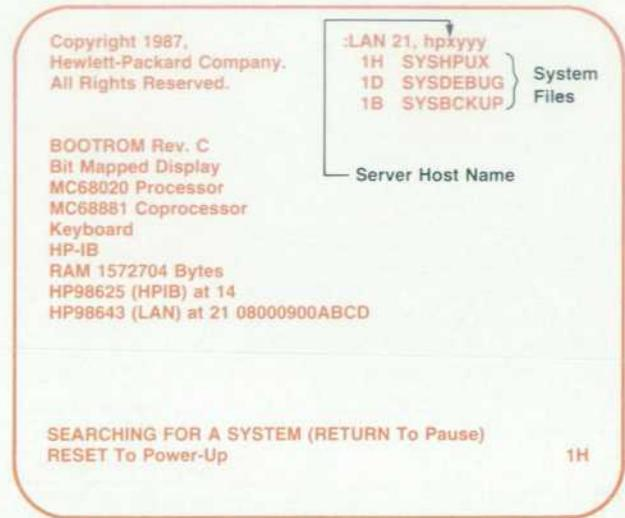
Fig. 2. A typical screen the user sees during the boot process.
