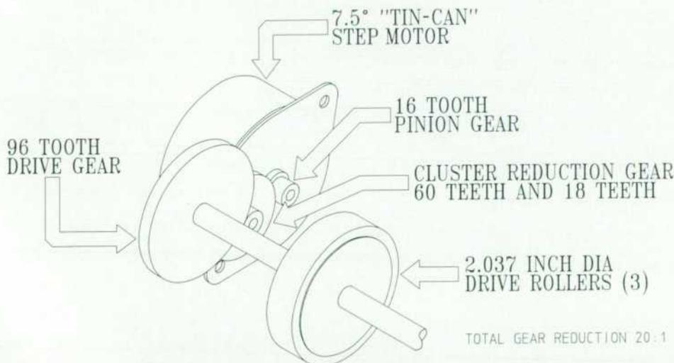
Fig. 4. Paper drive motor assembly.
