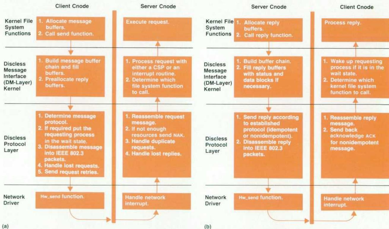
**Fig. 3.** Network control flow. (a) Originating a request from the client and receiving a request at the server. (b) Sending a reply from the server and receiving a reply at the client. CSP = cluster server process.
