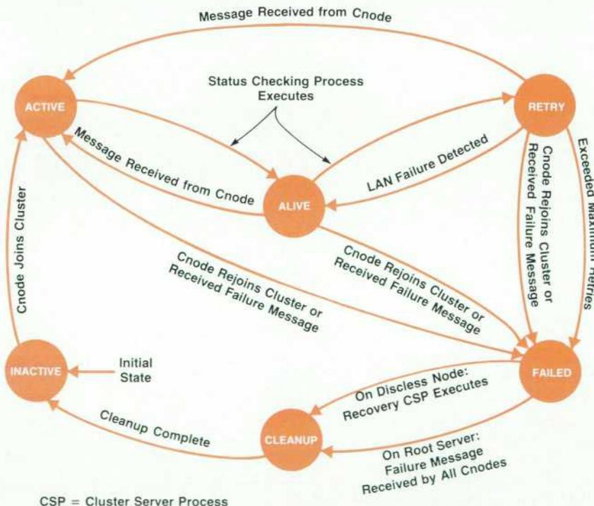
Fig. 1. States of crash detection and recovery.
