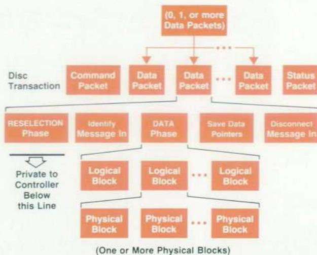
**Fig. 3.** Data packets for a typical disc transaction on the SCSI bus. The Command packet contains the information for setting up the environment for data transfer. Information such as the Identify and the Synchronous messages are contained in this packet.
