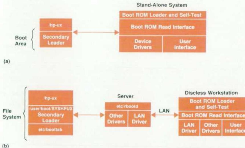
Fig. 1. (a) The major components involved in the boot process for a stand-alone HP-UX system. (b) The major components involved in the boot process in a discless environment.
