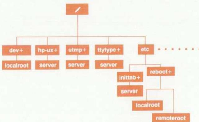
Fig. 2. Partial system model for the server cnode. "Server" is the cnode name given to the root server.
