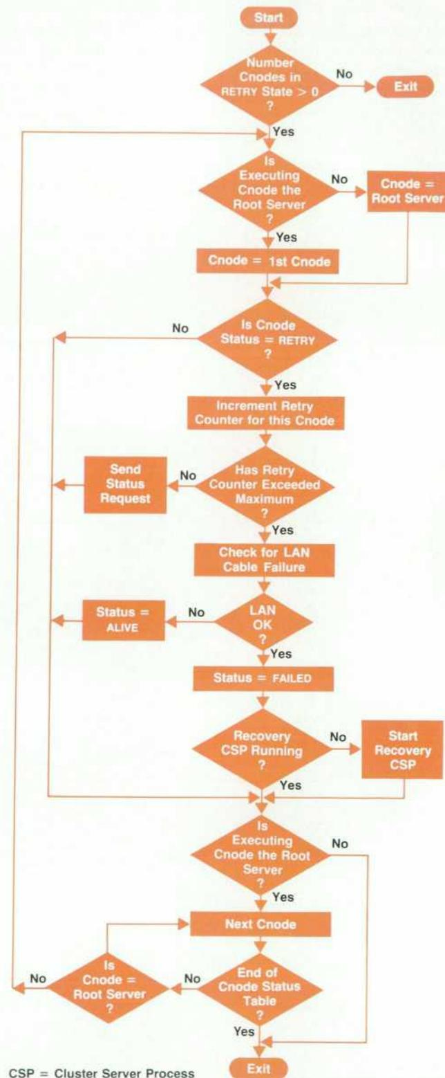
Fig. 3. Crash detection: retry status request process.
