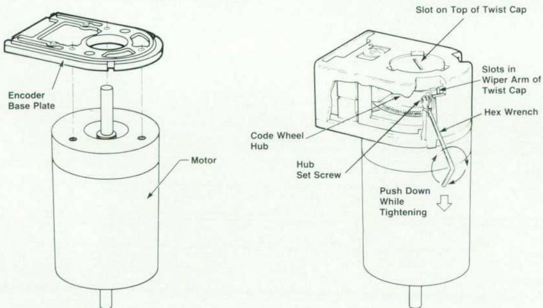
Fig. 1. To attach the HEDS-5500 encoder to a motor, a baseplate is attached to the motor with screws and the encoder is snap mounted to the baseplate. The encoder housing contains a code wheel and an HEDS-9000 encoder module.
