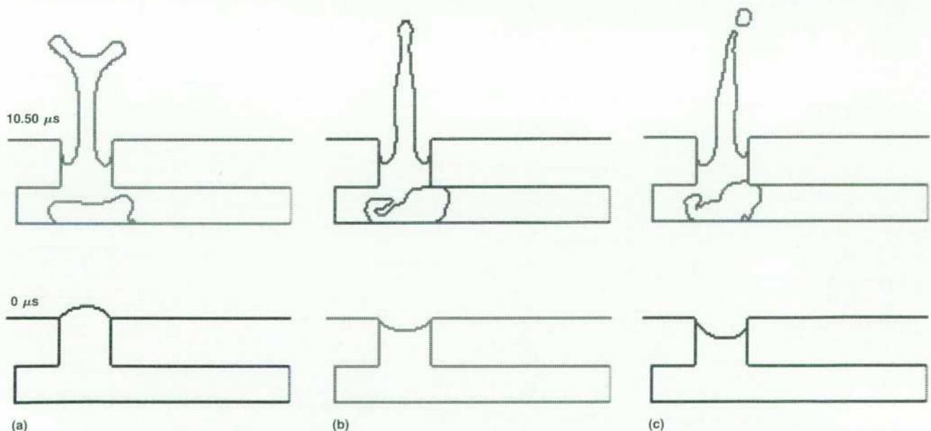
**Fig. 3.** Effects of the meniscus configuration on the ejected drop. (a) A bulging meniscus adds to the volume of the drop. (b) A retracted meniscus reduces the volume of the drop. (c) Fluid acceleration during bubble growth causes emerging drops to pull off-axis or flare out as in (a).
