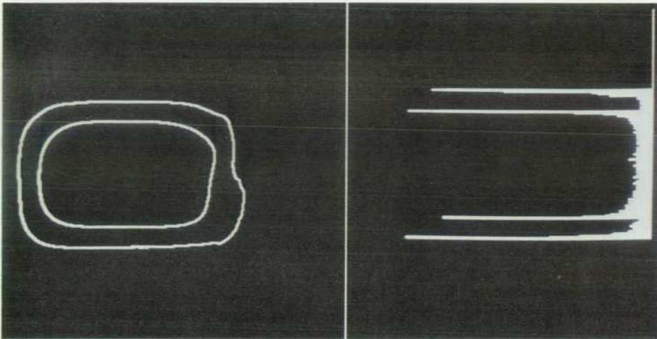
**Fig. 4.** Edge-enhanced adhesive image and horizontal profile.
