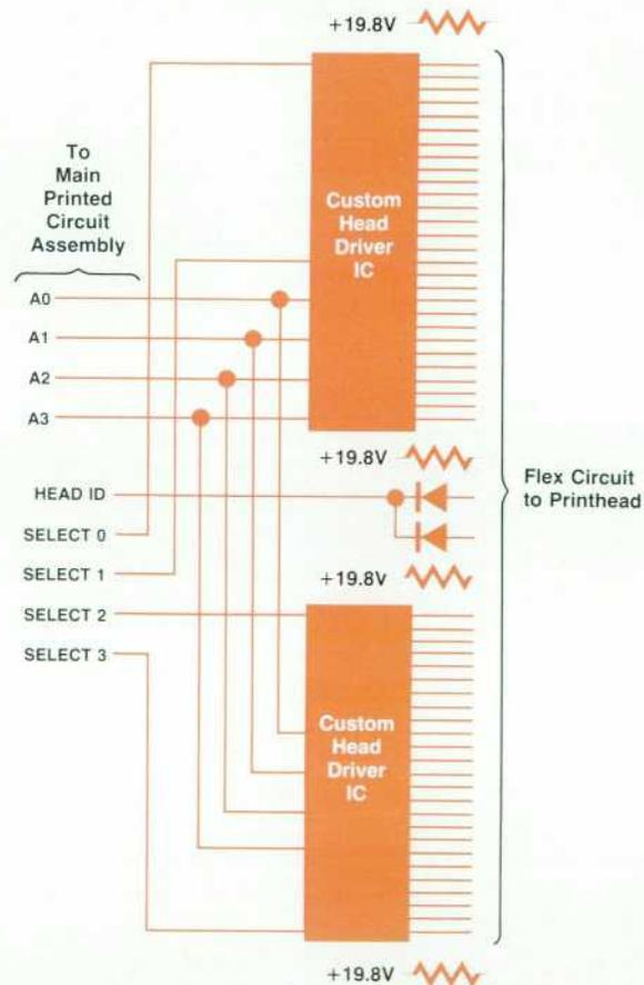
Fig. 1. Two custom ICs on a carriage-mounted printed circuit board drive the DeskJet printhead.
