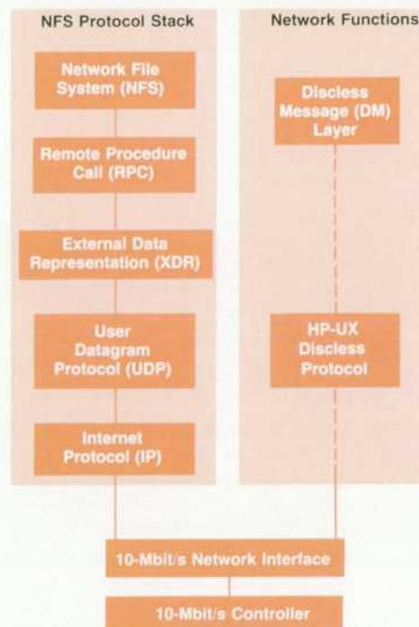
Fig. 2. NFS protocol stack versus HP-UX network functions.
