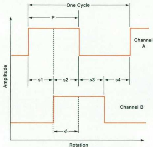
**Fig. 1.** Typical output waveforms for a two-channel quadrature encoder. One shaft rotation equals 360 mechanical degrees or  $n$  cycles, where  $n$  is the number of counts per revolution. Each count (cycle) corresponds to one code wheel spoke and window pair. One cycle equals 360 electrical degrees.
