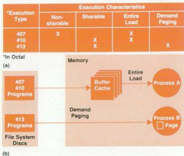
Fig. 1. (a) Standard HP-UX program types and their execution characteristics. (b) Loading behavior of the different program types.
