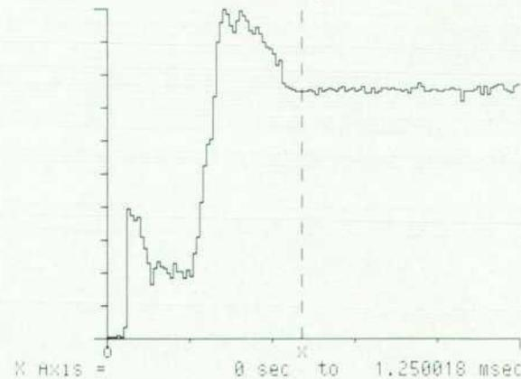
Fig. 11. The step response of a VCO is shown by a time variation plot.
