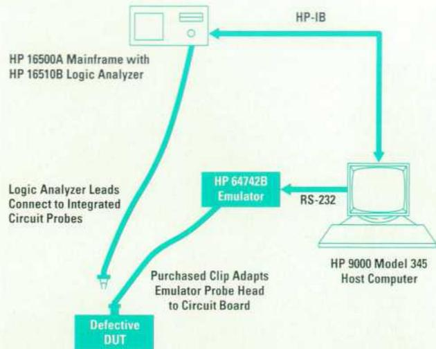
Fig. 1. System used in HP 54600 Series oscilloscope production to troubleshoot defective digital boards.
