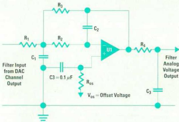
$$\text{Gain} = \frac{R_3}{R_1}$$
