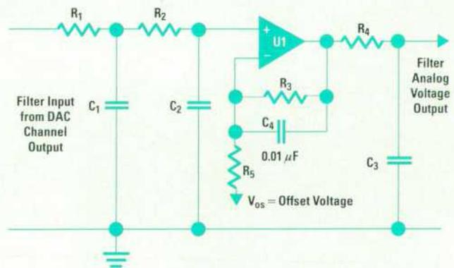
$$\text{Gain} = 1 + \frac{R_3}{R_5}$$
