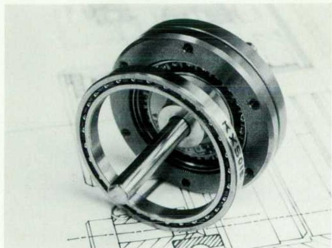
Fig. 5. Harmonic drive reduction unit.
