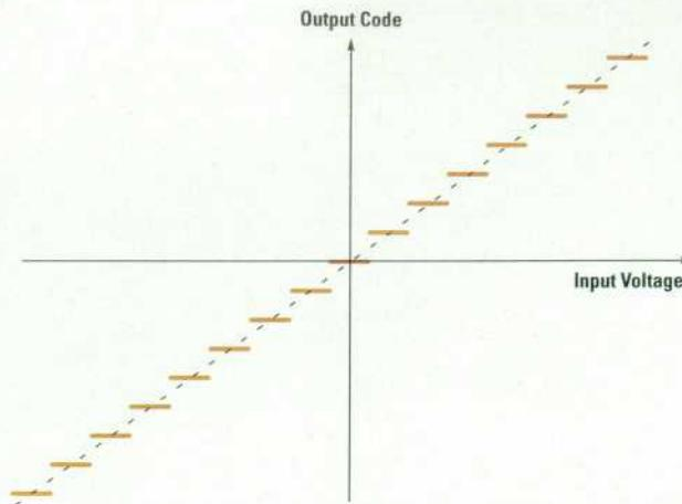
**Fig. 7.** Ideal quantizer transfer function.
