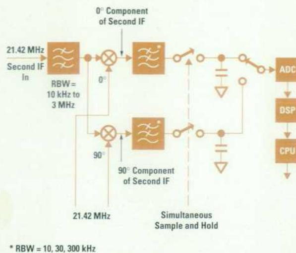
**Fig. 7.** Components involved in providing the dc sampling mode for spectrum analysis with wider RBWs. The in-phase and quadrature components are captured by the sample-and-hold circuits at the same time. The DSP chip calculates the power.
