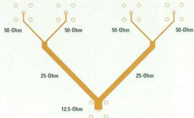
**Fig. 14.** The sample clock is distributed symmetrically to the four acquisition hybrids on transmission lines that transition from 50 ohms at the hybrids to 25 ohms and then to 12.5 ohms at the oscillator.
