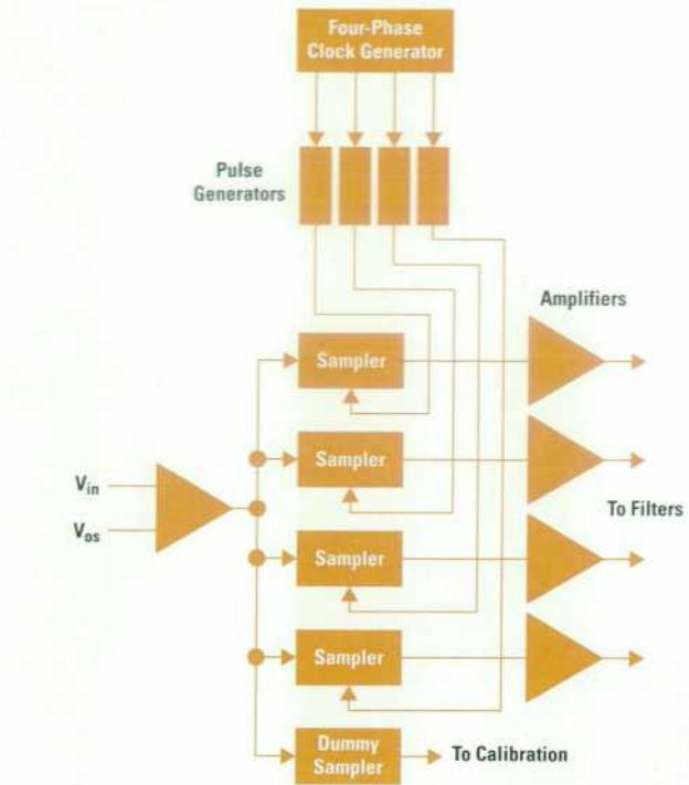
**Fig. 14.** Sampler channels with dummy sampler for calibration of gain and bandwidth.
