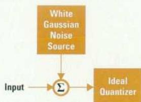
**Fig. 9.** Adding noise to randomize quantizing error.
