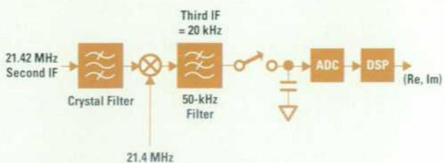
**Fig. 9.** Components involved in providing the ac sampling mode for network analysis. The 20-kHz IF is sampled and held at 80 kHz. The vector information is generated by the DSP chip, and the CPU receives the real and imaginary components of the IF signal.
