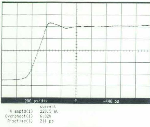
**Fig. 22.** Step response of an 8-GSa/s HP 54720 system.
