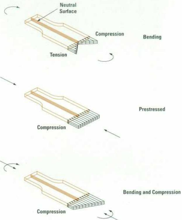
Fig. 8. Prestressing prevents tensile loads on the ceramic substrate.
