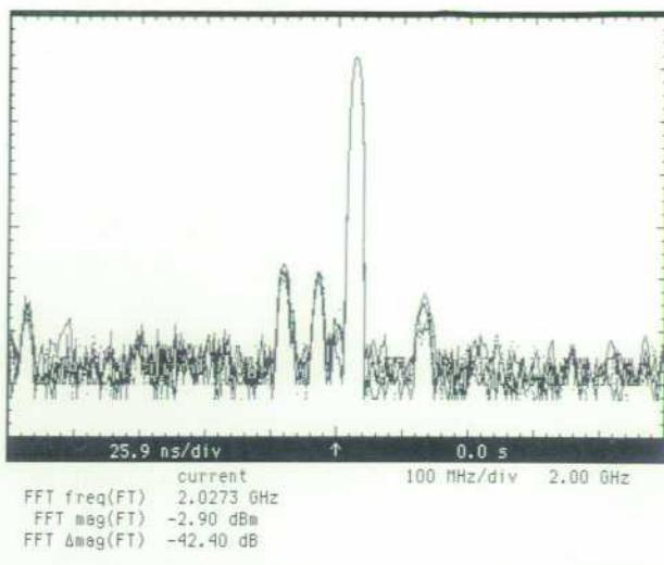
**Fig. 24.** FFT of the 2-GHz reconstructed sine wave of Fig. 20, showing sidebands down 42 dB from the fundamental.
