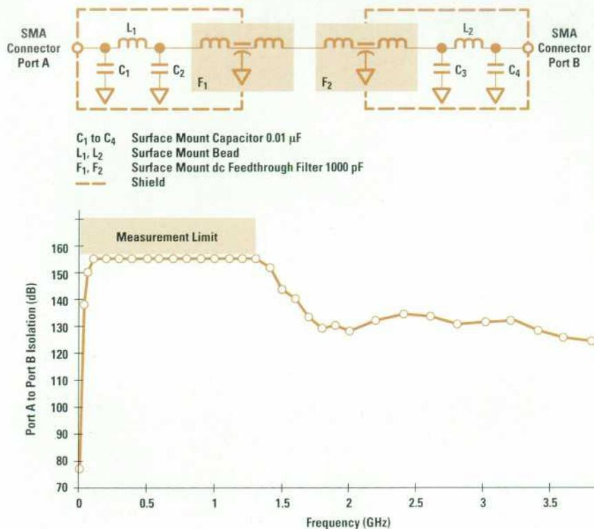
**Fig. 14.** Shield effectiveness of the RF structure using surface mount feedthrough filters.
