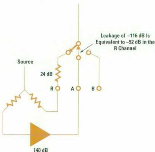
**Fig. 9.** Measurement of a high-gain amplifier (140 dB). The leakage through the A channel is 48 dB larger than the desired R-channel signal. Thus, the amplifier cannot be measured correctly because of the extra pad at the R channel.
