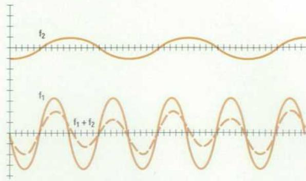
**Fig. 12.** Subharmonics are much more important than harmonics because they can cause periodic shifts in the sample positions.
