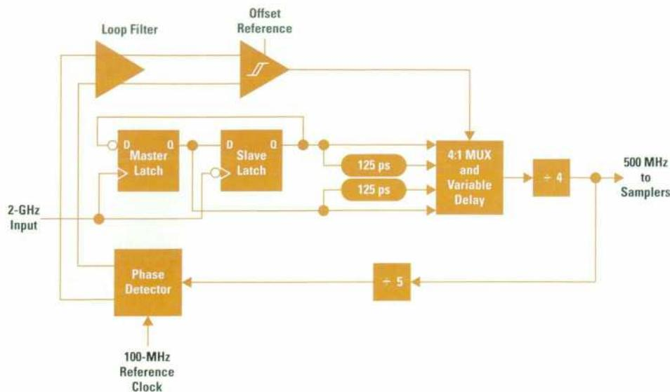
**Fig. 20.** Delay-locked loop schematic diagram.
