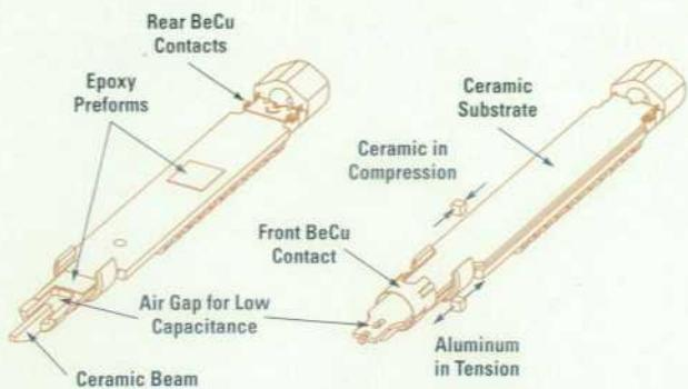
Fig. 9. Method of prestressing the substrate using epoxy.
