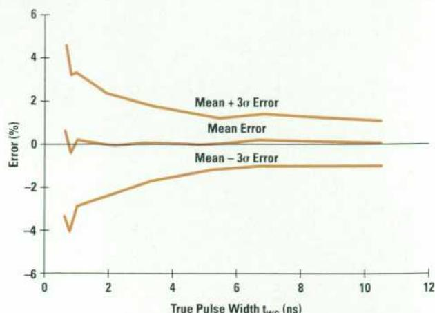
**Fig. 4.** HP 54720A bias-corrected impulse width error at 4 GSa/s. Bias correction equations using exponential terms can correct the HP 54720A's Gaussian pulse mean measurement accuracy to better than 0.5% and  $3\sigma$  accuracy to better than 4% for most pulses.
