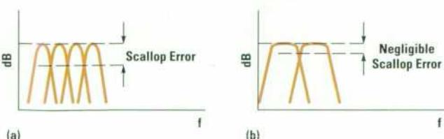
**Fig. 3.** A subtle side effect of using the Hamming window function is that if a component of the input signal is not centered in the filter's shape, a portion of the signal's amplitude will be attenuated. (a) Hamming passband filter shapes and the scallop error. (b) Using a window function with a flatter (flat-top) passband reduces the scallop error.
