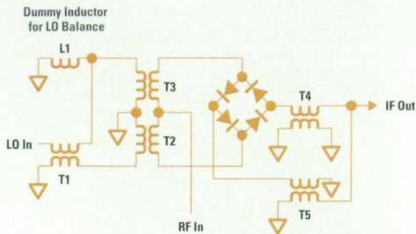
**Fig. 3.** Schematic diagram of the first mixer.
