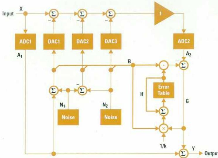
Fig. 14. DAC calibrator block diagram.
