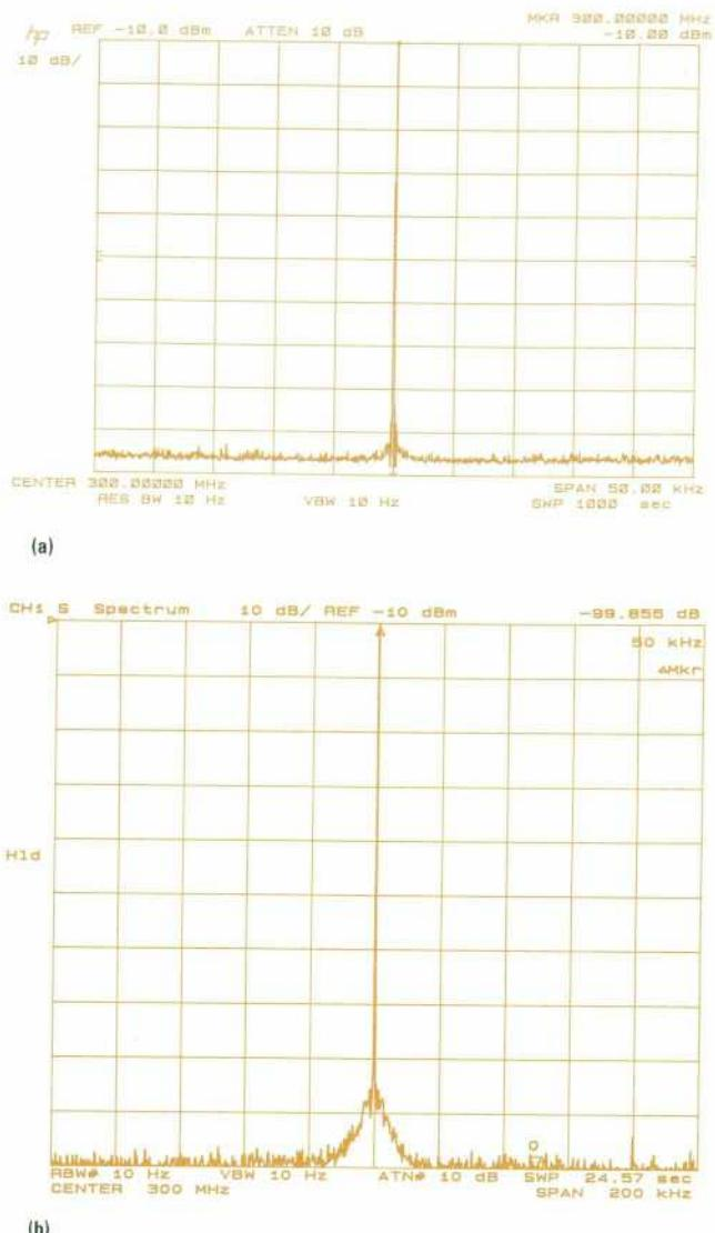
**Fig. 12.** The difference in scale fidelity between the HP 4396A and a conventional spectrum analyzer. (a) A dc offset of the rectifier is seen at about  $-95$  dB in a conventional logarithmic-based spectrum analyzer's display. (b) No dc floor is seen in the display of the HP 4396A.
