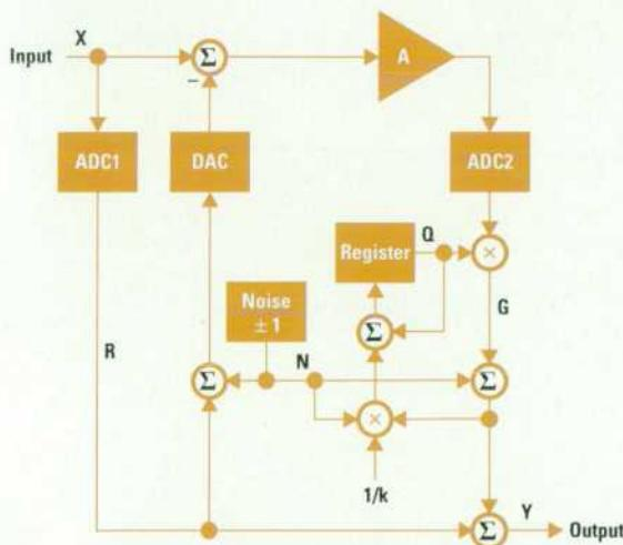
Fig. 12. Residue gain calibrator block diagram.
