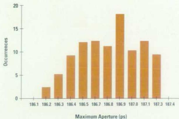
Fig. 6. Sample maximum aperture measurement repeatability histogram.
