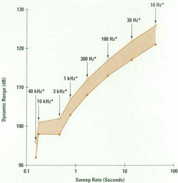
**Fig. 4.** The dynamic range of the network measurement mode is plotted as a function of the sweep rate and the IF bandwidth using 201 measurement points.
