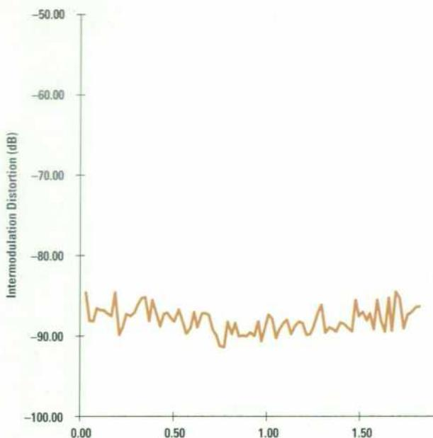
Fig. 13. Frequency response of the HP4396A's third-order IMD.
