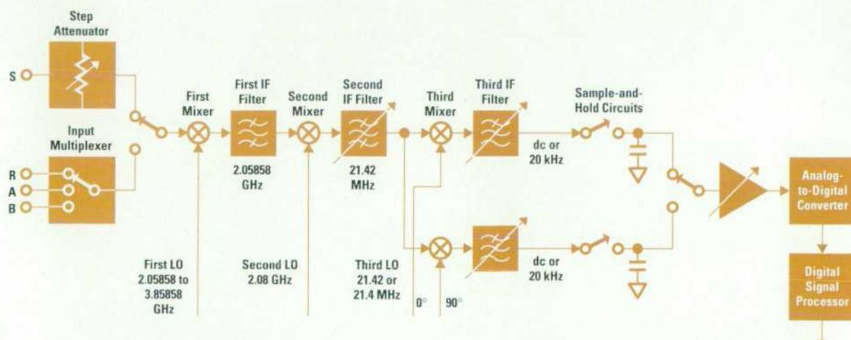
Fig. 1. Block diagram of the receiver for the HP4396A vector network and spectrum analyzer.
