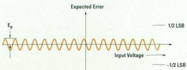
**Fig. 10.** Adding noise to reduce nonlinearity error.
