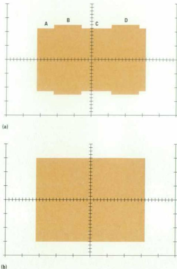
**Fig. 15.** Effect of HFADJ input on bandwidth matching, (a) without and (b) with calibration.
