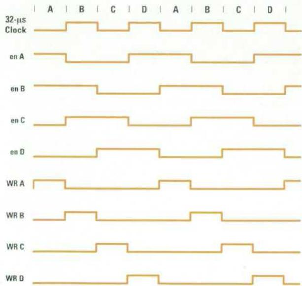
**Fig. 19.** (a) FISO memory write control schematic. (b) Timing diagram for chaining acquisition memory.
