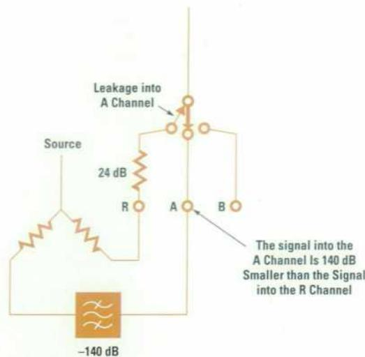
**Fig. 8.** An extra pad at the R channel makes 140-dB filter measurement possible.
