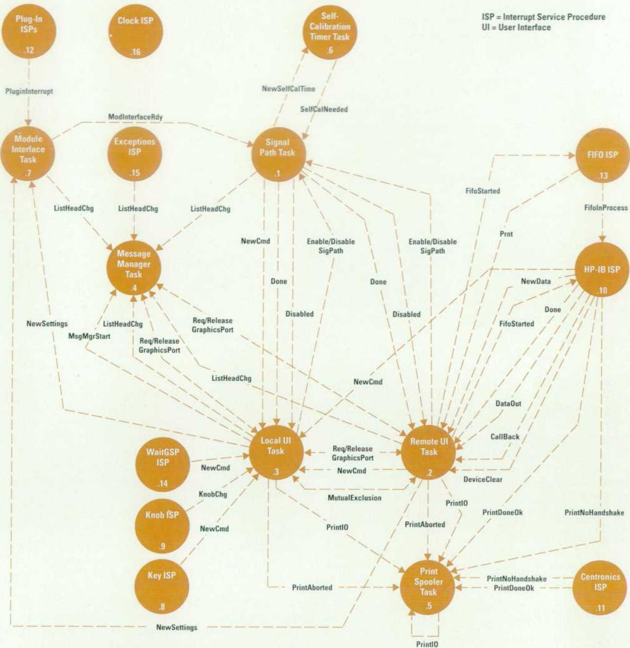
**Fig. 4.** Host processor tasks in the HP 54720/10 oscilloscope.
