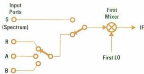
**Fig. 3.** Input multiplexer design to provide network and spectrum analysis in the HP 4396A.
