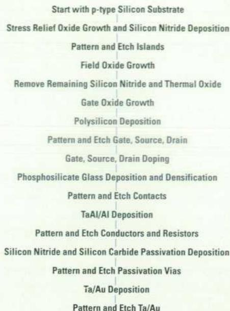
Fig. 5. Integrated driver printhead process flow.
