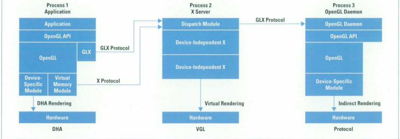
coupled with two distinct remote rendering modes, making our OpenGL implementation one of the most flexible implementations in the industry. These rendering modes are based upon the three-process rendering model shown in **Figure 6**. This model supports three rendering modes: direct, indirect, and virtual.
