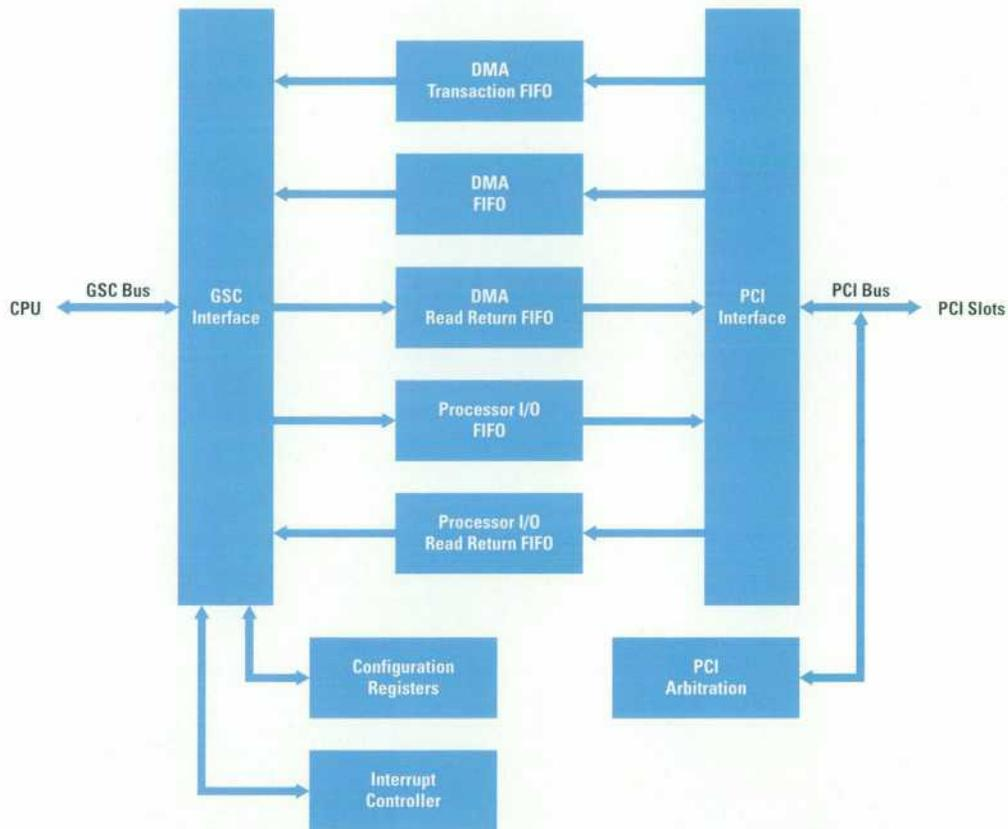
A FIFO is a memory device that has a port for writing data into the FIFO and a separate port for reading data out of the FIFO. Data is read from the FIFO in the same order that it was written into the FIFO. The GSC bus clock is asynchronous to the PCI bus clock. For this reason, the FIFOs need to be asynchronous. An asynchronous FIFO allows the data to be written into the FIFO with a clock that is asynchronous to the clock used to read data from the FIFO.
