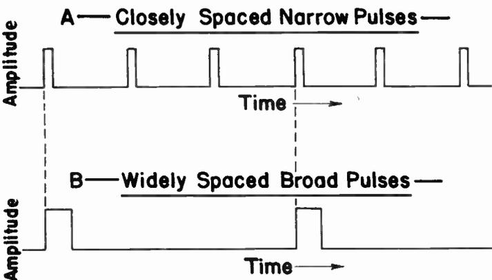
Fig. 10. Recurrent Pulses Representing Vertical Objects in the Picture.
