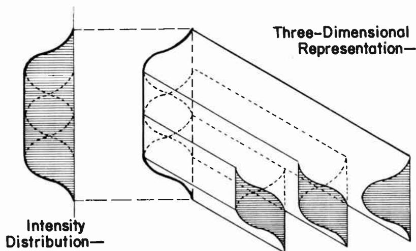
Fig. 2. Flat Field Obtained By Scanning With Cathode-Ray Spot.
