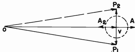
Fig. 13. Amplitude and Phase Distortion Components Superimposed on a Signal Component
