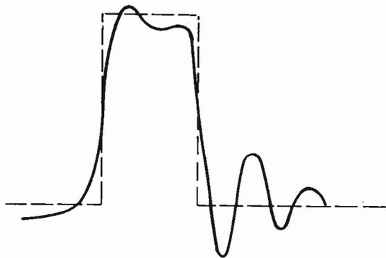
Fig. 12. The Effect of Both Sharp Cutoff and Phase Distortion on a Fairly Narrow Pulse.
