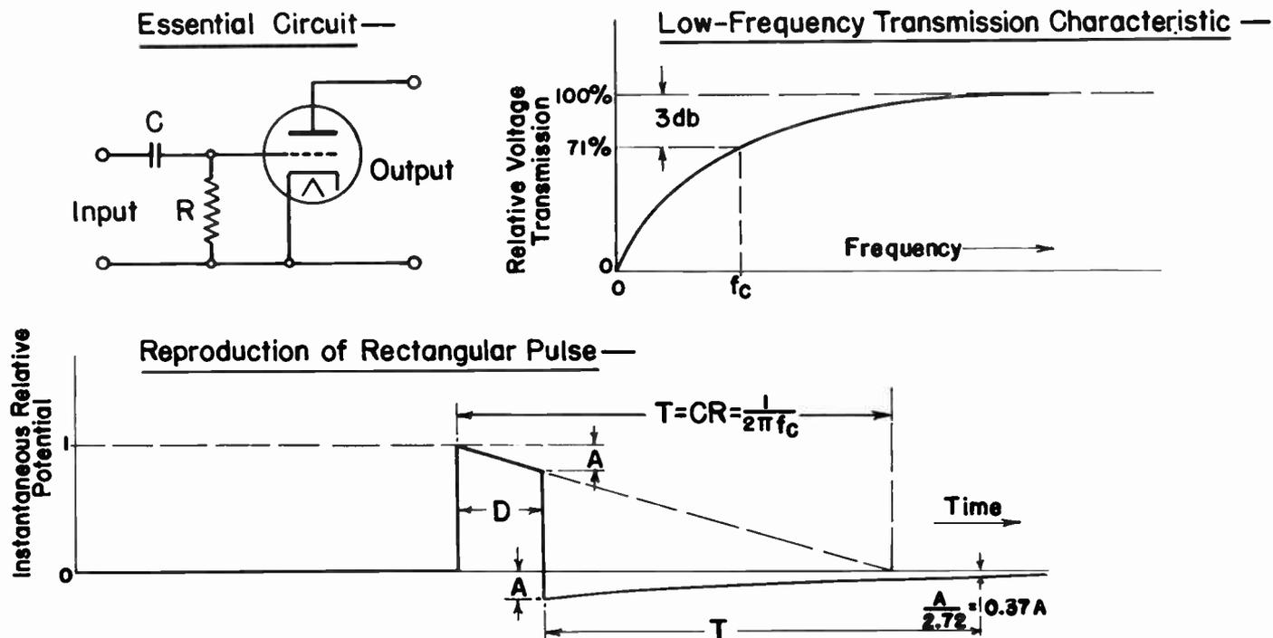
Fig. 14. Distortion of Pulse Caused Mainly by Phase Shift of Low-Frequency Components.
