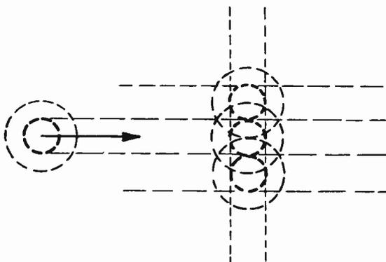
Fig. 5. Demonstration That the Minimum Width of Reproduction of a Vertical Line is Equal to the Pitch of the Scanning Lines.
