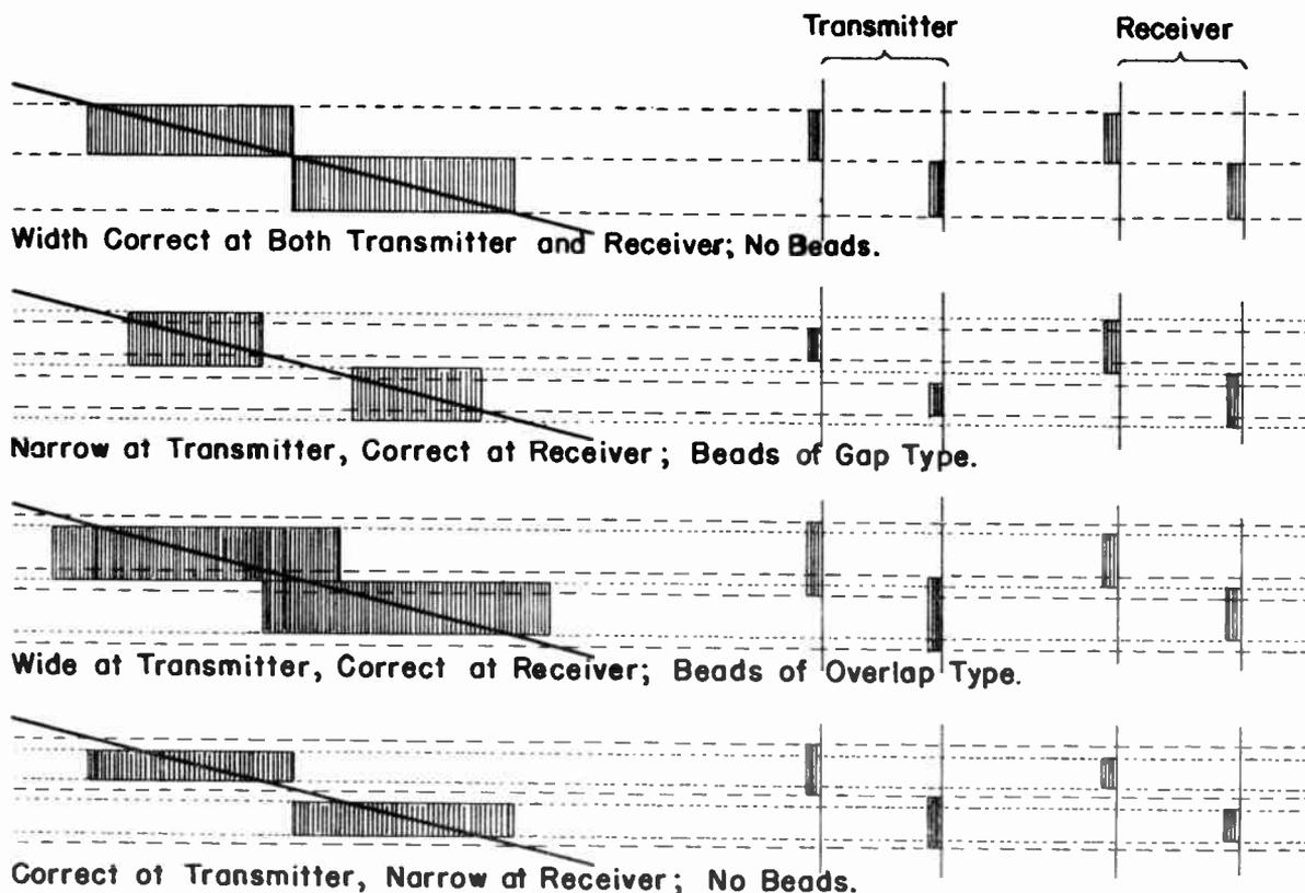
Fig. 3. The Production of Beads by Improper Width of Scanning [Wikipedia History](#) in the Transmitter.
