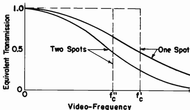
Fig. 7. Frequency Characteristics of the Transmitter Scanning Spot Alone, and of Both Transmitter and Receiver Spots Together.
