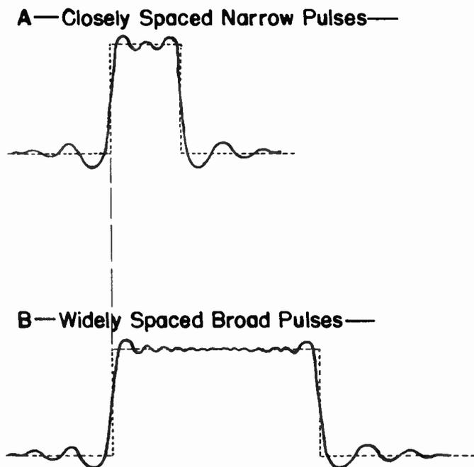
Fig. 11. The Effect of Cutting Off the Higher-Frequency Components of the Pulses of Fig. 10.
