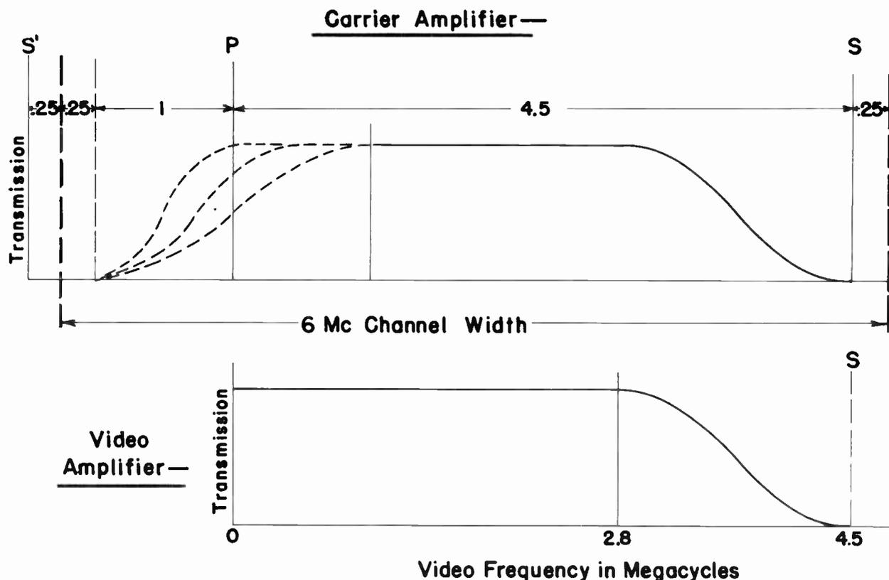
Fig. 8. Amplitude Characteristics of the Carrier-Frequency and Video-Frequency Amplifiers of the Receiver.
