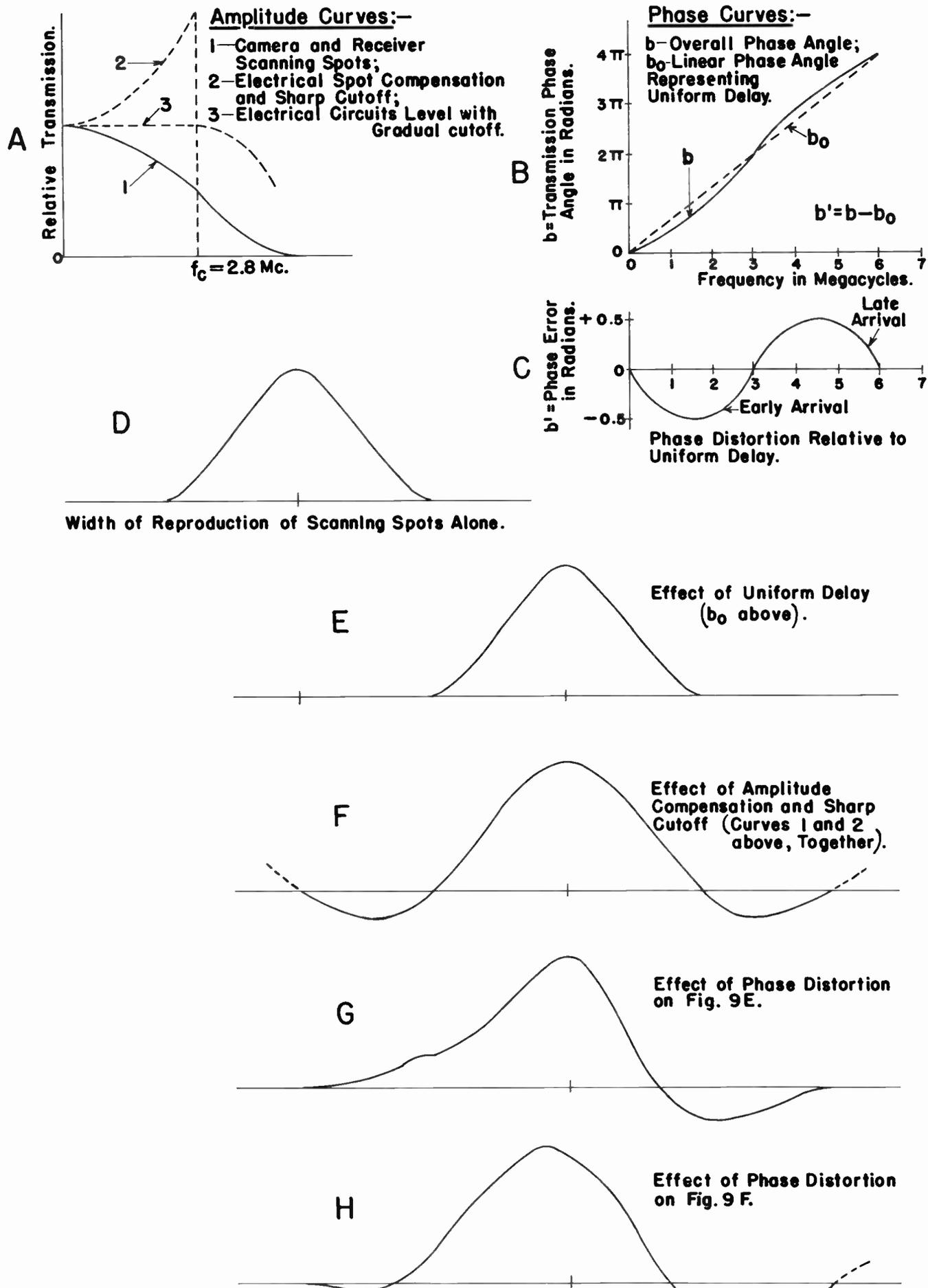
Fig. 9. Amplitude and Phase Effects in Reproduction of a Narrow Vertical Line.
