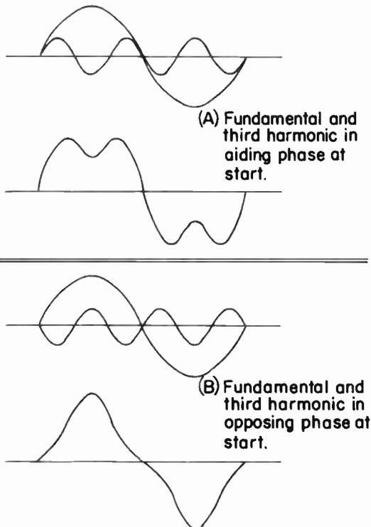
Fig. 7. Dependence of Wave Form on Phases of Components
