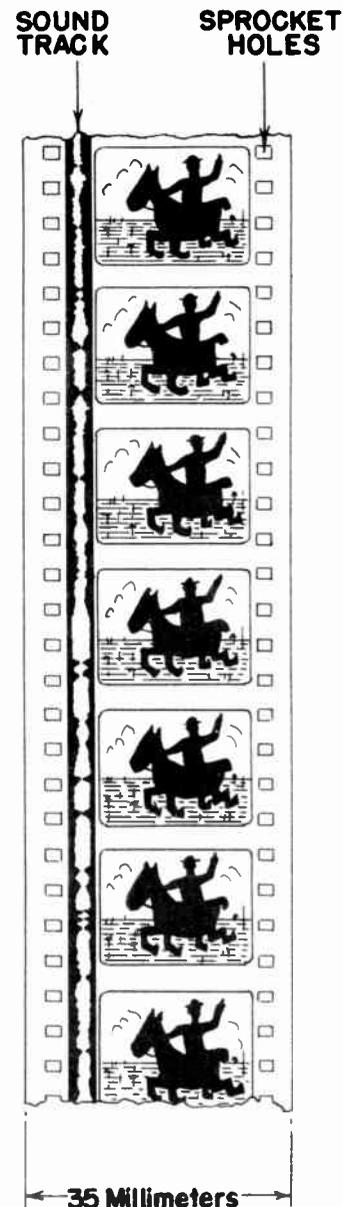
Fig. 8. Motion-Picture Film.
