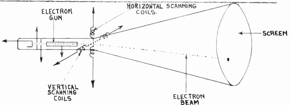
(C) PICTURE TUBE WITH MAGNETIC SCANNING.
