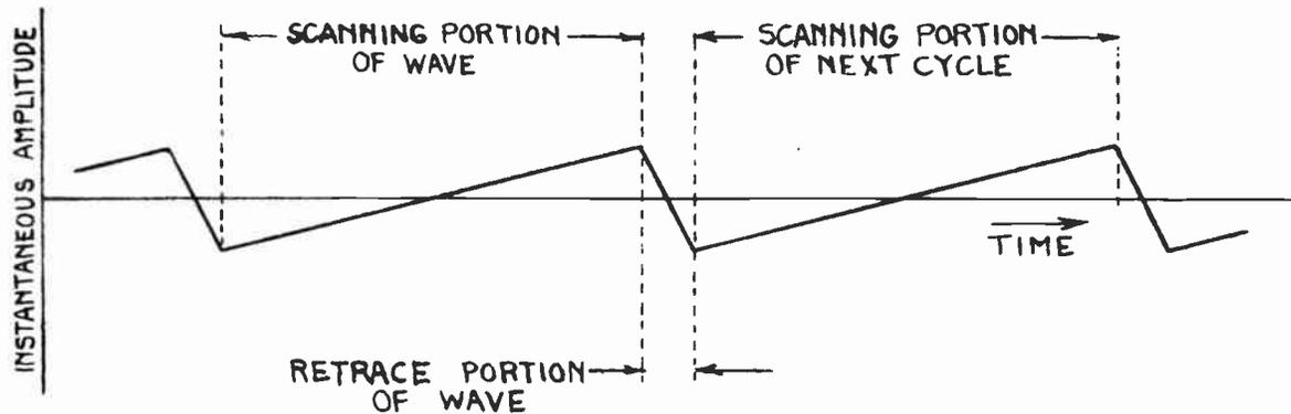
Fig. 6. Saw-Tooth Wave Form.
