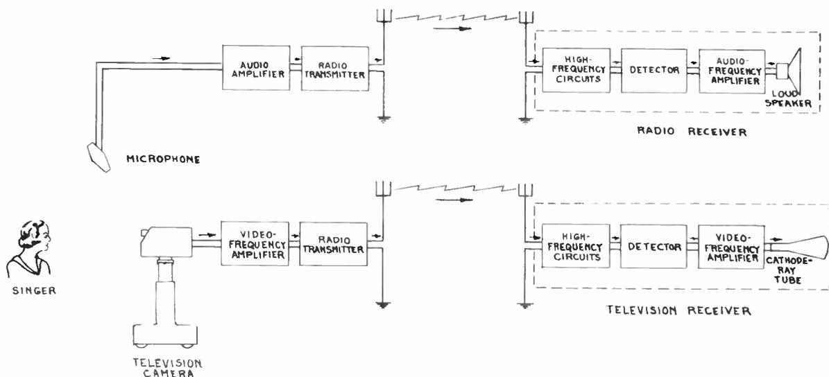
Fig. 1. Sound Radio System Compared With Television System.
