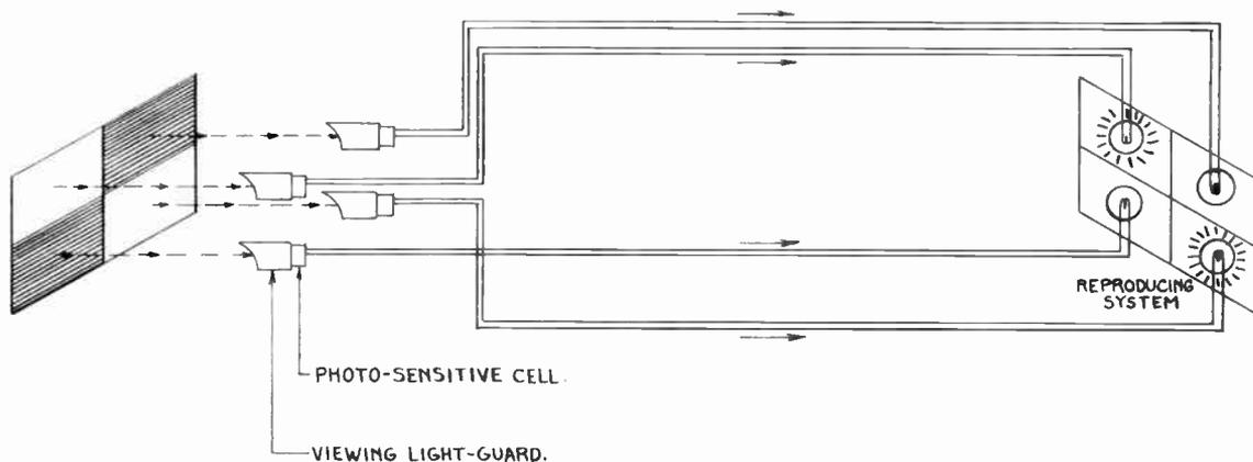
Fig. 2. Multi-Channel Transmission of Very Simple Changing Picture.
