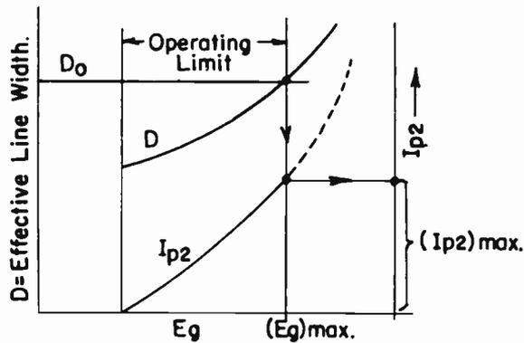
Fig. 21. Determination of Maximum Beam Current According to Spot Size.
