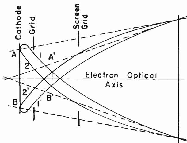
Fig. 17. Electron Paths and Cross-Over in Lens of Figure 16.
