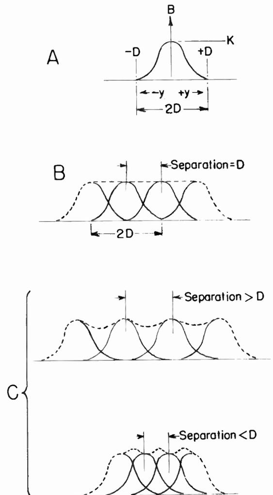
Fig. 5. Uniform or Non-Uniform Brightness Across the Lines According to Spacing in Terms of Effective Line Width.
