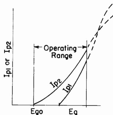
Fig. 20. First-Anode and Second-Anode Currents for Various Grid Potentials.
