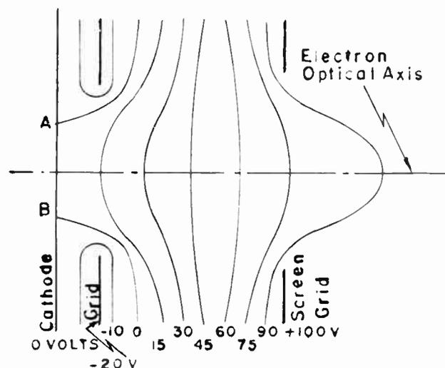
Fig. 16. Equipotential Surfaces at First Lens of Electron Gun.
