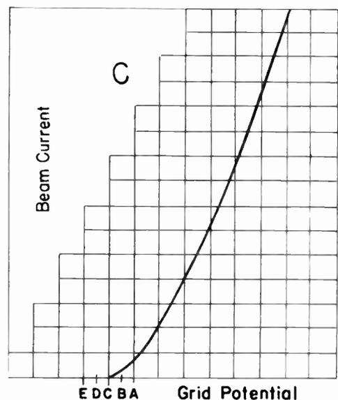
Fig. 10. Effects of Background Light and Improper Bias on Reproduction.
