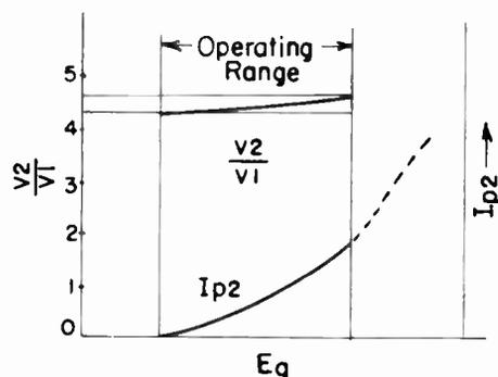
Fig. 18. Second-Lens Voltage Ratio for Perfect Focusing.
