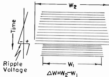
Fig. 13. Effect on Raster of Insufficient Filtering in High-Voltage Supply to Tube.
