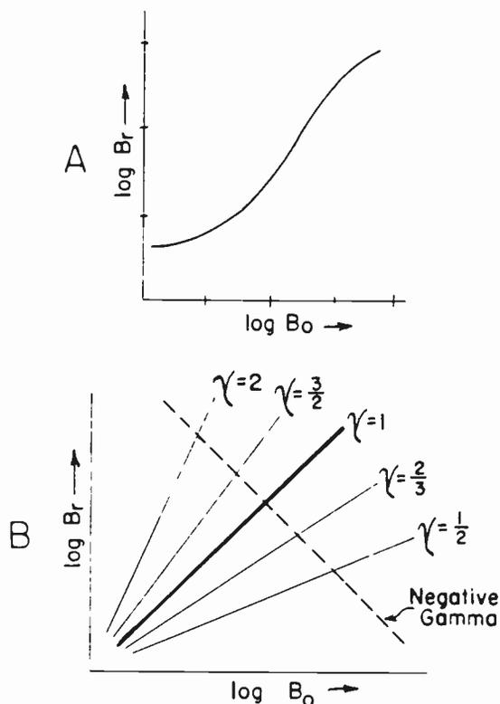
Fig. 9. Curves Relating to the Gamma of a Television System.
