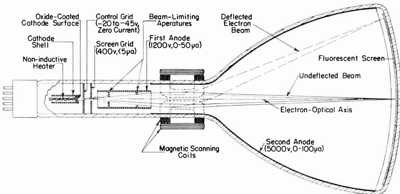
Fig. 1. Cross-Section of Picture Tube with Electric Focusing and Magnetic Scanning, Showing Parts of Electron Gun.
