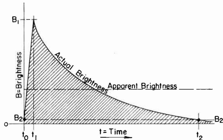
Fig. 7. Instantaneous and Apparent Brightness.
