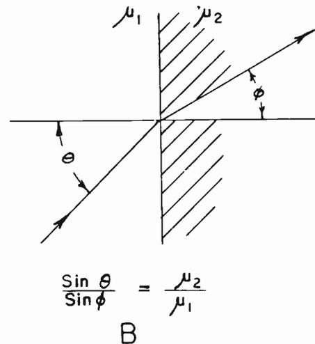
Fig. 14. Analogy Between Electric Double Layer and Passage of Light Ray Thru Interface of Two Media.
