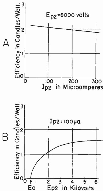
Fig. 8. Efficiency of Screen at Various Beam Currents and Voltages.
