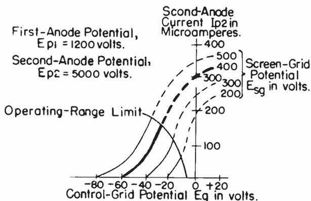
Fig. 3. Second-Anode Current of Picture Tube as Function of Potentials of Control Grid and Screen Grid.
