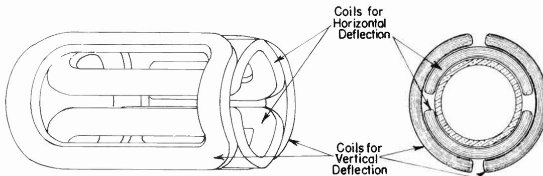
Fig. 2. Arrangement of Scanning Coils Around Neck of Tube.
