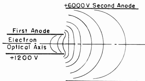
Fig. 19. Arrangement of Second Lens.
