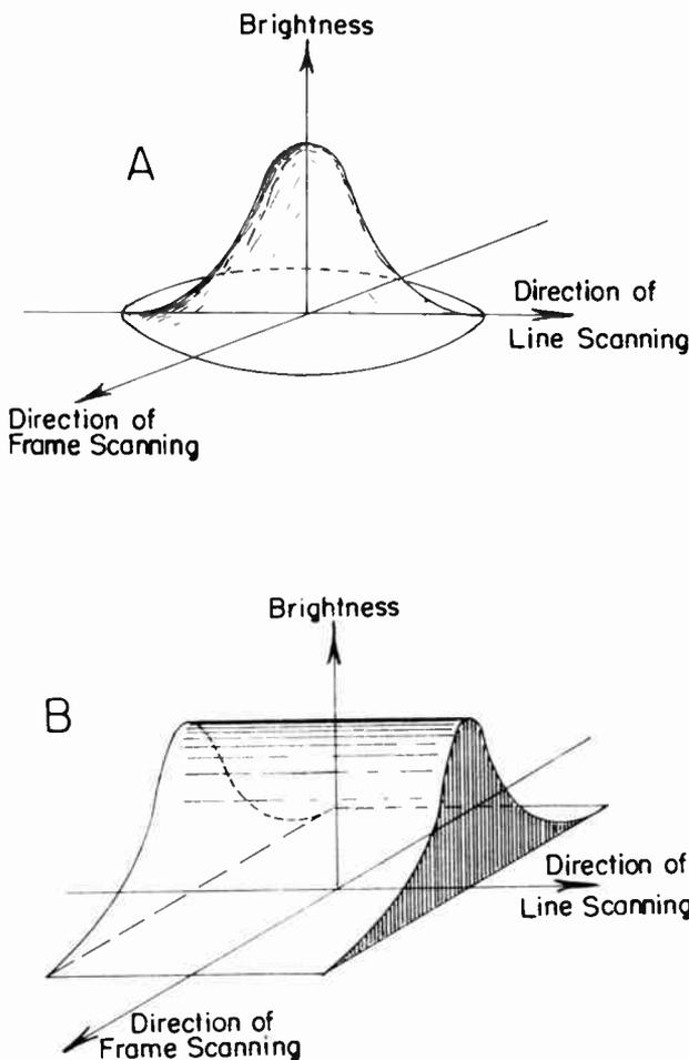
Fig. 4. Brightness Distribution Over Scanning Spot and Line.
