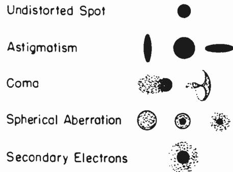
Fig. 11. Distortion of Spot by Faults in Electron Lenses.
