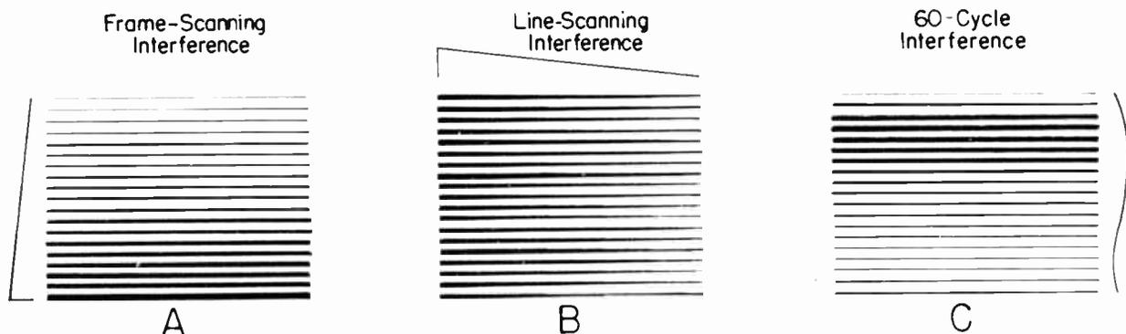
Fig. 12. Effect on Raster of Interference in the Video Channel from Scanning and Power-Supply Circuits.
