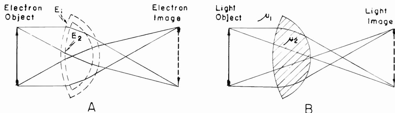
Fig. 15. Hypothetical Electron Lens Made of Double Layers, and the Corresponding Light Analog.
