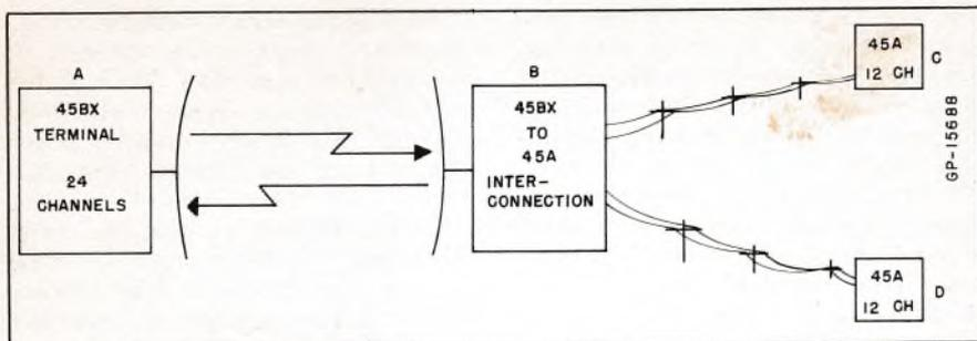
FIGURE 3. Typical interconnection of 45-class carrier equipment. If the network is equipped with the DMB feature, loss of one channel group should not affect any other group.
