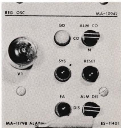
tem can be reset from either terminal. Holding down the loop test key for 15 seconds or longer causes all the relays at both terminals of a system to be returned to normal and removes the "busy" condition from the channel signaling leads at both terminals. This far-end reset feature is especially advantageous when one terminal of a system is unattended.
