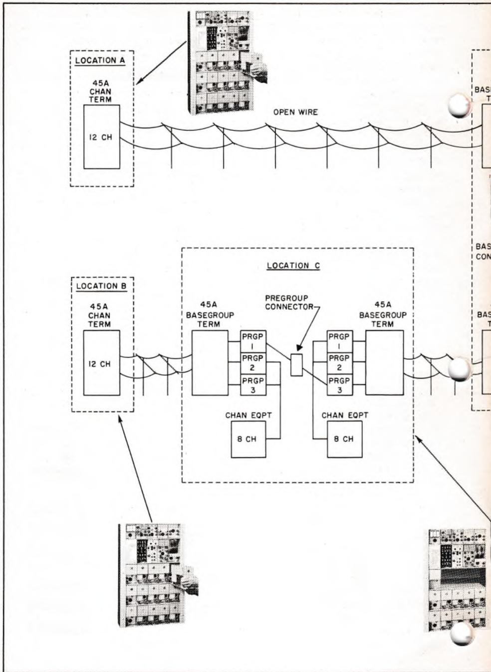
FIGURE 2. Typical 45-class carrier network. A 12-channel basegroup is transmitted from station A to station F over three different transmission media. Basegroup transfers are made at the junctions of the media at stations D and E. Similarly, an 8-channel group (2 pregroups) is transmitted from station C to station F, being
