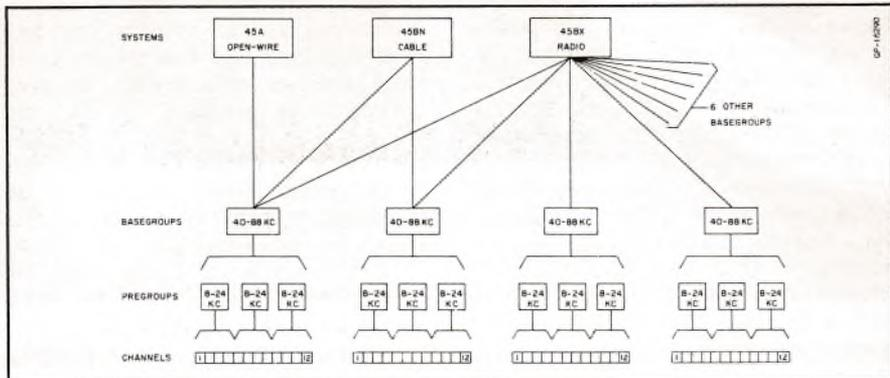
FIGURE 1. Different 45-class carrier systems are developed by combining suitable numbers of pregroups and basegroups and preparing them for transmission over different media.
