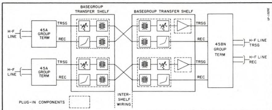
FIGURE 3. Block Diagram of a 45A to 45BN interconnection. Equipment required in addition to the group terminals consists of the amplifiers, pads, filters and transformers making up the transfer shelves.
