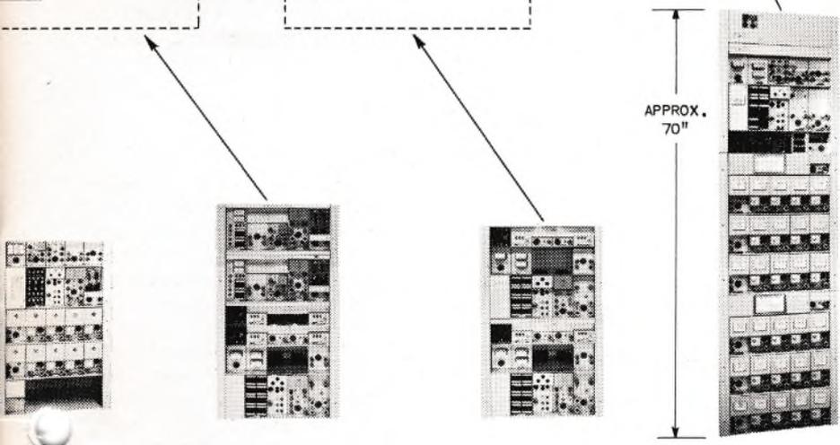
*combined with the 12-channel group at station D. From station B, a 4-channel pregroup is transmitted to station F with a pregroup transfer being made at station C. The 45A system between stations B and C is also used to provide 8-channels directly between these two points. The photographs show the actual equipment (less companders) required at each station.*
