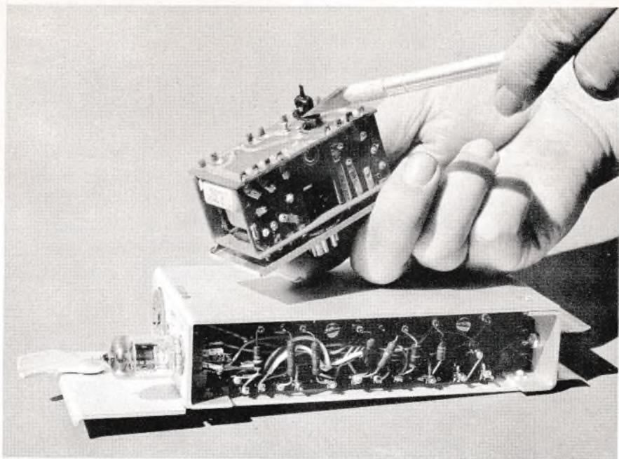
FIGURE 1. *Experimental model of a transistorized, print wired, line amplifier compared to equivalent vacuum tube type. Pointer indicates transistor raised above its normal position.*
