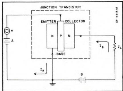
from the emitter to the collector, via the base, to vary with the instantaneous magnitude of  $e$ . As a result the current  $I_B$  and the power delivered to the load impedance  $Z_L$  have the characteristic wave form of  $e$  (which may be very complex in the case of speech) superposed upon them.
