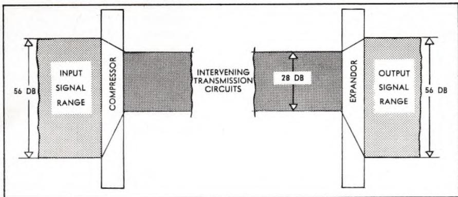
FIGURE 2. Compression and expansion of various signal intensities in a typical compandor for telephone applications. The compressor is at a  $-16$  db level point. The expander is at a  $+7$  db level point.
