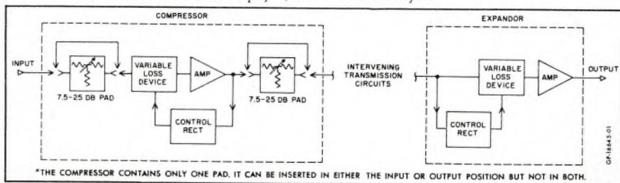
and a -16 dbm input will result in an output of -1.5 dbm, a gain of 14.5 db instead of 2.5 db with respect to the -16 db input. The gains obtained with various magnitudes of input power, without any pad loss, are:
