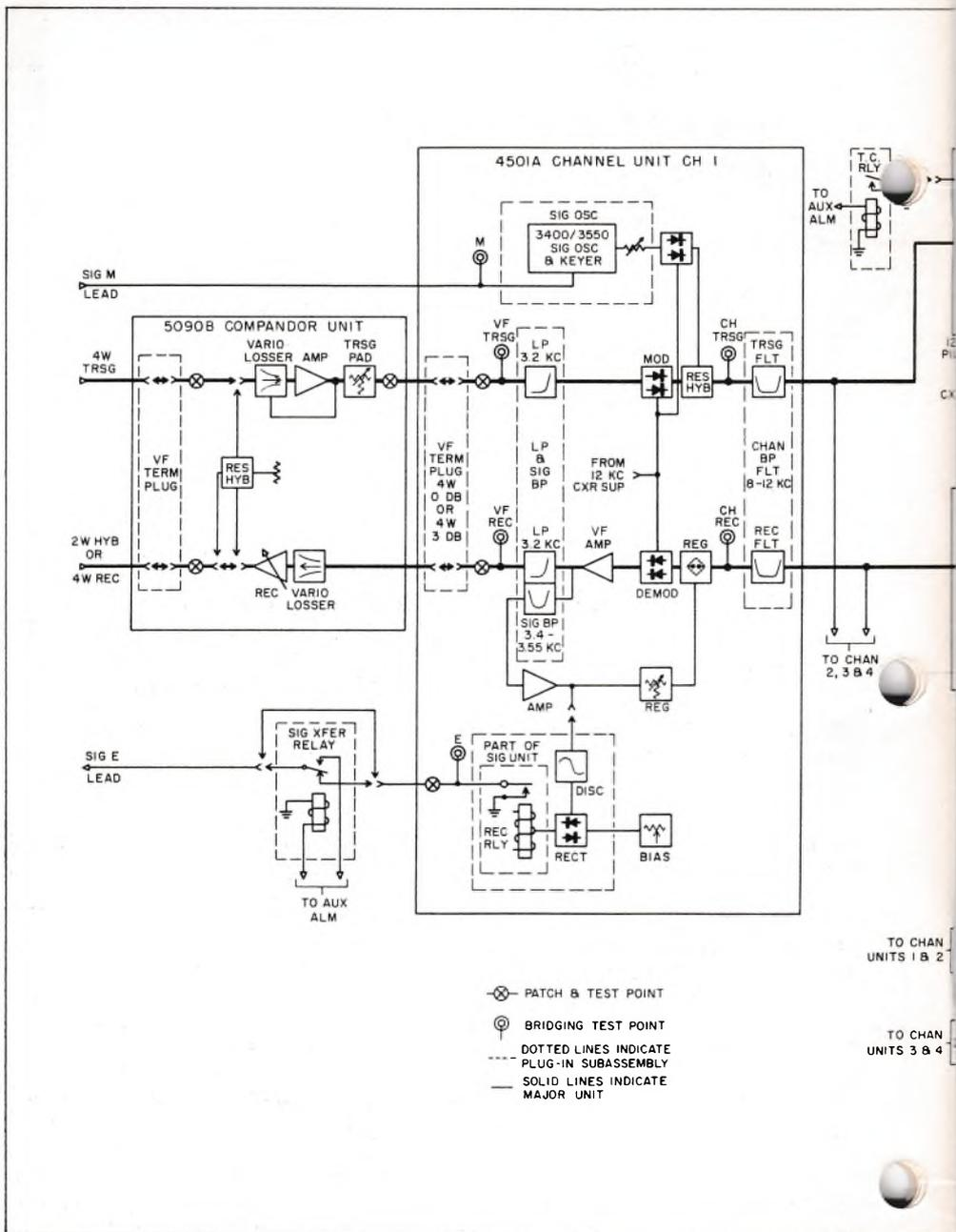
FIG. 5. Block diagram, Type 45CB terminal. in all 45-class carrier systems. Any terminal mission by strapping arrangements in the dire
