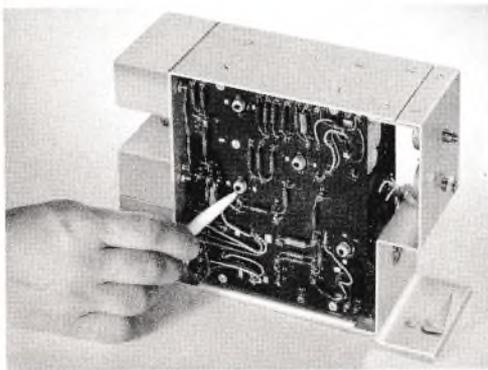
*FIG. 3. The carrier frequency supply unit for a Type 45CB carrier terminal. The pointer indicates one of the six transistors in this unit.*
