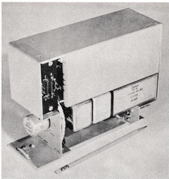
In addition to the channel units and companders, the basic terminal assembly includes group transmitting, group receiving, directional filter, and carrier frequency supply units; also a power distribution and alarm panel. The transmitting, receiving, and carrier frequency supply units make the maximum practical use of transistors and miniaturization techniques. As a result, power drain for these units is reduced to a minimum.
