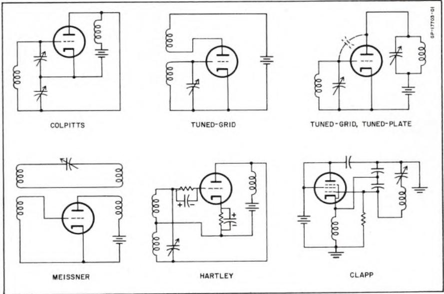
FIG. 3. Six typical LC oscillators. Although the configurations are different, the theory of operation is the same.
