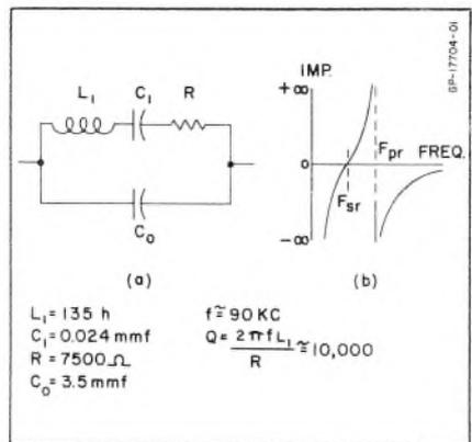
FIG. 4. (a) The equivalent circuit and typical values for a 90-kc crystal. (b) The impedance-frequency characteristic of a crystal.
