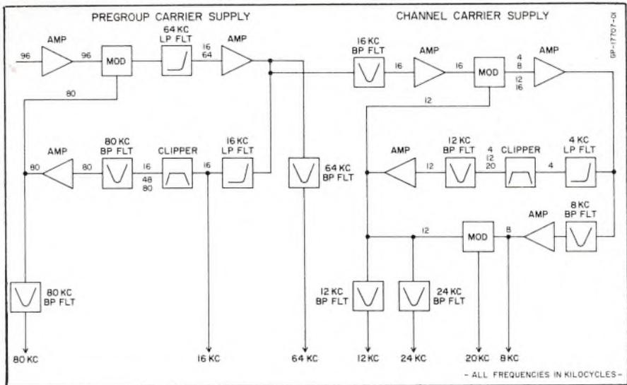
FIG. 9. Block diagram of the pregroup and channel carrier supply units of Lenkurt's 45-class carrier equipment.
