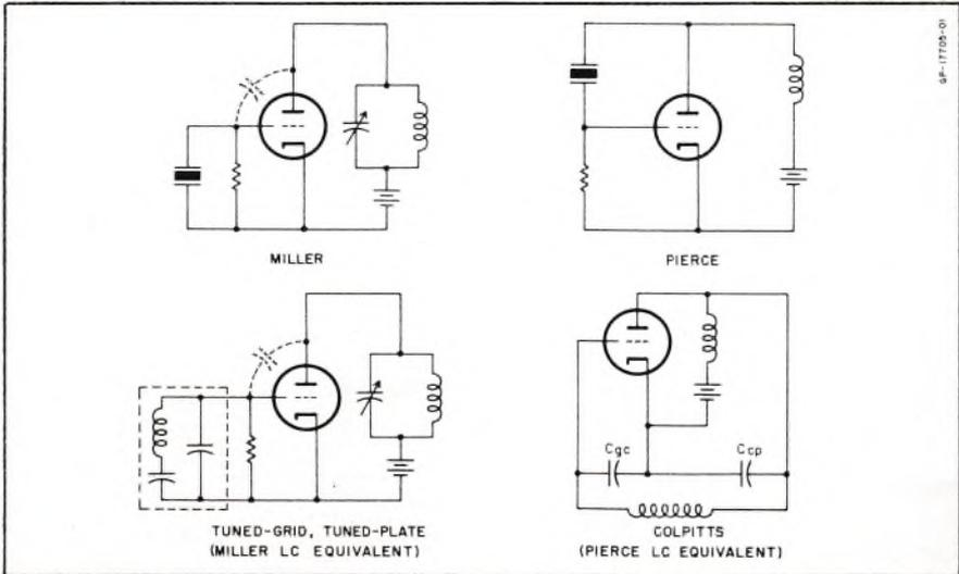
FIG. 5. Two crystal oscillators and their equivalent LC circuits.
