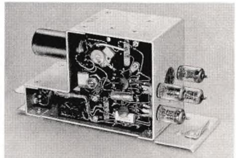
At other than the resonant frequency, the crystal presents a much higher impedance to the feedback loop. When this is the case, most of the feedback voltage appears across the crystal and little is returned to maintain oscillations. The operating frequency of the oscillator is therefore self-compensating and does not deviate appreciably from the desired value of 96 kc.
