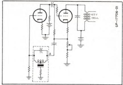
FIG. 6. The circuit of a typical master oscillator for use in a carrier communication system.
