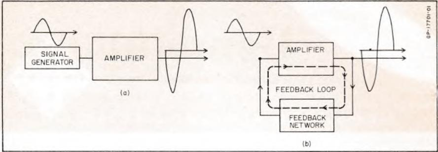
FIG. 1. An amplifier with and without a feedback path. Under certain conditions feedback will cause the system to oscillate.
