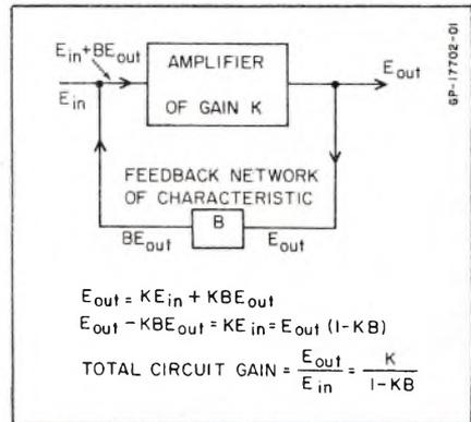
FIG. 2. A feedback amplifier. When  $KB$  equals plus one at an angle of  $0^\circ$  or multiples of  $360^\circ$ , the system becomes oscillatory and  $E_{out}$  can exist without  $E_{in}$ .
