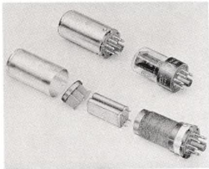
*FIG. 8. An exploded view of a crystal oven, an assembled oven, and a conventional vacuum tube to illustrate relative size. The oven contains two crystals—one for each of the two oscillator circuits in the master oscillator. The oven is electrically heated and thermostatically controlled.*
