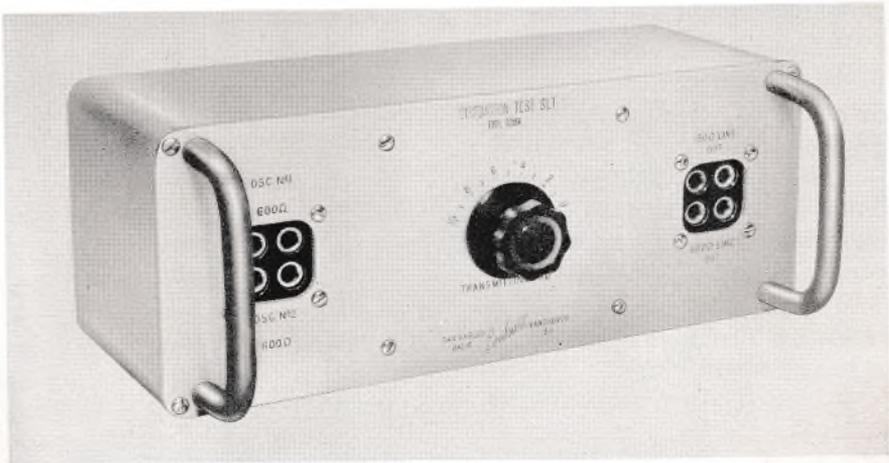
*FIG. 1. Type 7281A Test Set used in testing Lenkurt Type 72 radio equipment. Transmitting pad controls level of reference signal.*
