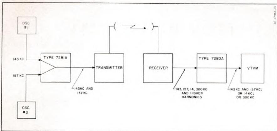
FIG. 2. Block diagram of typical test arrangement. Signal frequencies shown are those used in testing Lenkurt Type 72B radio equipment.
