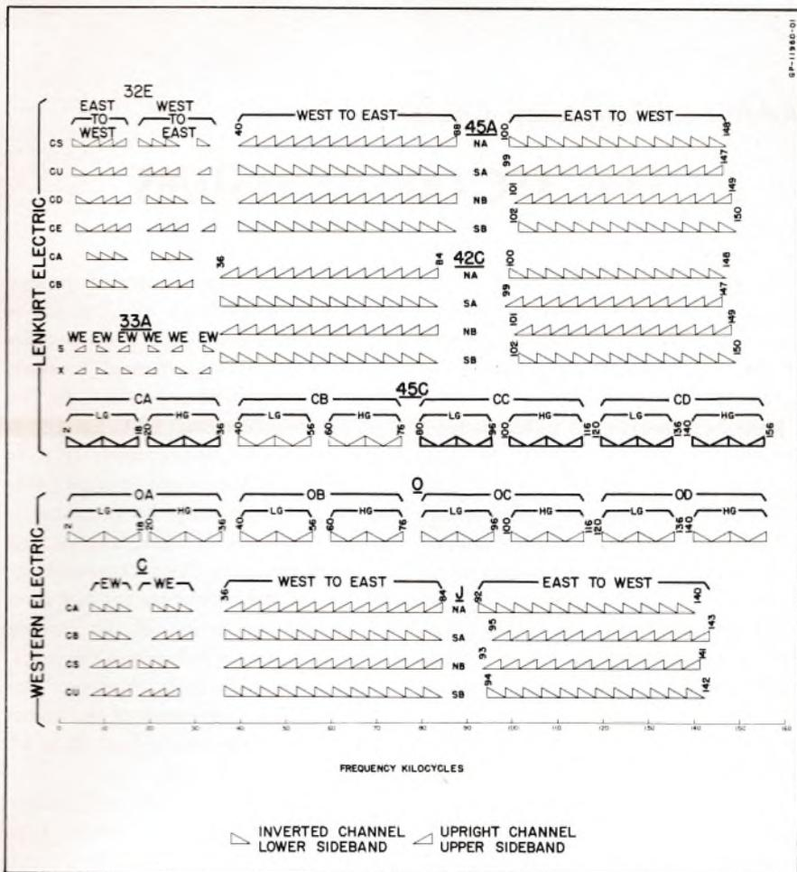
FIG. 1. Frequency allocations of open-wire carrier systems. Heavy lines indicate new Type 45C allocations.
