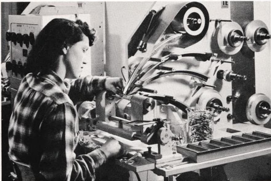
FIG. 4. Automatic machine used for winding polystyrene capacitors at Lenkurt.
