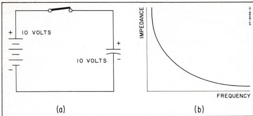
FIG. 2. (a) A circuit in which electric charge has built up in a capacitor opposing the flow of current from the d-c source. When steady state has been reached, no current can flow. (b) The impedance-frequency characteristic of a capacitor.
