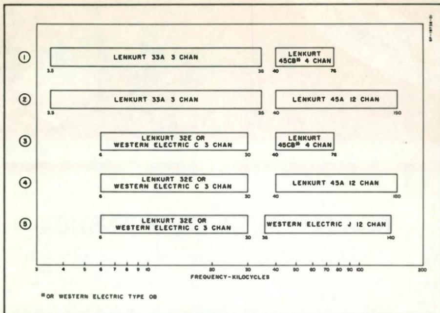
FIG. 1. Five combinations of open-wire carrier systems which co-ordinate on the same pair. All combinations shown may be superposed on physical voice-frequency circuits.
