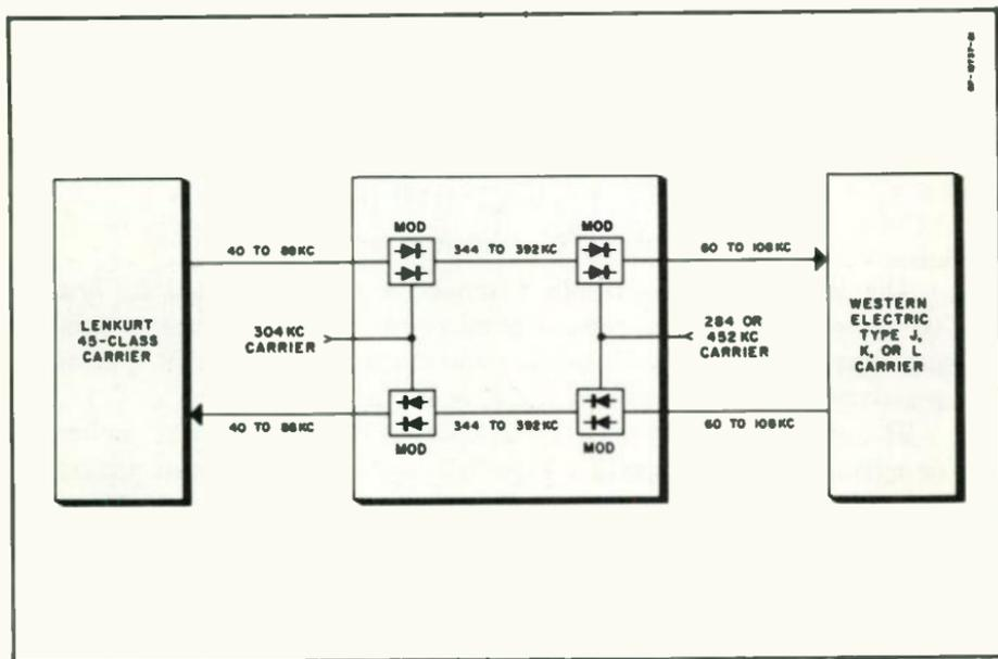
FIG. 2. Group modulation is used in the Lenkurt Basegroup Transfer Converter Unit to interconnect 45-class carrier to Western Electric J, K, or L systems at carrier frequencies.
