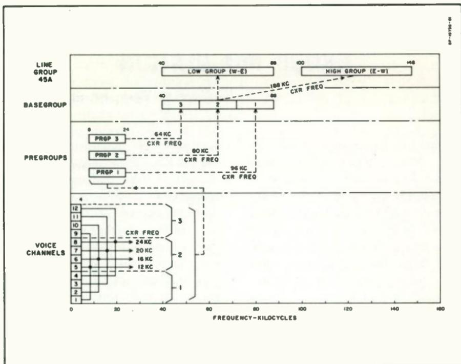
FIG. 1. Modulation plan for Lenkurt Type 45A carrier. Except for the high-frequency line group, this plan also applies to Type 45BN cable carrier and Type 45BX radio channelizing equipment.
