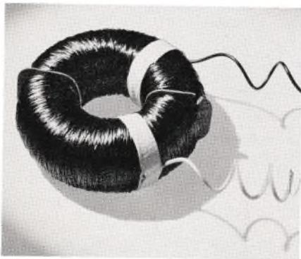
FIG. 1. Typical toroidal coil.
