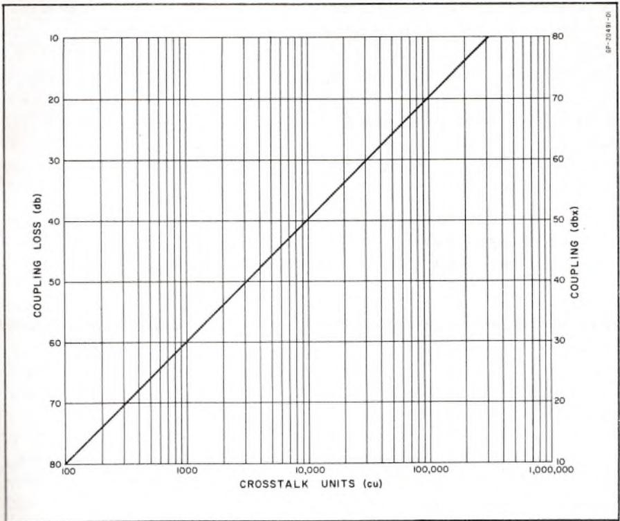
FIG. 1. Nomograph showing the relationship between *cu*, *db* and *dbx*.
