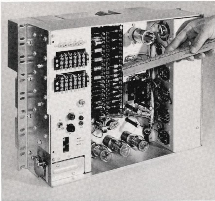
*FIG. 2. Power supply for the transmitting and receiving klystrons. The only active components in this supply are the three voltage regulator tubes shown near the bottom of the unit.*
