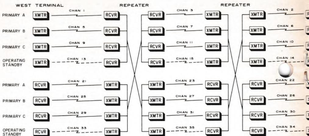
FIG. 6. Frequency assignment plan for a radio system, each radio-frequency channel
