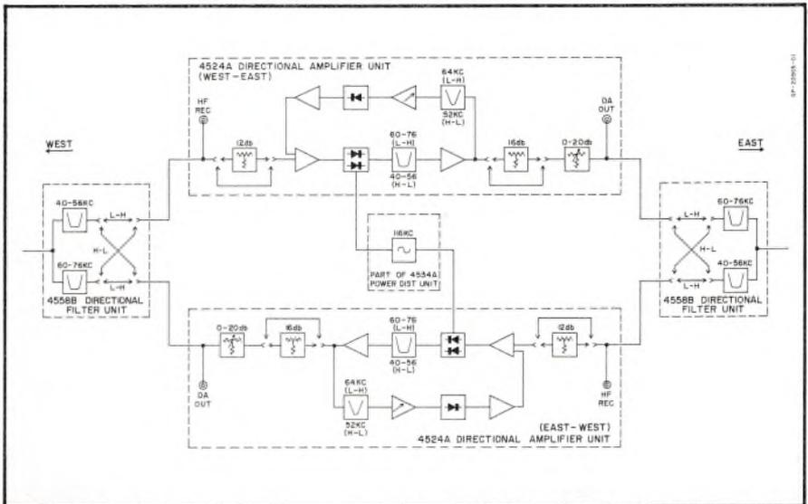
FIG. 1. Block schematic diagram of the 45C Repeater. The frequencies shown are for the CB allocation.
