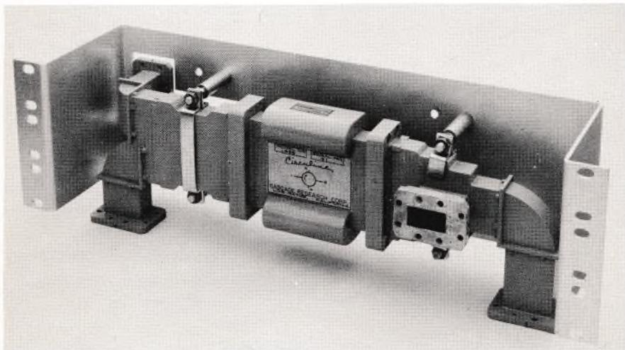
FIG. 3. The waveguide ferrite circulator designed specifically for the Type 74A Radio System. This device permits three microwave terminals to be connected to the same antenna without mutual interference.
