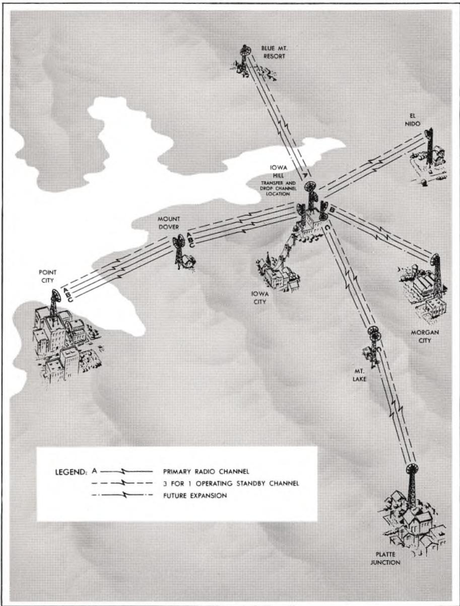
FIG. 7. A possible network of Type 74A microwave equipment using one standby channel for three operating channels.
