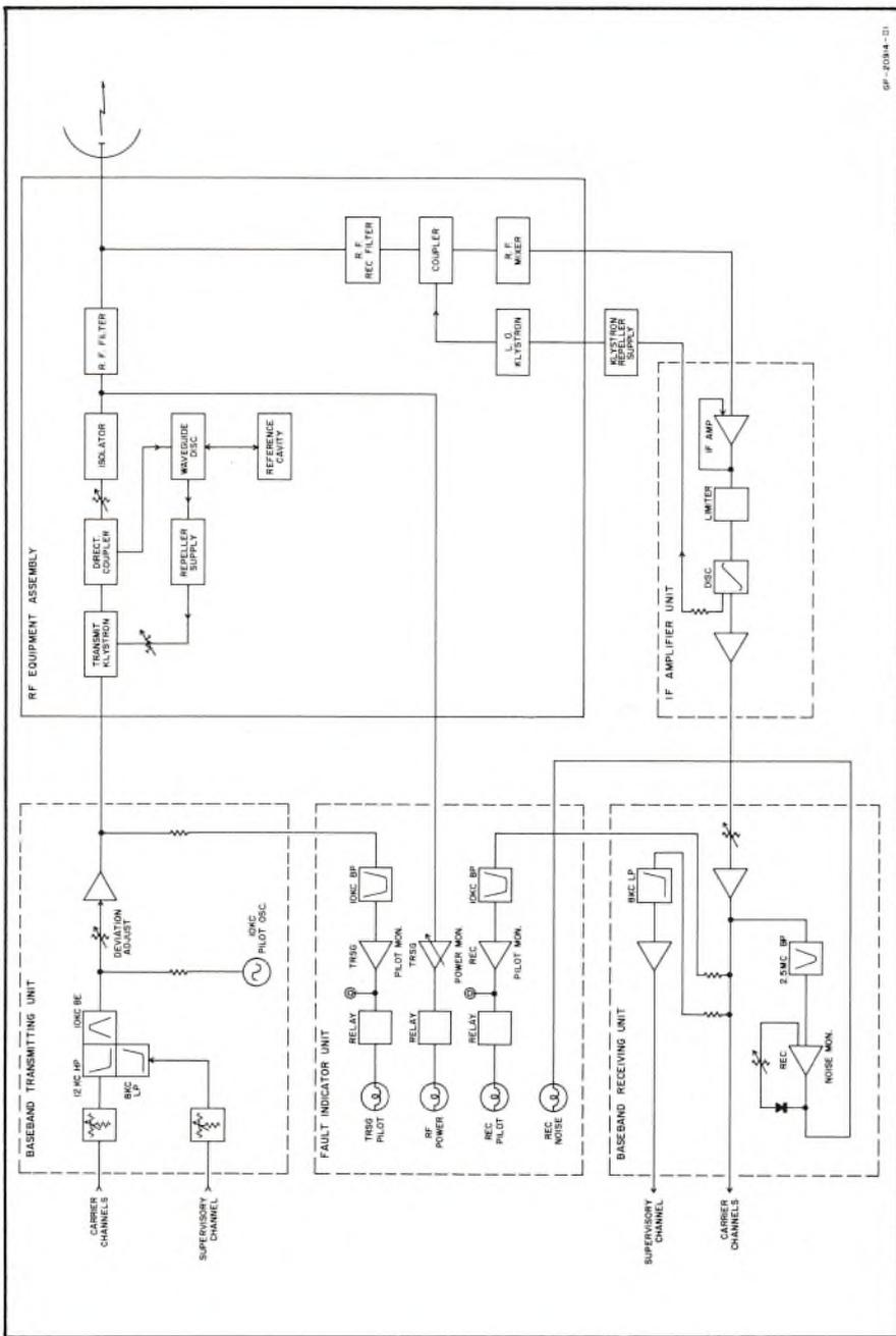
FIG. 5. Simplified block diagram of a Microtel terminal. When standby equipment is furnished, a terminal also includes a combining and transfer unit and a ferrite circulator.
