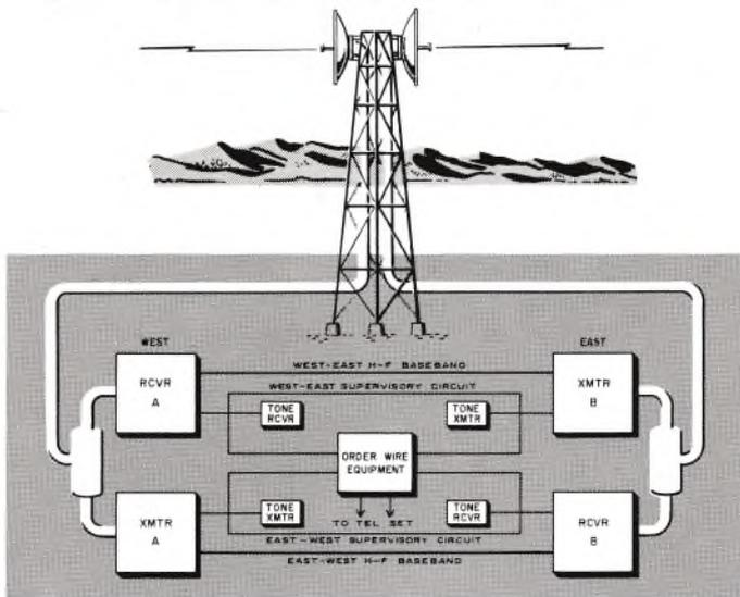
FIG. 4. Block diagram of a typical Microtel repeater station.
