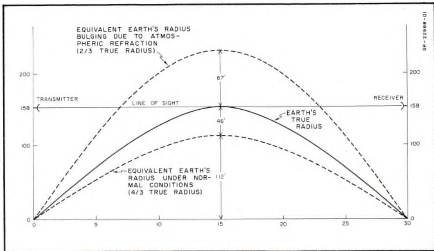
Fig. 5. In this example normal atmospheric refraction permits a signal clearance of 46 ft. above the earth. This is represented by an equivalent flattening of the earth's radius to  $4/3$  true radius. When atmospheric density increases with height the earth's surface appears to bulge upward. Here a bulge of 67 ft. above line-of-sight gives an equivalent earth's radius of  $2/3$  true radius.
