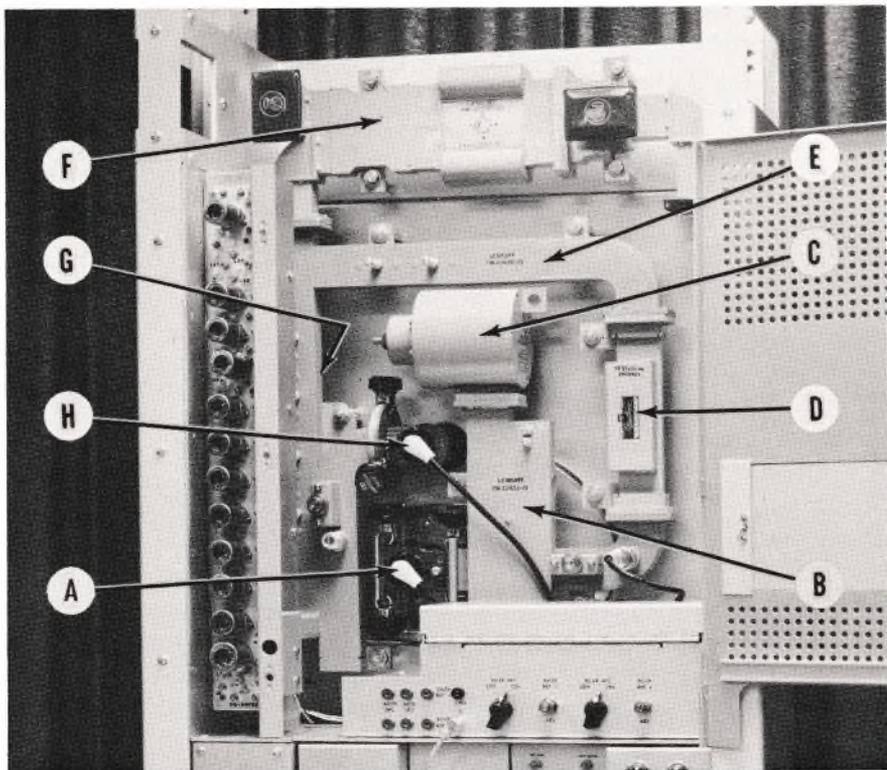
*Fig. 2. Type 74A transmitter-receiver with waveguide assembly exposed. The principal microwave components shown are: (A) transmitting klystron; (B) waveguide discriminator; (C) reference cavity for controlling transmitter frequency; (D) isolator; (E) waveguide run to circulator panel; (F) circulator panel; (G) waveguide run to r-f mixer; and (H) local oscillator klystron.*
