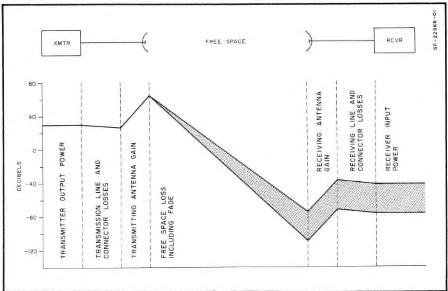
Fig. 3. Gains and losses in a typical radio section. The shaded area indicates the range of losses expected from fading during 99.9% of the time.
