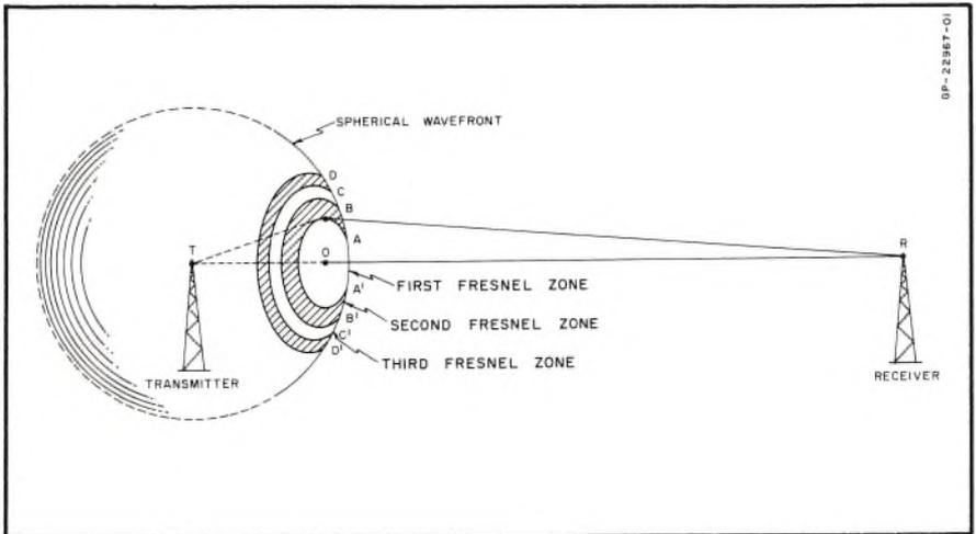
Fig. 4. Fresnel zones of a transmitted signal's wavefront at distance OR from a receiver. The difference in path length to receiver from edge of one zone and edge of adjacent zone is one-half wavelength. Odd-numbered zones reinforce the signal and even-numbered zones cancel it.
