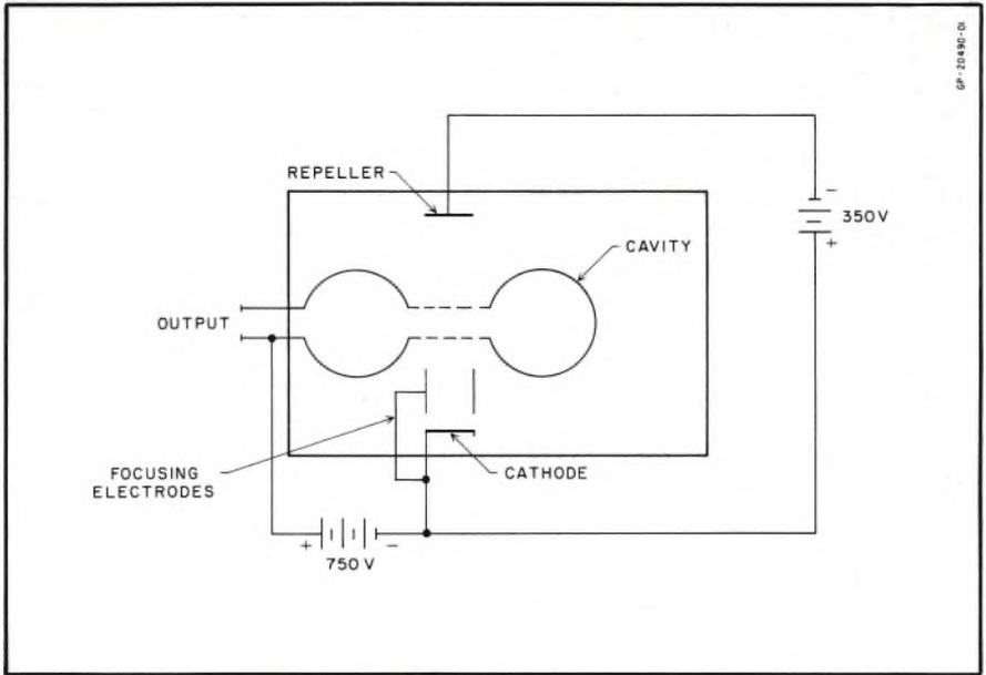
Fig. 1. Diagram of a reflex klystron. Electrons flow from the cathode across the cavity gap toward the repeller. The repeller returns the electrons in bunches to the cavity gap. These electron bunches induce voltages across the cavity at its resonant frequency and maintain a condition of oscillation.
