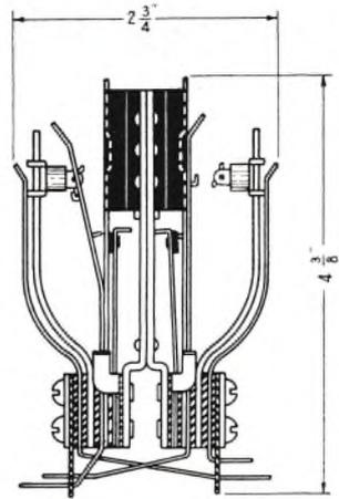
Fig. 4. Cross-section of the Type 675 protector. One heat coil is shown operated.
