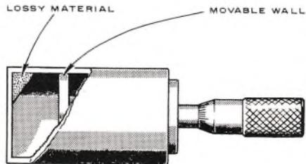
*Fig. 2. A typical resonant cavity.*
