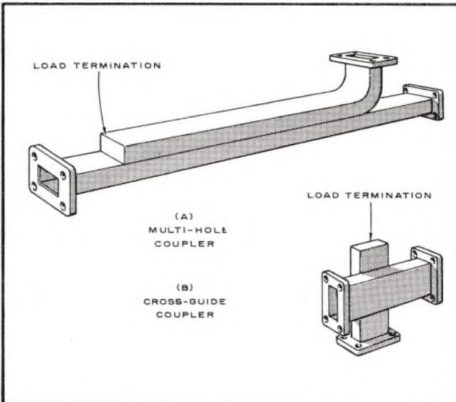
Fig. 5. Directional Couplers: At top, a typical example of a multi-hole coupler; at bottom, a typical example of a cross-guide coupler.
