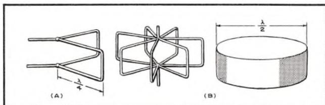
Fig. 3. Development of a Resonant Cavity.
