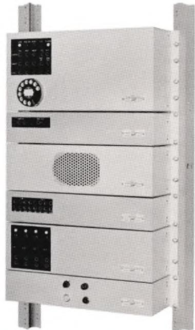
Fig. 3. The above is a photograph of a complete L2 Control Terminal used in the Lenkurt Mobiltel-Manual system.
