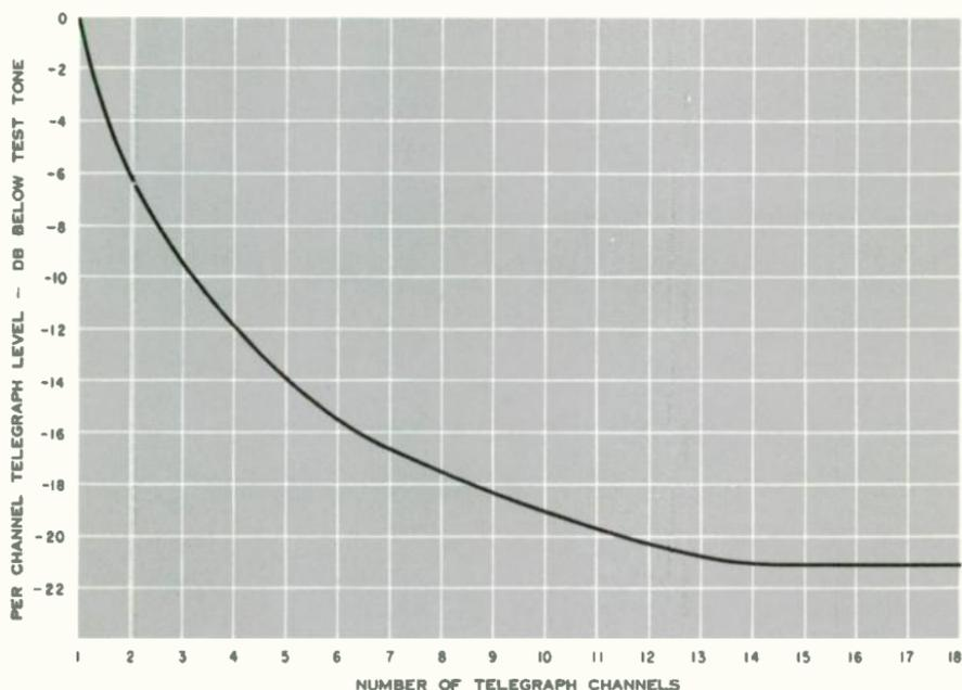
Figure 1. Theoretical maximum per-channel transmission levels for various numbers of telegraph channels transmitted over a carrier voice channel.
