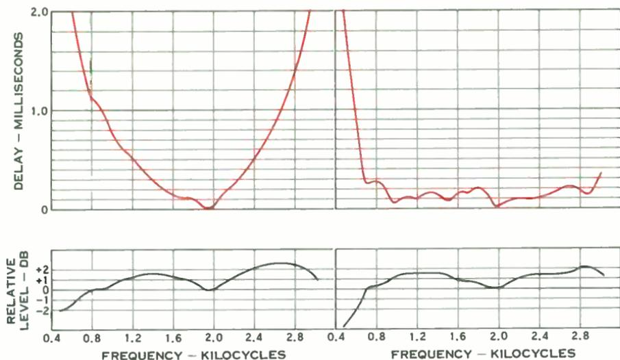
*Figure 3. Amplitude and delay characteristics of a cable carrier channel before and after equalizing delay. In this 450-mile path, signal was translated down to voice frequencies four times.*
