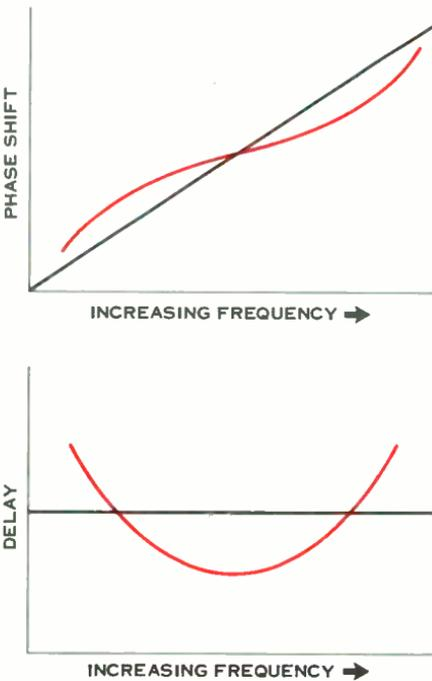
Figure 2. Comparison of the effects of linear and non-linear phase shift on envelope delay in a communications link. Linear phase shift produces uniform delay at all frequencies. Non-linear phase shift causes delay to vary with frequency.
