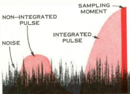
Figure 11. Bit integration builds up pulse amplitude. Noise fails to build up because of statistical cancellation of individual noise pulses.
