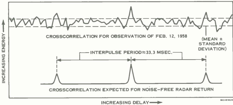
Figure 10. Use of pulse integration and statistical correlation techniques made possible radar contact with planet Venus and Sun. Similar technique can be used to improve high speed data transmission, particularly with longer pulses.
