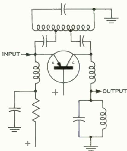
Figure 2. One variation of Vodicka converter which has provided useful gain at frequencies several times the transistor alpha cutoff frequency.
