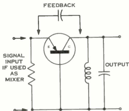
Figure 1. Basic grounded-base oscillator, showing possible feedback path for high frequency oscillation.
