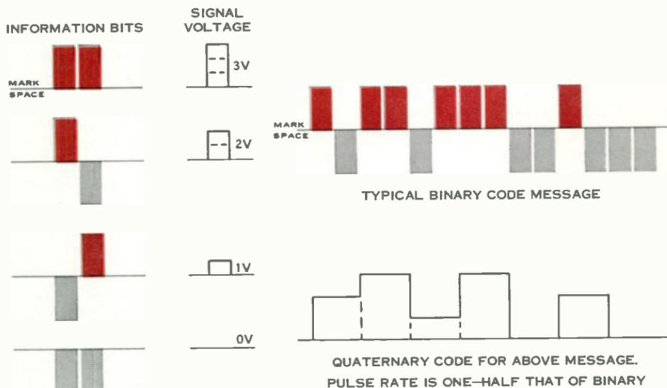
Figure 8. Quaternary (four-level) code adapts binary information for transmission by four tone system shown in Figure 7. Each pair of information bits is represented by one tone or level. System requires transmission system with good tolerance to noise and level changes.
