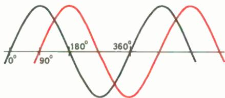
Figure 3. Phase Modulation systems are based on shifting the phase of a carrier from the normal or "zero" phase. Red waveform is shown advanced  $90^\circ$  in phase.
