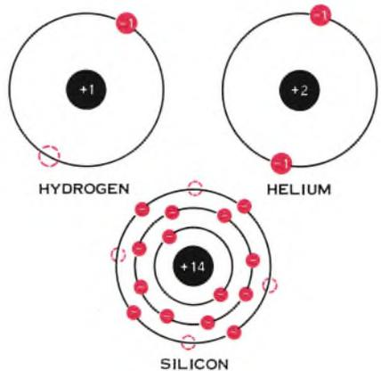
Figure 6. Hydrogen atom with one electron has incomplete outer ring. Helium atom has filled outer ring and is completely inert. Silicon atom has four of the eight possible electrons required to complete its outer ring. Relatively little energy is required to free electrons.
