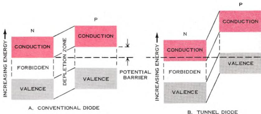
Figure 12. Very heavy doping of  $n$  and  $p$  semiconductors shift their respective energy levels. Applied forward bias tends to reduce difference between two. When valence band of  $p$  material is directly opposite conduction level of  $n$  material, current carriers may "tunnel" through potential barrier at speed of light. Increased forward bias shifts  $n$  valence band opposite  $p$  forbidden zone, restoring normal diode behavior.
