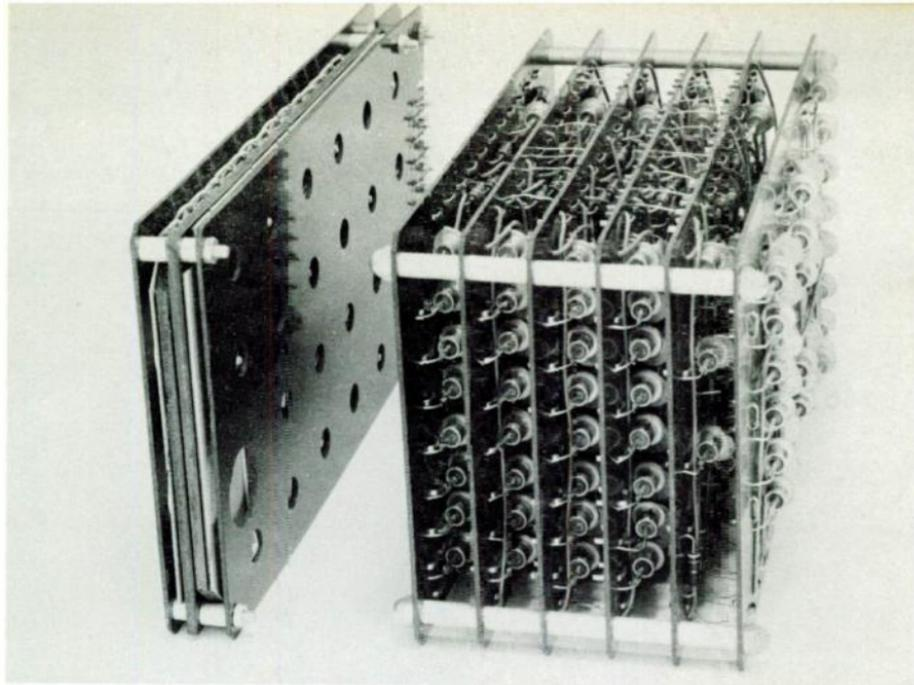
*Figure 6. Modern communications systems are becoming more complex, requiring careful design to reduce space requirements. Prototype logic circuit on right employs 96 semiconductor diodes. Production version on left uses 332 diodes, yet requires only small fraction of the space of the earlier unit.*
