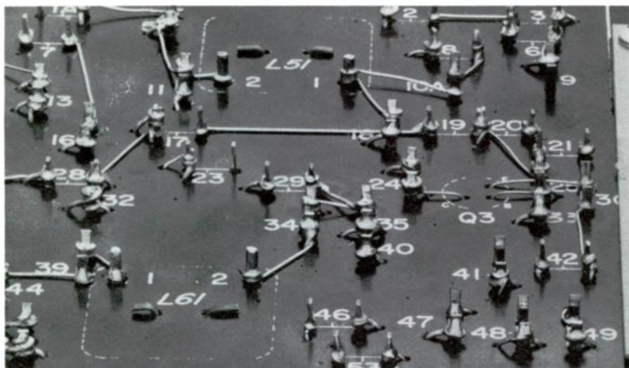
*Figure 5. Back view of channel unit. Interconnections are automatically machine-wired, thus providing uniformity and economy of printed wiring. All wires and component leads are machine-wrapped around staple-ends at optimum tension for good mechanical and electrical connection. Units may be performance-tested before soldering. Unlike printed wiring, components are easily replaced without risk of damaging board or interconnections.*
