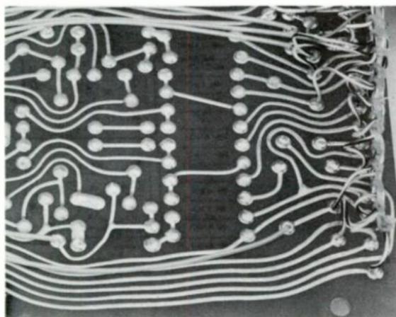
*Figure 2. Typical high-quality printed circuit. Board material is Fibreglas and epoxy resin to minimize effect of moisture absorption on circuit performance. Printed circuits are uniform and economical, but require very tight control of many process steps to maintain high reliability.*
