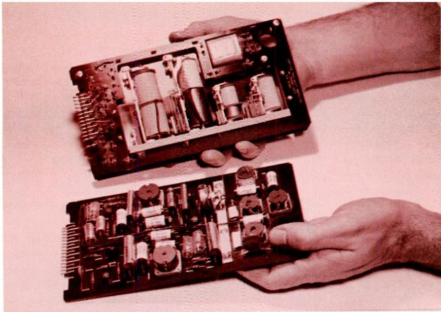
*Figure 4. The new Type 81A Exchange Carrier uses "stitched wiring" to improve solder joint reliability and reduce the number of hand operations. Automatically-inserted bronze staples serve as attachment points for components and interconnecting wires. Components may be inserted by machine or hand. Units shown are a channel unit and a signaling unit. Although far smaller than old channel-signaling units, new design approach permits far more elaborate signaling functions.*
