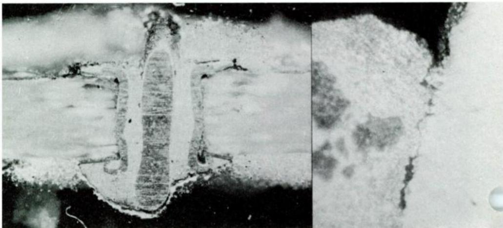
*Figure 3. Magnified cross section of printed wiring solder joints, showing cracks between solder and component lead. This type of failure cannot be detected visually, but results in high resistance joint or open circuit.*
