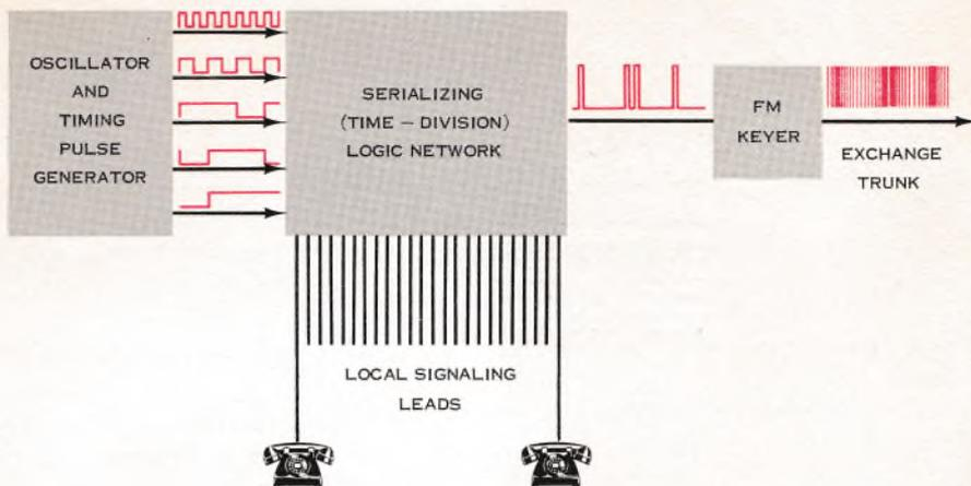
Figure 6. Type 81A Exchange Carrier system employs time-division for signaling. Each local line is assigned its own "time slot." Local signals from all 24 telephones are carried in special binary FM signaling channel.
