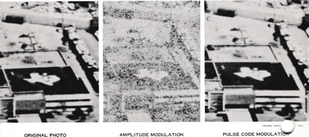
*Figure 3. Comparison of transmission by amplitude modulation and pulse code modulation. Both transmissions were made under identical conditions of noise and transmitting power (4 db signal-to-noise ratio). Improved transmission by PCM is obtained at expense of bandwidth.*
