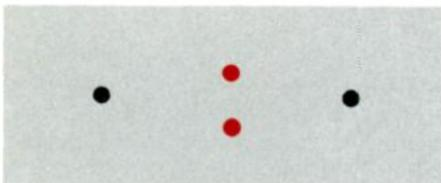
*Figure 1. Two pairs arranged so that both conductors of each pair are equidistant from disturbing conductors. Such arrangements are impractical for many pairs.*
