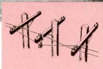
*Figure 2. Typical open wire lines showing drop-brackets for transposing pairs. The insert shows the manner in which the individual conductors are transposed, using the brackets.*
