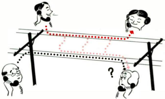
mission frequencies are used for each direction of transmission. Even though signal energy is coupled from one pair to another, the crosstalk is in the wrong portion of the frequency spectrum to pass the carrier channel filters. This "frequency staggering" not only reduces the effective crosstalk coupling between circuits, but it changes the nature of whatever crosstalk does get through, to a form that is much less annoying than the crosstalk between non-staggered channels.
