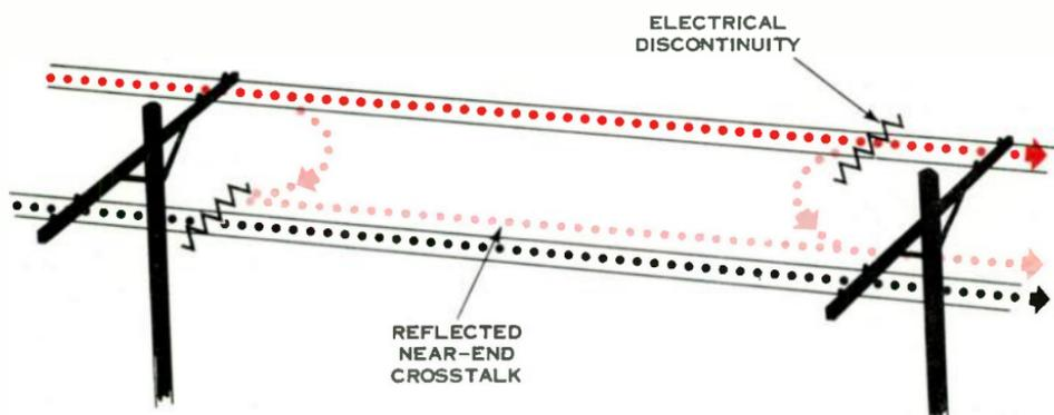
Figure 6. Two types of far-end crosstalk resulting from near-end coupling and reflection from an electrical discontinuity, such as an impedance mismatch.
