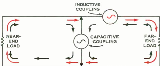
Figure 5. Transverse far-end crosstalk reaches far end without reversing direction in process, is due mostly to inductive coupling.
