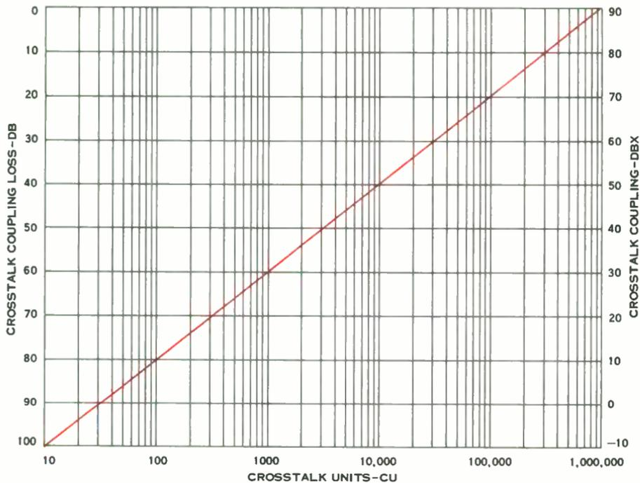
**Figure 9.** Relationship between crosstalk coupling loss in db, crosstalk units, and crosstalk coupling in dbx. Crosstalk units are little-used now, having given way to coupling loss and dbx coupling for measurements of circuit characteristics, and to crosstalk index for subjective performance rating.
