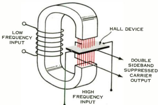
Figure 5. One possible design for Hall-effect ammeter that would operate without breaking the circuit to be measured. C-yoke collects field around conductor, concentrates it through Hall device.
