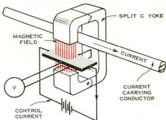
telemetering sensor for variables such as air pressure or mechanical strain, which may change at very slow rates.
