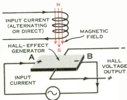
*Figure 2. Modern Hall-effect device produces output voltage proportional to the product of magnetic field strength and input current (A and B leads).*
