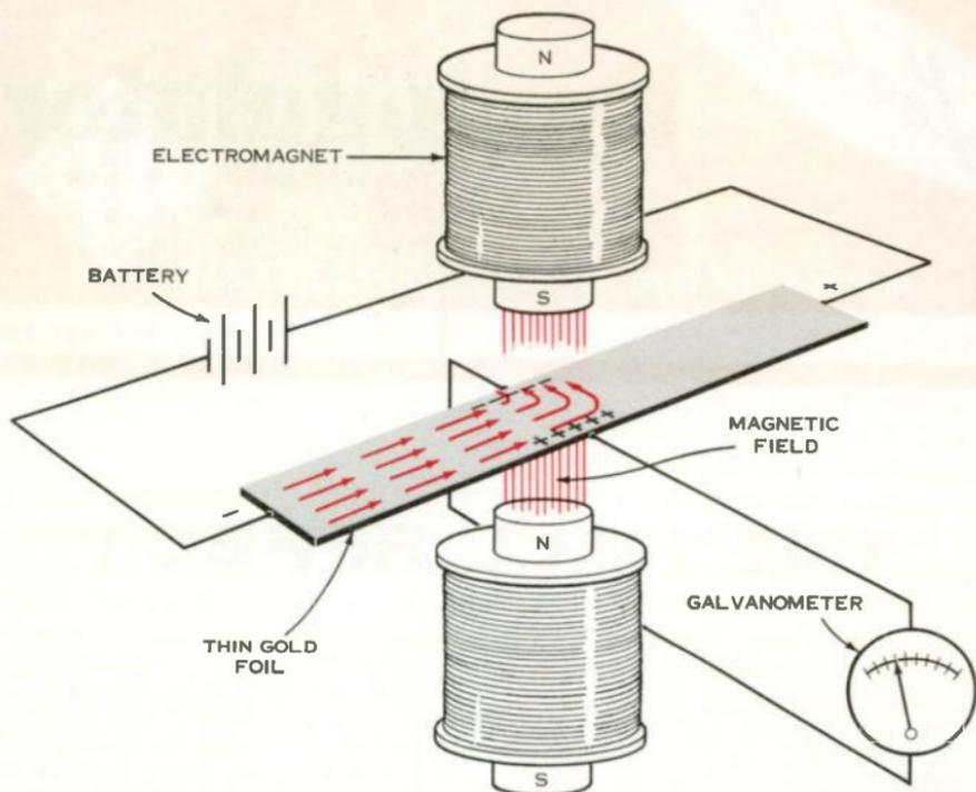
*Figure 1. Original Hall experiment measured deflection of electrons in conductor by magnetic field. This important experiment contributed to basic knowledge by the nature of electrical conduction, and paved the way for future semiconductor developments.*
