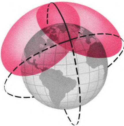
*Figure 7. Time during which communication is possible between stations will vary with location of orbit relative to stations. This will change with each pass. Tinted area shows coverage of each station and where they overlap. Communication between the two is possible only in overlap area.*
