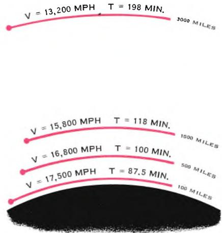
Figure 4. Gravitational force decreases with increased altitude, requiring lower velocity to maintain orbit. Some typical velocities and periods for earth satellites of different altitudes are shown. Although less velocity is required at high altitudes, much more energy must be expended in reaching it.
