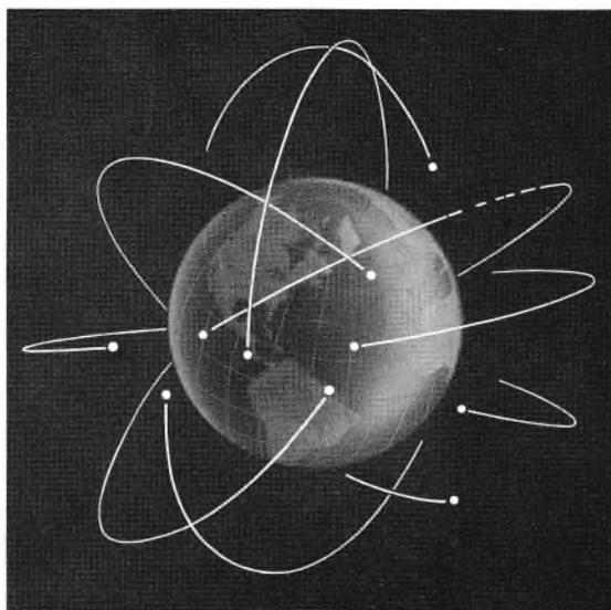
*Figure 8. Fifty or more low- or medium-altitude satellites in random orbits will be required to assure continuous communication between any two stations. Number must be even larger to allow communication with other stations. Although numerous, these satellites can be relatively cheap. Terminal costs are high, due to finding and tracking difficulties.*
