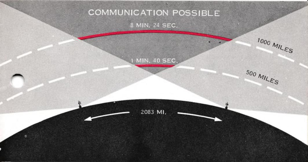
*Figure 6. A major difficulty of low-altitude satellites is their rapid transit time and limited coverage. For communication, satellite must be within view of two stations simultaneously. Experimental low-level satellite soon to be launched will be placed in highly elliptical orbit designed to increase its time over northern hemisphere at expense of southern hemisphere.*
