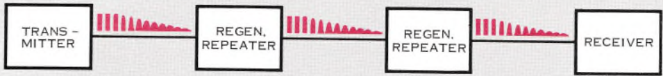
Figure 4. Pulses undergo constant attenuation and degradation in cable. Most crucial function in system is the accurate retiming and regeneration of distorted pulses.
